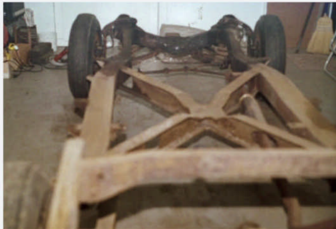
An early image of the Custom Royal Lancer's X-braced frame after the engine and transmission had been removed. The suspension and exhaust systems still remain. Little is left of the original factory chassis paint, replaced by light surface rust from moisture.
