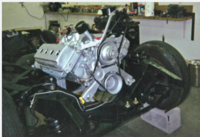
The 270-cu.in. Hemi V-8 has been completely reassembled with new pistons, a complete set of valves and a new camshaft, and then carefully refinished in correct silver and reunited with its rebuilt PowerFlite transmission before being bolted back in place.
