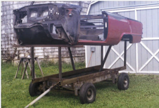
After the Dodge was fully disassembled, the convertible body was braced from within to prevent twisting, and then placed on a homemade dolly. The height may imply adverse working conditions; however, it did assist with inspecting the underside.
