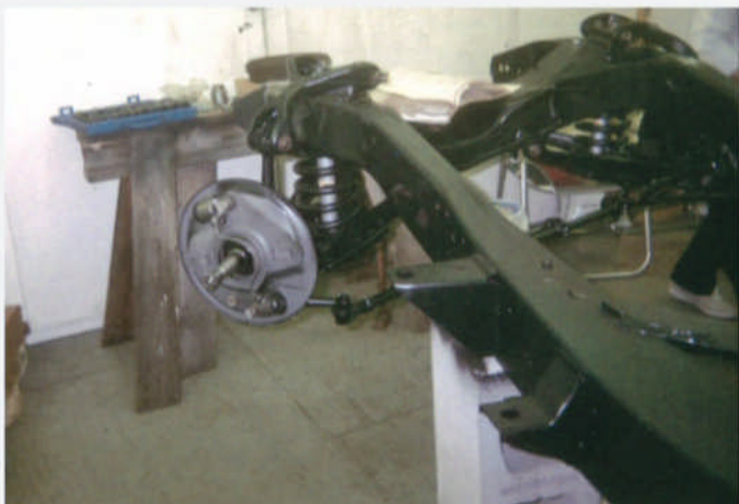
After the chassis and suspension were media blasted, sealed in primer and then painted in chassis black, reassembly could begin. Here, much of that process has been accomplished, including new brake parts; note Dodge's use of dual front brake cylinders.
