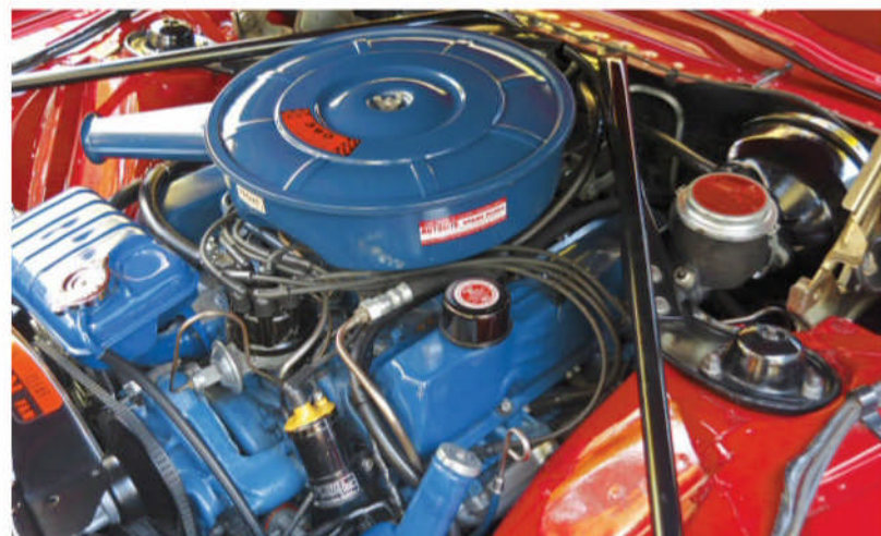
Ford’s muscular 390-cu.in. V-8 made a solid 315 horsepower and 427-lb.ft. of torque in Thunderbird Special guise as shown here.
