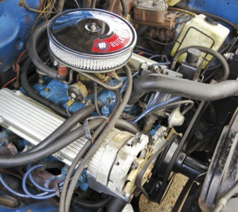
Fitting a chrome air cleaner was a popular period “upgrade” to the V-6, as owners hunted for every ounce of extra horsepower. With its two-barrel Holley carb, it made just 105 horsepower.
