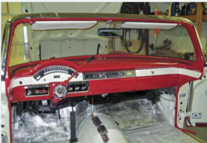
Final reassembly is progressing in the passenger compartment with the installation of the instrument panel and associated trim. Sun visors are in place, and both doors have already been hung and balanced. Also visible is the restored forward-hinged hood.
