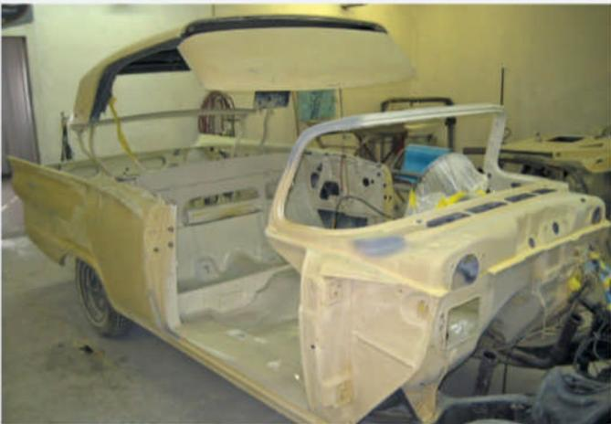
At this stage, after small repairs had been made to the quarter panels, the main body shell was sprayed in a layer of self-etching primer and Rage Gold body filler. A keen eye will note that the interior has already been repainted in Colonial White.
