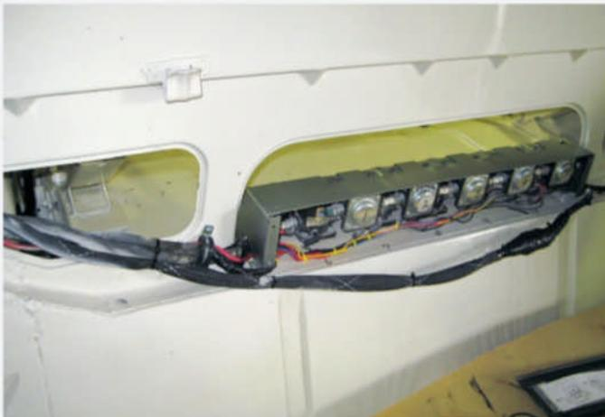
Located behind the rear seat is the primary bank of 12-volt starter relays required to manipulate the folding hardtop. The process of restoring the wiring was tedious, as each unit had to be properly linked to circuit breakers and limit switches.
