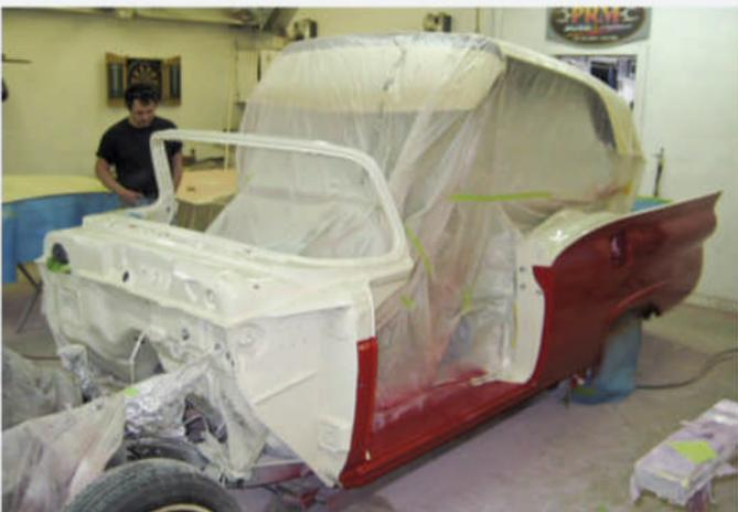
Three coats of PPG Flame Red urethane have been applied to the Skyliner's flanks, completing the bulk of the body's restoration; four layers of clearcoat would soon follow. It was at this point when the restoration took on a new direction and meaning.
