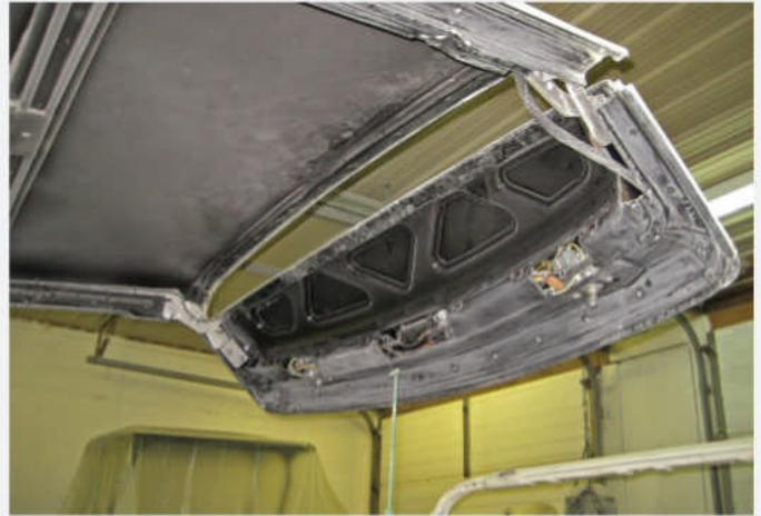
Look closely at the forward lip of the folding roof, and you'll note the electrical system is still in place late in the disassembly phase. These components were left in order to keep the roof functioning, which would help later on during the primer and paint stages.
