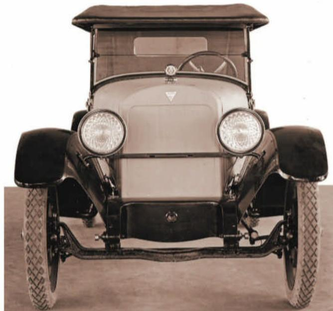
This 1921 experimental car, which looks to be a seven-passenger touring model, demonstrates some of the methods used in styling early Hudsons. From the side, it appears to be a fully-functioning automobile, but a look at the front reveals the radiator is a fake, used to gauge its appearance on the car. The fake radiator would have been made of either wood or plaster.
