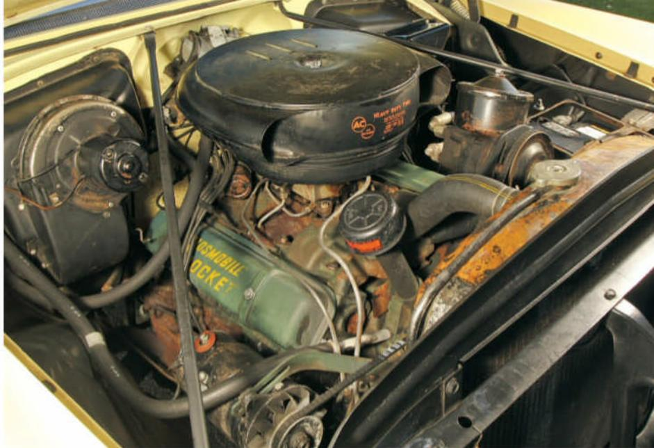
The 202-hp, 324-cu.in. four-barrel engine hasn't required significant work, just maintenance, since the day it was installed on the Lansing assembly line.
