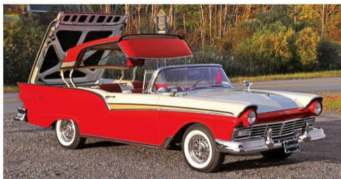
from the household wall switch, someone had redone most of it with cheap yellow wiring, making it a nightmare to trace. The top requires a series of relays, circuit breakers and limit switches, and those limit switches are the key to making the system operate in perfect order and timing. It was a very time consuming repair."
