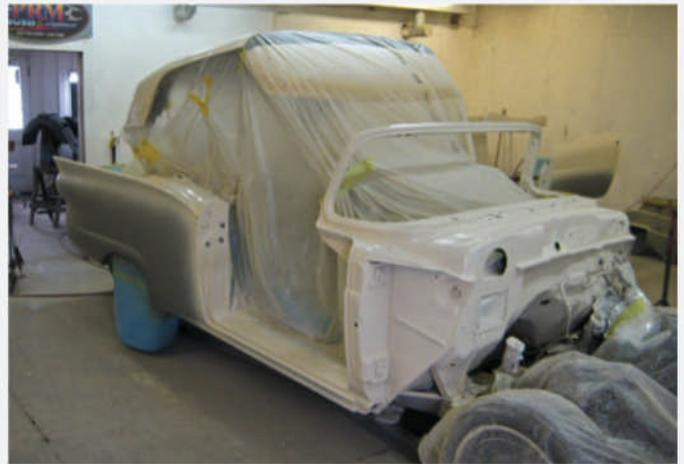
With the chassis and interior masked, the body has already received a final coat of epoxy primer, visible on the quarter panel. The rest of the body has been given three coats of Colonial White PPG urethane to complete one half of the two-tone finish.
