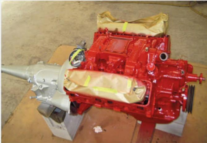
A previous owner's refurbishment effort had the 312-cu.in. V-8 engine and Ford-O-Matic two-speed automatic transmission already rebuilt. After careful inspection, all that was required for this restoration was a simple cleaning and proper repaint.
