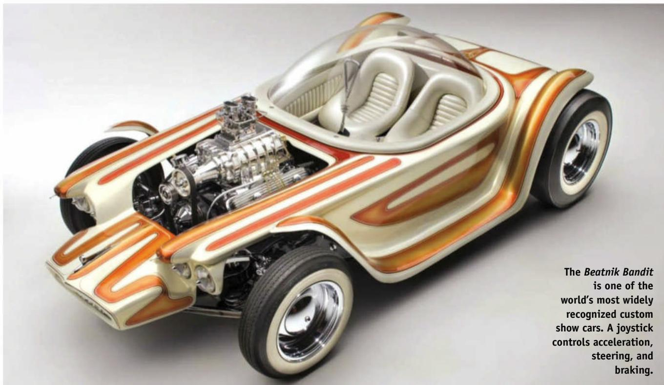
**The *Beatnik Bandit* is one of the world's most widely recognized custom show cars. A joystick controls acceleration, steering, and braking.**
