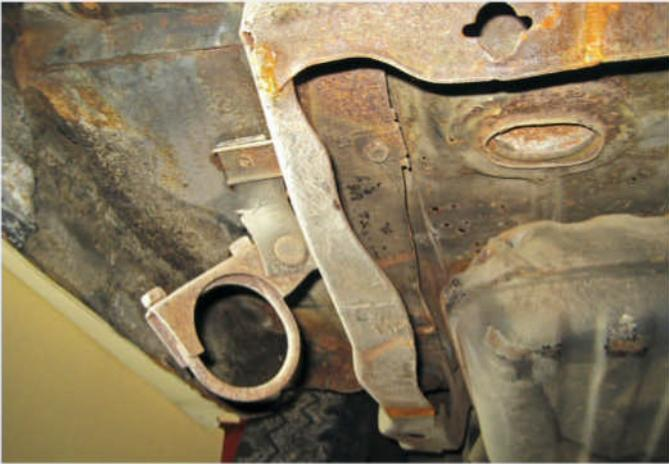
Few photos of the Skyliner's restoration were taken because of the original intention to merely make a good "driver"; however, this one illustrates the overall condition of the chassis in the early stages of disassembly. Only a few patch panels were found and no rot.
