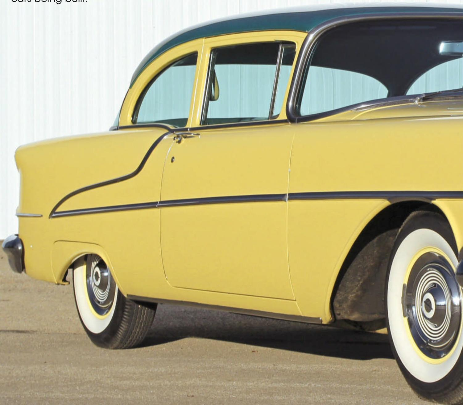
Oldsmobile offered the 88 and Super 88 series on a 122-inch wheelbase and the Ninety-Eight on a 126-inch wheelbase. The entry-level 88 line featured a four-door sedan, two-door sedan or two-door Holiday coupe (hardtop). A 324-cu.in. two-barrel engine and three-speed manual transmission were standard with the four-barrel engine optional.
