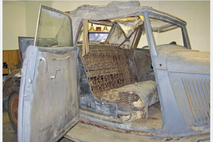
The Ford was immediately evaluated for obvious needs, including a new seat and—given the layer of mold and primer throughout—new door panels. Note the copious rust exposed along the top of the outer rocker panel, hinting at what was yet to be exposed.
