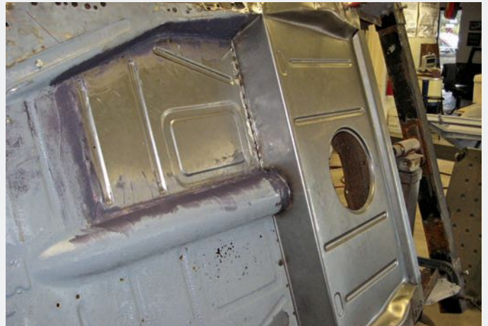
Using a rotisserie, the body was rotated, exposing the underside and allowing the floorpan patch panels to be butt-welded into place. Tack welds initially secured the panels before the entire seam was welded in small sections to avoid warping.
