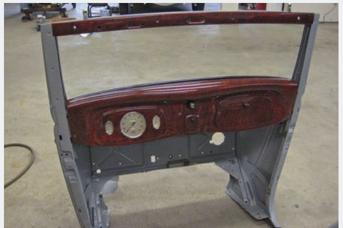
Earlier, the dash panel was restored by means of a woodgrain kit that was matched to Ford's original pattern; the instruments were also refurbished and installed in the dash. Here it is being test-fitted within the cowl, verifying tolerances.
