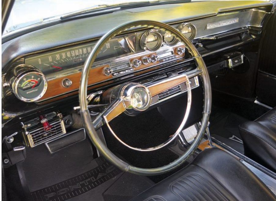
Beautifully crafted instrument panel features safety pad on top as standard; woodgrain on dash and steering wheel same as the console. Manifold vacuum gauge on far left was optional, but three gauges in the center—fuel, clock, and battery—were standard equipment.
