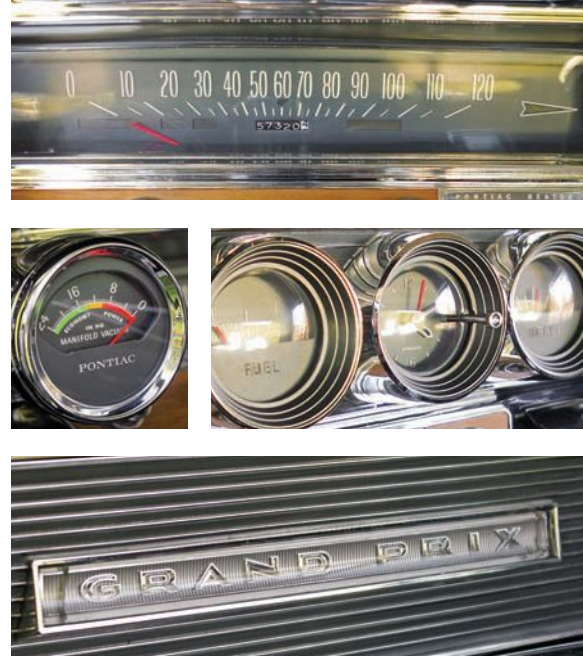
Beautifully crafted instrument panel features safety pad on top as standard; woodgrain on dash and steering wheel same as the console. Manifold vacuum gauge on far left was optional, but three gauges in the center—fuel, clock, and battery—were standard equipment.
