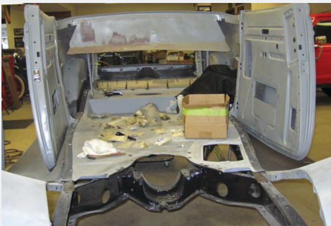
Although one patch panel was still required to complete the forward floorpan, at this stage the parts of the body are being test-fitted for fit and finish against each other and the frame prior to paint. Critical flaws are easier to correct at this stage of the restoration.
