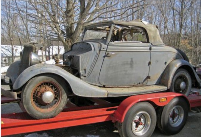
One of the first images of the newly purchased 1934 Ford Cabriolet, replete with visible rust weeping through an ancient layer of gray primer. The top was in shambles, but the wire wheels were surprisingly undamaged. The hood was stored during transport.
