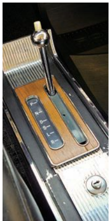
Ribbed stainless steel and woodgrain console was a standard accessory on the Grand Prix; it featured a lockable compartment. Below the rear speaker resides the armrest, which folds down for added comfort. Original black upholstery is hardwearing Morrokide vinyl.
