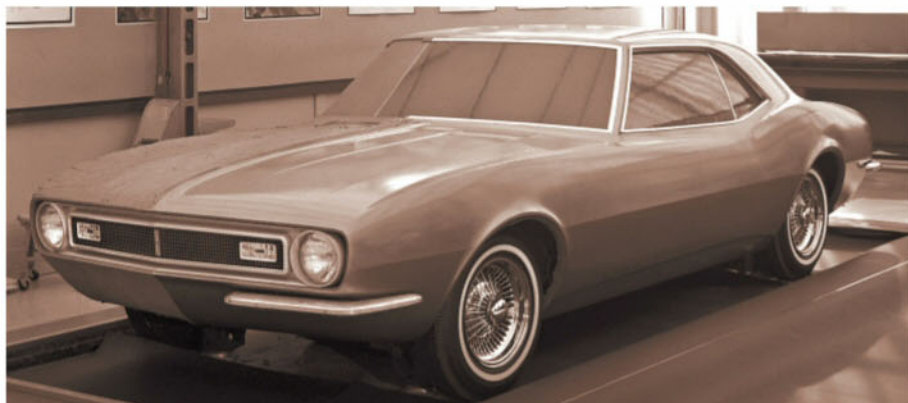
This front view of the clay model reveals rectangular instead of the round parking lamps that the 1967 production car ultimately received, and grille differences.
