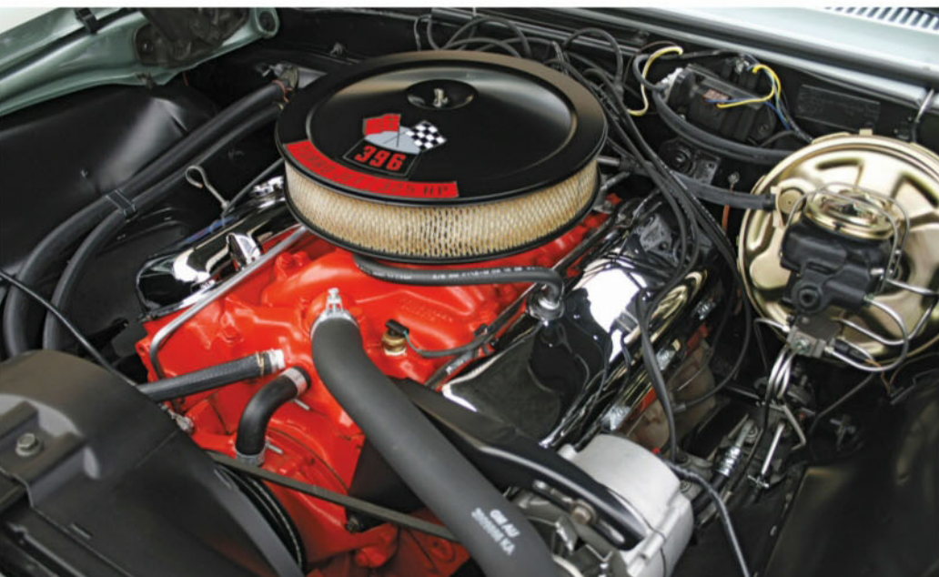
The 325-hp, 396-cu.in. big-block V-8 was released partway through the model year. It featured a Quadrajete carburetor, oval-port cylinder heads and a hydraulic-lifter camshaft.
