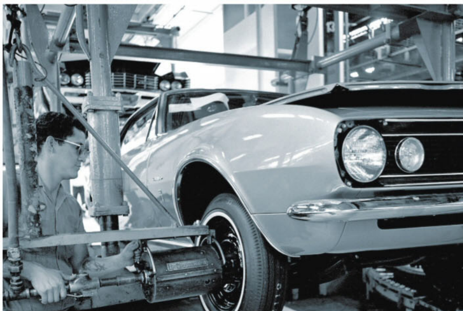
One of the engineering requirements for the Camaro was that it could be built on the same assembly line as other models. Note the full-size Chevrolet in the background of the previous assembly line photo and in this one. This Camaro is awaiting its headlamp trim installation.
