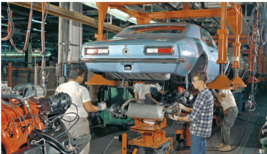
Moving along the assembly line, the Camaro nears the installation of its drivetrain, suspension and exhaust. Shown are the standard tailamps, with integral back-up lamps.
