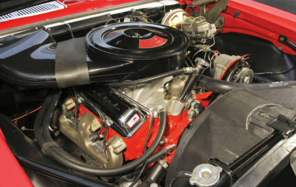
An optional plenum air intake is revealed on the underrated, Holley-carbureted, solid-lifter-camshaft, 302 engine in this Z/28 RS.
