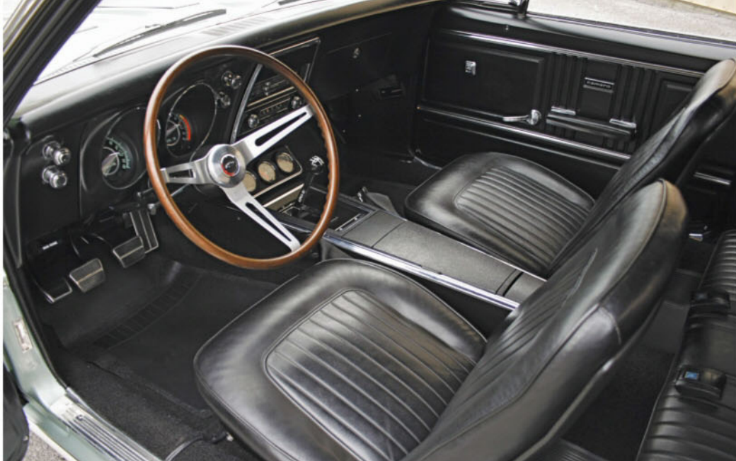
Standard interior features bucket seats, with optional woodgrained plastic steering wheel, four-speed, console, Special Instrumentation, and power windows.
