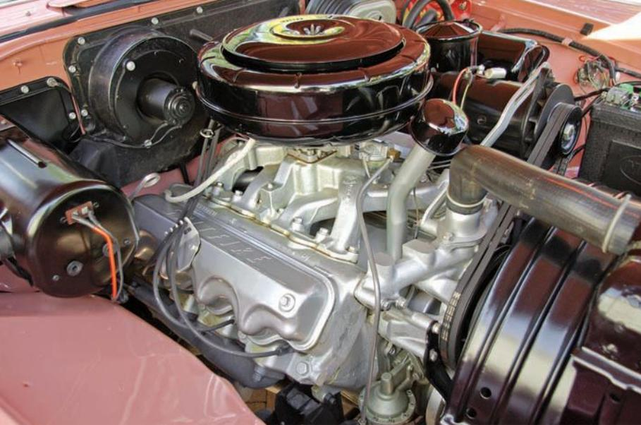
**Recognizable by the scalloped valve covers, Chrysler's 331-cu.in. Spittfire polyspheric V-8 engine from 1956 never made the headlines the way the Hemi V-8 did.**
