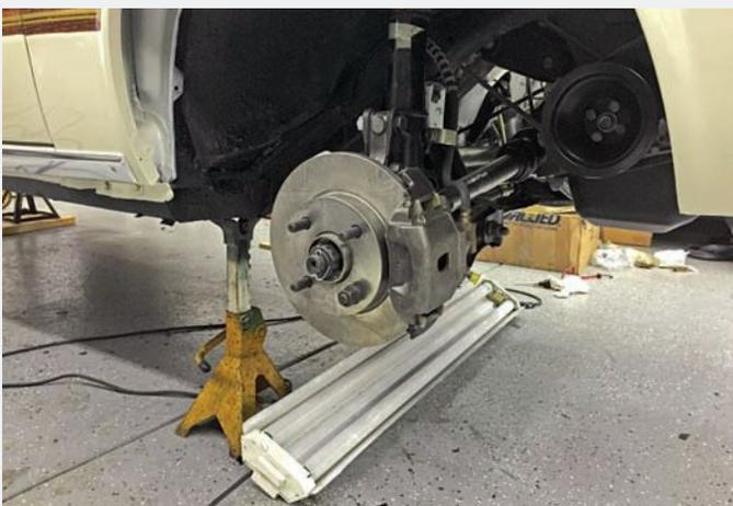
Up front, NOS MacPherson struts (with the parts decal still in place), steering knuckles, hubs, CV-style drive shaft assemblies and disc brakes were bolted in, and new lines and hoses were employed. Single-piston calipers squeeze the pads against rotors.
