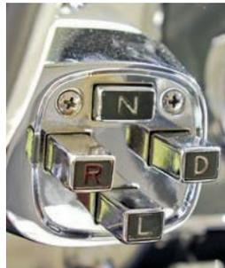
Excellent and thorough restoration of this 1956 Windsor Newport four-door hardtop shows in the interior details as much as outside the car. Chrysler introduced its pushbutton transmission control that year with the two-speed, fully automatic PowerFlite transmission.
