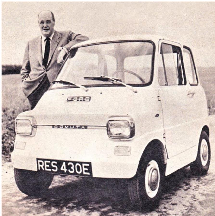
McCahill traveled the globe; in England he tried Ford's experimental Comuta in 1967. Designed as a full-on electric car to reduce congestion and pollution, the Comuta had four 12-volt, 85-amp lead batteries, a top speed of 37 miles an hour, and a 37-mile range at 25 mph.
