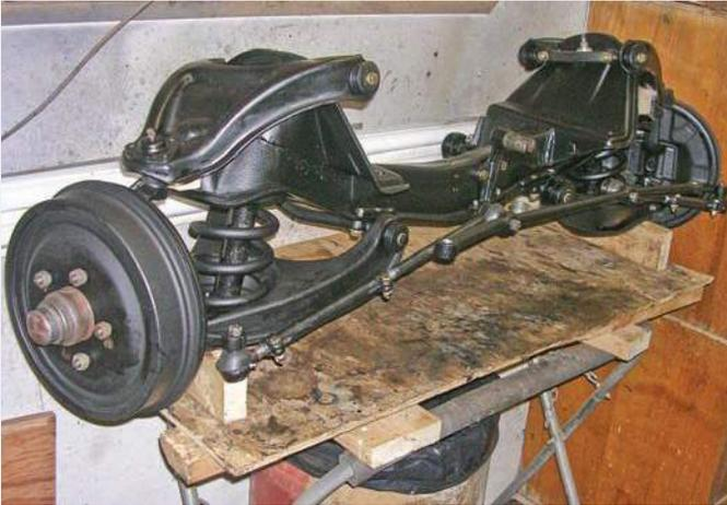
Both the front and rear suspension systems were removed from the chassis as subassemblies. Each was then broken down into individual components, painted, and carefully rebuilt. This is the completed front suspension assembly ready for installation.
