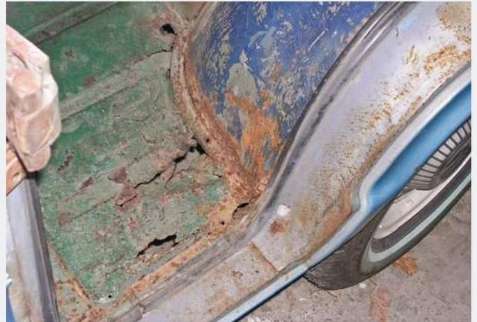
Even before sandblasting, the stability of the driver's-side floorboard is clearly completely compromised; a condition repeated on the front passenger side of the Greenbrier, due, in part, to its water-catching design and wheel proximity.
