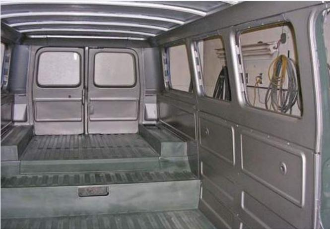
With all of the metalwork completed throughout the Chevrolet, the interior was the first to receive paint. Here, three of the four different colors used to finish the cabin can be seen, including Fawn Metallic side panels, a color first used in 1962.
