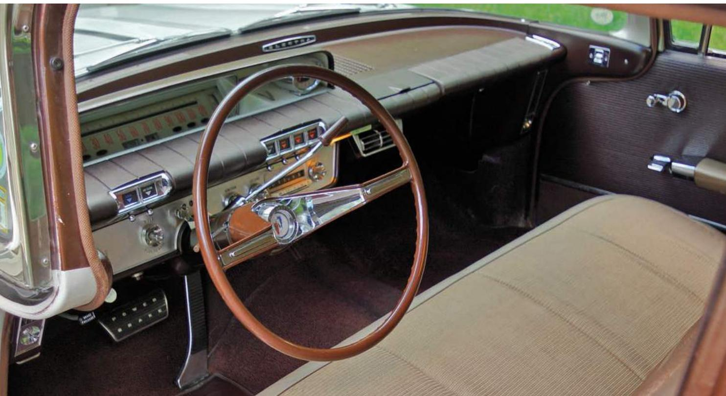
The softly sprung foam-cushioned upholstery on the power-activated, six-way adjustable, wide bench seat is still covered in the original cloth and vinyl fabric. Flat-top instrument panel adds to the cabin's airiness, which is enhanced with the wraparound windshield.
