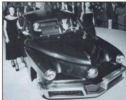
**PRESTON TUCKER INTRODUCES THE** Tucker Torpedo, powered by a rear-engine capable of 166 horsepower. The prototype has been making its rounds at various auto shows, and it will be interesting to see what becomes of this venture. Only 49 inches tall, the car has many innovative safety features, including a cycloptic center headlamp that turns with the steering wheel, pop-out windshield, and disc brakes. In addition to its safety features, it boasts performance with a top speed around 120 mph.
