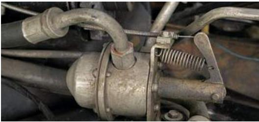
Original 401-cu.in. V-8 is called the Wildcat 445 — it has never been rebuilt; the A/C's hot-gas bypass valve activates via the "COLD" lever on the left side of the dash; radiator "Caution" decal is original to the car.
