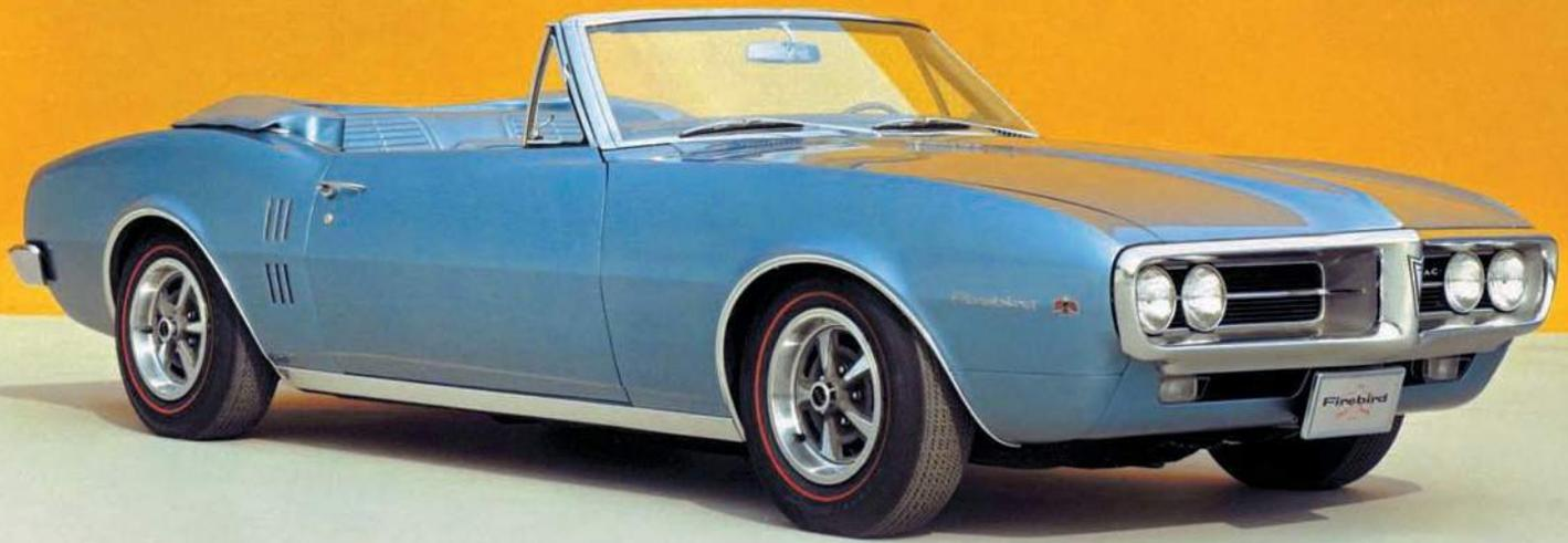
**This OHC-6-equipped Firebird convertible is also a pre-production car. Notice the “Firebird” callout and emblem appear to be decals. The extended horizontal bright grille trim and the arrowhead emblem shown here were only used on the production Firebird 400s.**
