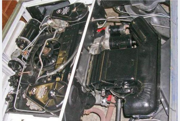
In this image, the engine bay has been painted Cameo White, and both the re-detailed 164-cu.in., air-cooled six-cylinder and the transaxle have been reunited to the chassis. Interestingly, the block is from a passenger car and did not require a rebuild.
