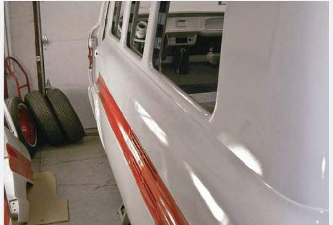
Rather than retain the original dark blue/light blue two-tone scheme, Cameo White and Cardinal Red were chosen. A PPG-basecoat/clearcoat system was used, consisting of two color coats and four applications of clearcoat. Sanding and polishing followed.
