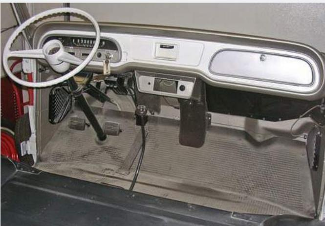
With the paint process completed inside and out, final reassembly could begin. Here, new rubber floor mats have been secured into position, while the instrument panels had been fitted and wired. The radio and other trim parts have yet to be installed.
