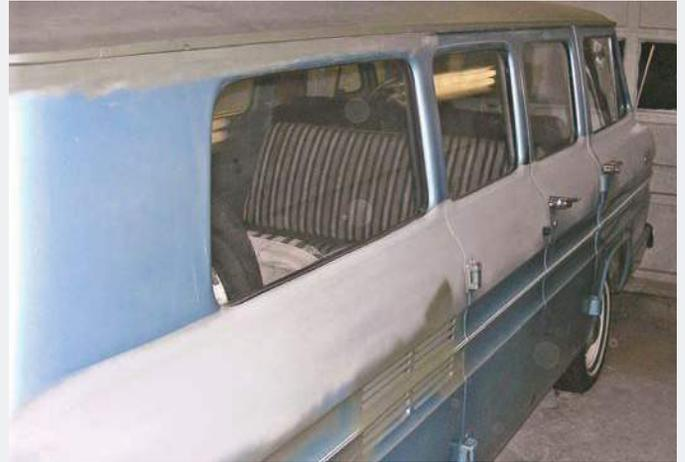
The first part of the restoration to be accomplished was the elimination of surface rust on the upper sections of the body, roof, and within the rain rails. Corrosion was removed via sanding, and the metal was quickly sealed in self-etching primer.
