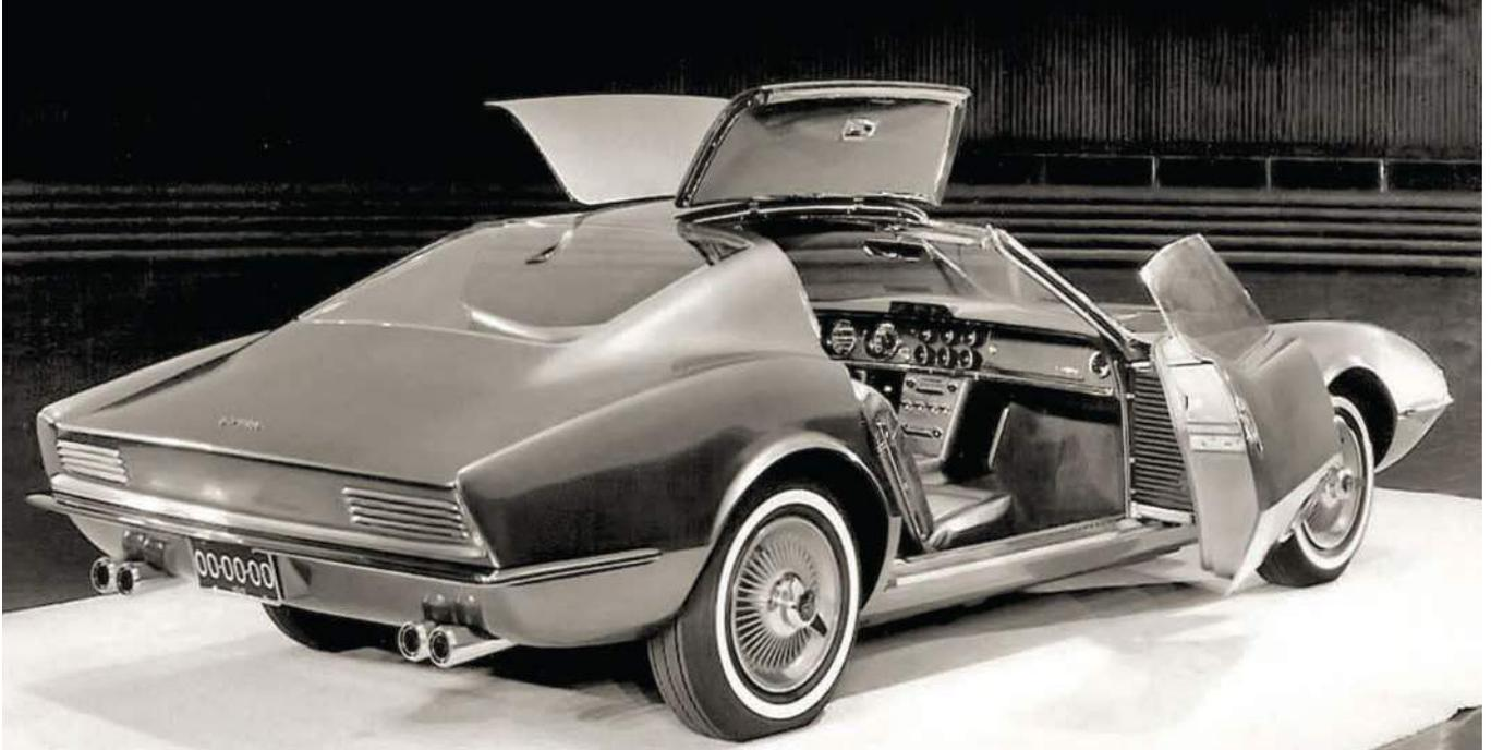
The XP-798 was an innovative four-seat sporty personal car. However, the features that made it unique, like its fiberglass body, flip-up roof panels, and extended doors with a one-off hinge system, also made it too expensive to build, and difficult for GM to justify as a Pontiac exclusive. Thus, it remained an idea car.
