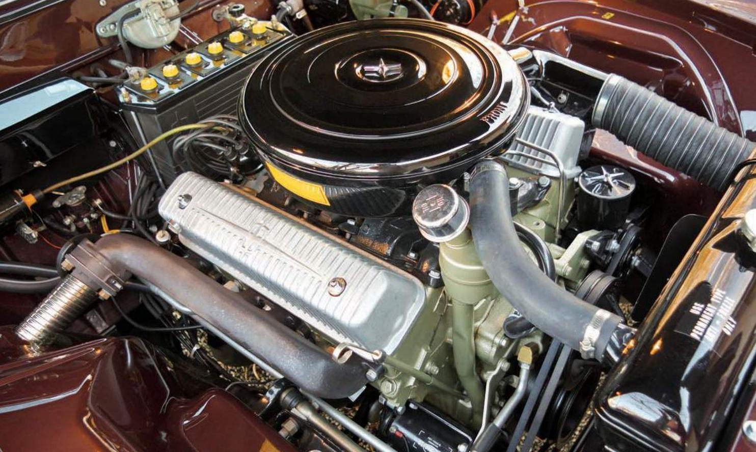
Lincoln extensively upgraded and modified its V-8 engine for 1956. Displacing 368-cu.in. and sporting a 9.0:1 compression ratio, the powerplant breathed through a Holley four-barrel carburetor to produce 285 horsepower and 402 lb-ft of torque.
