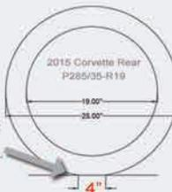
With a FlatStopper, the contact area increases by a factor of three
