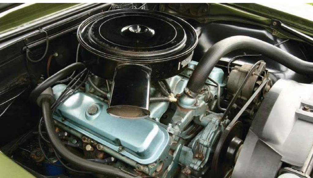
This original, low-mileage 326 H.O. engine features a Carter AFB carburetor, standard log manifolds, and dual exhaust with a crossflow muffler.
