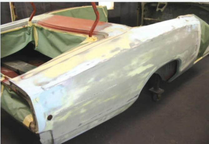
Vertical flanks from reproduction coupe quarter panels have been butt-welded into place. Welds were then ground smooth, and the metal was sealed in a layer of epoxy primer. Here a skim coat of filler has been applied and block-sanded smooth.
