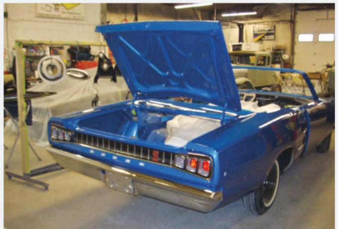
Though much of the interior, front windshield, and convertible top have yet to be fitted, at this point in the project the decklid has been installed and aligned, while several pieces of rear panel trim have been returned to the Coronet.
