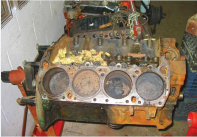
During downtime between stages of body repair, other aspects of the restoration were accomplished, such as rebuilding the Mopar's 330-hp, 383-cu.in. V-8 engine. During disassembly, a massive mouse nest was discovered in the lifter valley.
