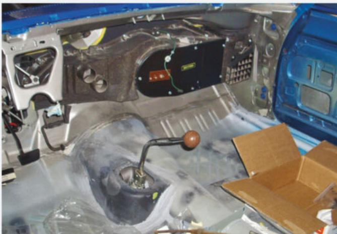
Before floor carpet and seats could be installed, the interior side of the front firewall needed to be repopulated with pedal assemblies, some of the wiring harness, and the car's climate-control system. Note the transmission is in place.
