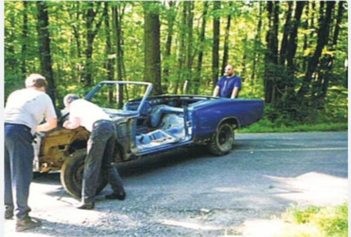
Flash forward to summer 2002. Having been in garage storage since the winter of 1979-'80, the convertible's restoration has finally begun. Except for the suspension and differential, the unit-body Dodge has been completely disassembled.
