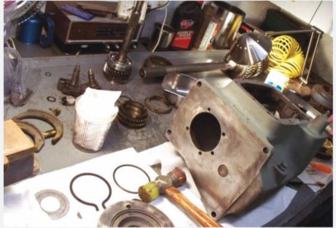
Like the engine, the Coronet's original four-speed manual transmission, fitted with a Hurst shifter on the assembly line, was disassembled and rebuilt. With no wear to speak of, it only required new seals and bearings.
