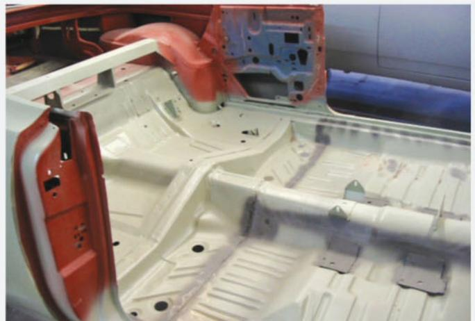
Convertible floorboards tend to suffer the wrath of the elements from both sides, usually with devastating results. This Dodge required a front floorpan replacement, which was butt-welded into place. The seam can still be seen here, under darker primer.
