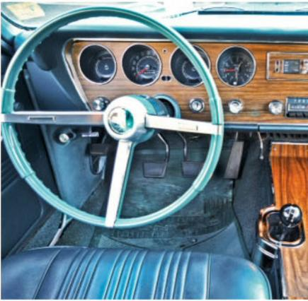
The interior is original, and the woodgrain dash appliqué was included when the console was ordered. A lever under the dash is for a windshield-washer hand pump (since removed) that was added when the stock pump expired.
