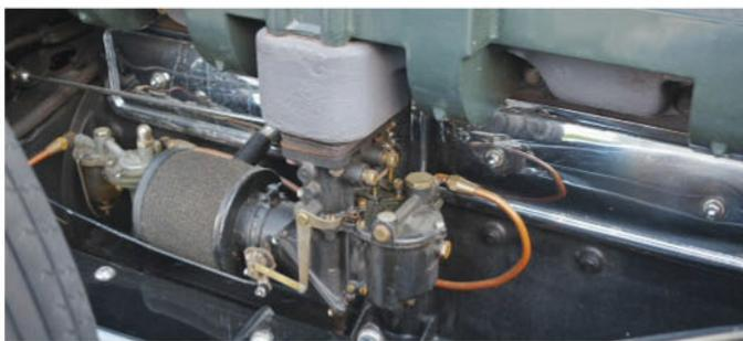
**This new-for-1929 L-head straight-eight sported a standard oil filter and two-barrel updraft Stromberg carb. The generator was driven off the timing chain, and it, in turn, drove the water pump.**
