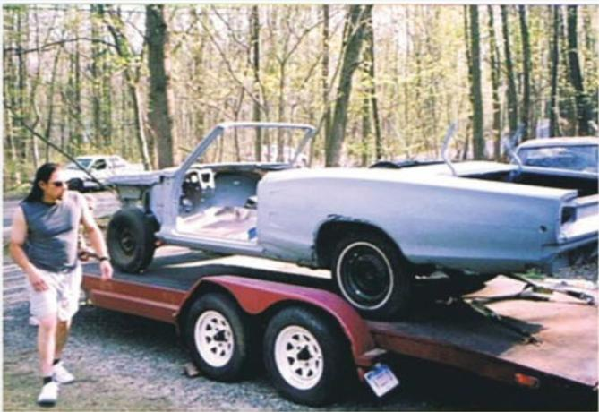
After disassembly, the body was sent to a facility for media blasting. The process exposed bare metal and extensive rust, attributed to the rigors of daily driving; it can be seen around the rear wheel opening. Primer was applied to protect the metal.
