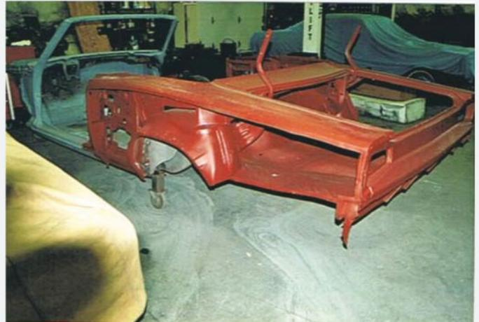
The restoration was put on hold until Wayne could find a facility capable of managing the rest of the effort could be found. In 2004 it resumed, and here the vertical flanks of the rear quarter panels have been removed, as well as one part of the trunk floor.
