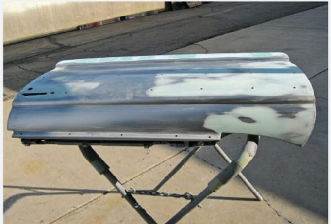
After fabrication work had been completed, the restoration team applied a skim coat of filler on each of the body panels where needed. The material was then sanded smooth, with special care taken to maintain factory body lines during the intensive process.
