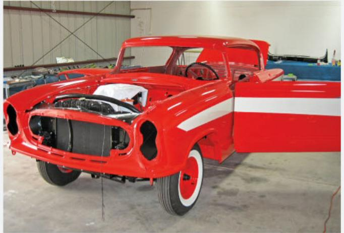
At this stage, the body has received its finish coat of Mardi Gras Red trimmed with Frost white paint. The car's suspension, engine, transmission, and remaining driveline system have been reinstalled, while the doors have been hung and balanced.
