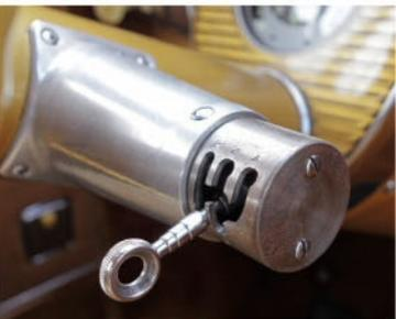
**Radio and all instrumentation crowd behind the Lincoln steering wheel, leaving the passenger's side clear for a crash chamber. Glovebox is integrated into door, and pre-selector shifter sprouts from the steering column.**
