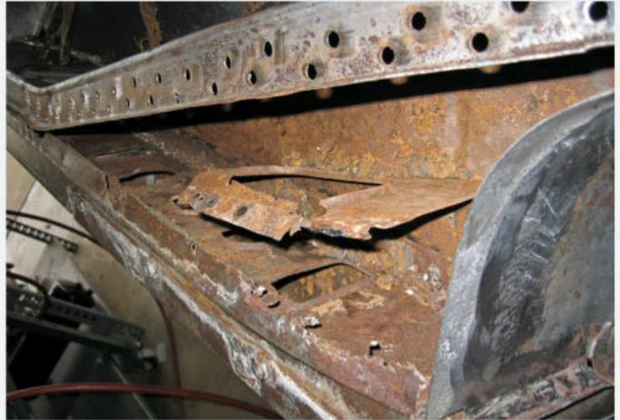
After disassembly, the body was mounted to a rotisserie, which provided easy access to every surface of the unit-body Nash for the restoration team. This included the underside, where some corrosion within and near the rocker panels was found.
