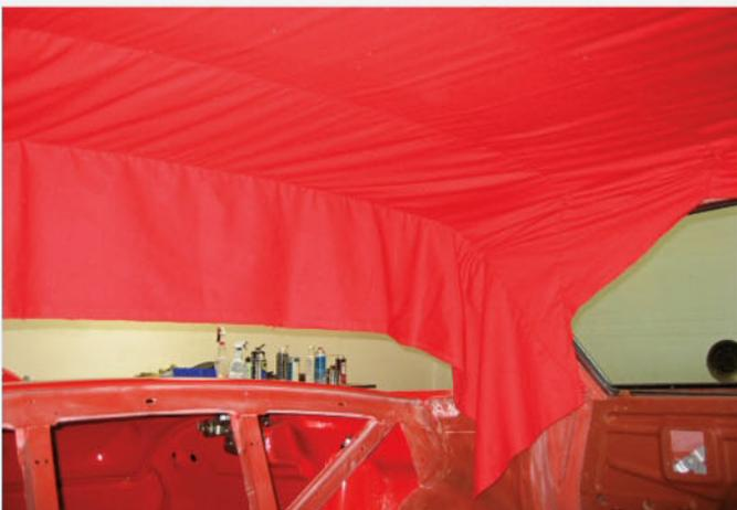
While it may seem easier to begin installing new upholstery with door- and side-panel assemblies, the best method is to begin with hanging the headliner, as seen here. The top-down method enables all seams to be hidden by the lower panels with less effort.
