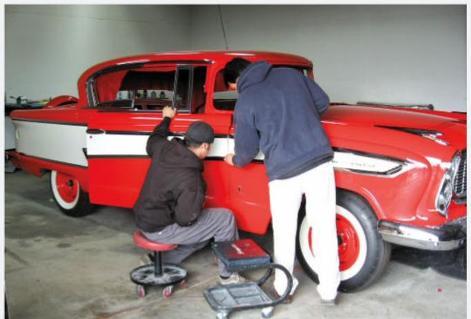
Although the doors had been hung and balanced earlier, a second alignment was required during the reinstallation of the exterior trim. Improper installation wouldn't just look bad, it could lead to damage at the trim extremities, such as the door/fender junction.
