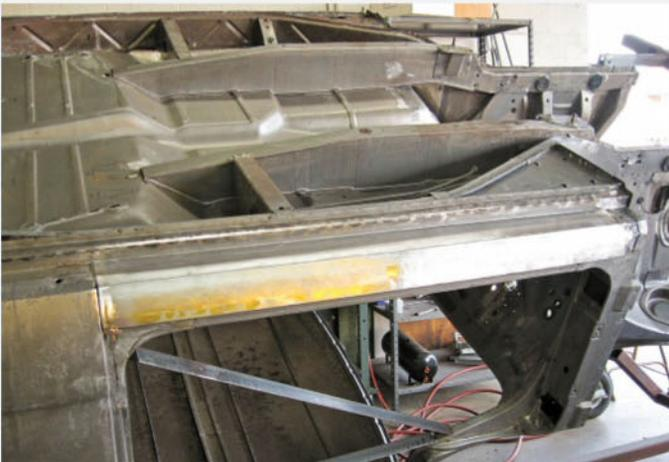
A keen eye will note the temporary bracing within the door opening, which is helping maintain the car's structural rigidity. At this stage, a new outer rocker panel has been fabricated and is being test-fitted for correctness.
