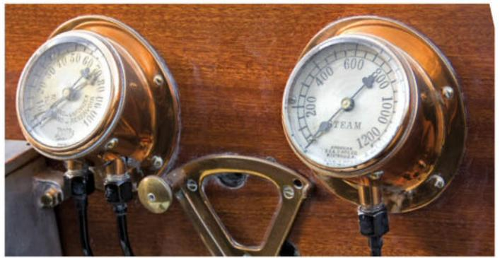
**Unconventional controls on the 1909 White Model M steamer include a hand throttle on a concentric ring inside the steering wheel, gauges for steam temperature and fuel vaporizer, and pedals for the fuel-feeding air pump and simpling valve, along with a brake pedal.**
