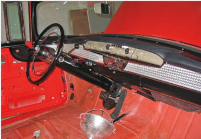
Reassembly of the hardtop's interior began with the installation of the completed instrument panel, steering column, and pedal assemblies. Hidden from view is a new wiring harness. Note that the owner resisted adding air conditioning from the parts car.
