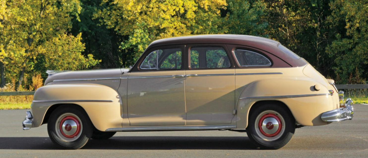
not seem as heavy as many modern automobiles, keep in mind that its six-cylinder engine produces only one horsepower for every 28.8 pounds it has to move.
