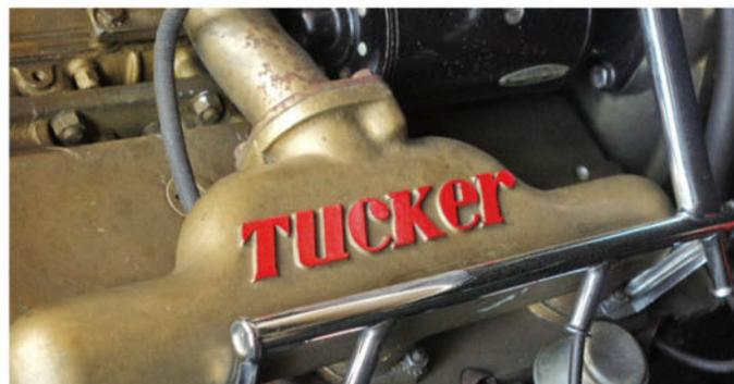
**The originally planned low-revving, massive 589-cu.in. engine was replaced early on with a Franklin flat-six engine originally designed for helicopters and significantly reengineered by Tucker to accommodate water cooling. Despite the odd engine, Tucker used a thoroughly conventional 6-volt, positive-ground electrical system and battery/coil ignition. Dual exhaust pipes split to six tips to hint at cylinder count.**
