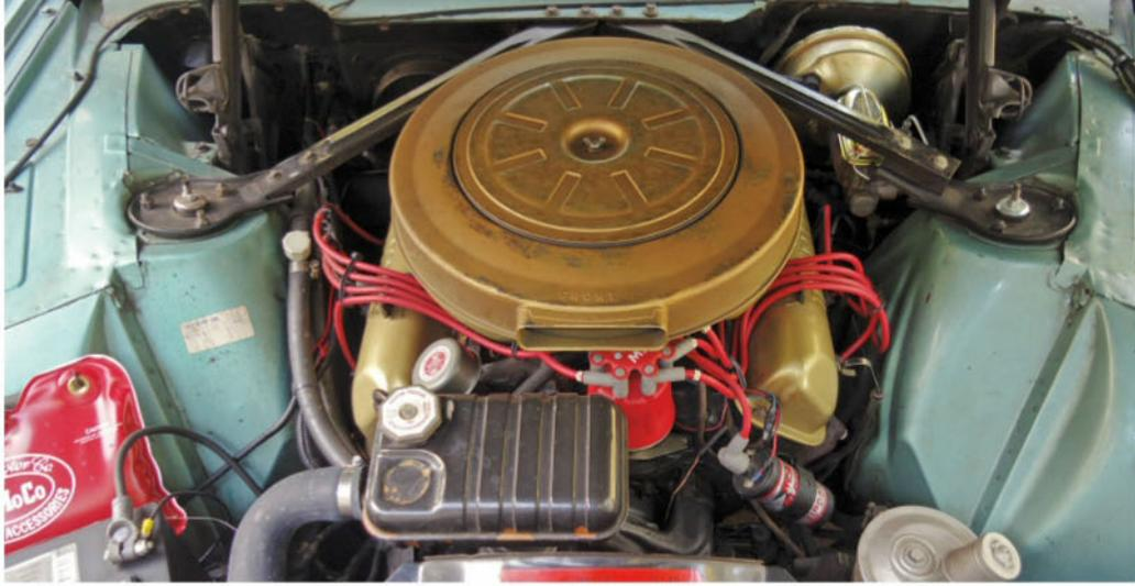
Limited use led to the 300-hp, 390-cu.in. V-8 developing many fluid leaks, which were quelled by installing new gaskets. This engine, and Cruise-O-Matic automatic transmission, were later completely rebuilt. A front disc-brake/dual-master-cylinder conversion was performed for added safety in modern traffic, the switch to high-performance ignition wires and coil was made, and the car now rides on Granada wheels.
