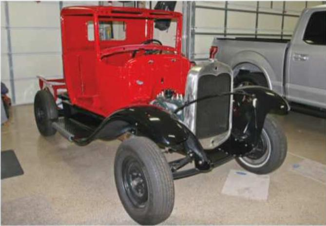
The cab, properly aligned to the frame, is bolted into place, while a few components have been secured to the firewall. Note that, in addition to the fenders, the running boards and headlamp bar are installed; the steel wheels are temporary.
