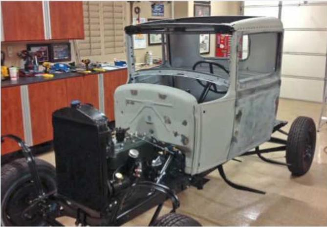
At the conclusion of Part I of this story, the body had been returned to Kevin in primer. It was then partially reassembled on top of the restored chassis. The test-fit enabled the team to check tolerances and alignment, and make corrections prior to paint.
