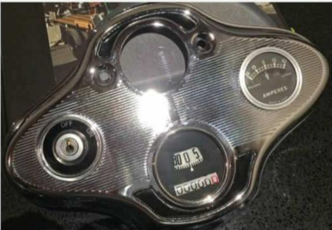
Earlier, several pieces of trim were replated, while others were polished to a factory-new shine, including this simple-yet-detailed instrument bezel. The bezel was repopulated with restored gauges; it would then be installed in the cab as a sub-assembly.
