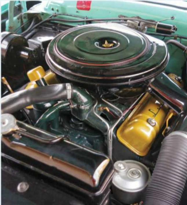
According to this Premiere's owner of 36 years, the original 300-hp 368-cu.in. V-8 engine has yet to require any major work, aside from detailing.
