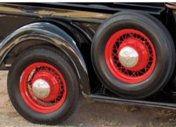
The 1935 restyle included moving the pickup's spare tire from the front fender to the bed side.
