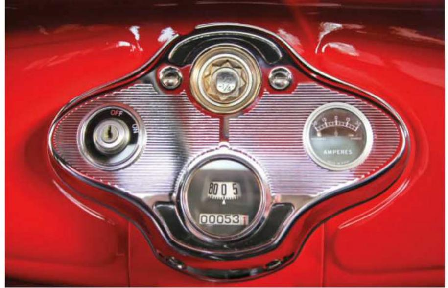
**Ford updated the appearance of the Model A's basic instrument panel for 1931, which was now chrome plated and featured a ribbed wood motif. New varnished wood complements the pickup's bed, the one visual deviation from factory-stock configuration. The gloss black rectangular plate is centered over the differential.**
