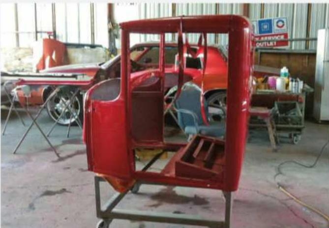
The Ford cab has just emerged from the paint booth after receiving a few coats of DuPont enamel paint matched to Vermillion Red, a hue original to the 1931 Ford color spectrum. The cowl and hood were also painted the same color at that time.
