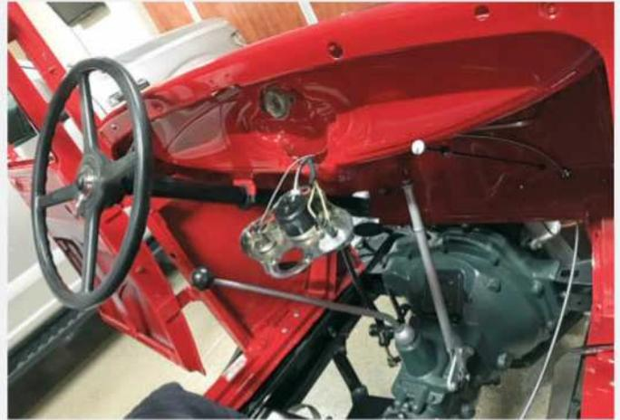
Reassembly has commenced in earnest with the fitting of the cowl/fuel tank with its integral fuel gauge, the latter slotting into the open position on the instrument panel. A new wiring harness was obtained earlier. Note that the doors have been hung.
