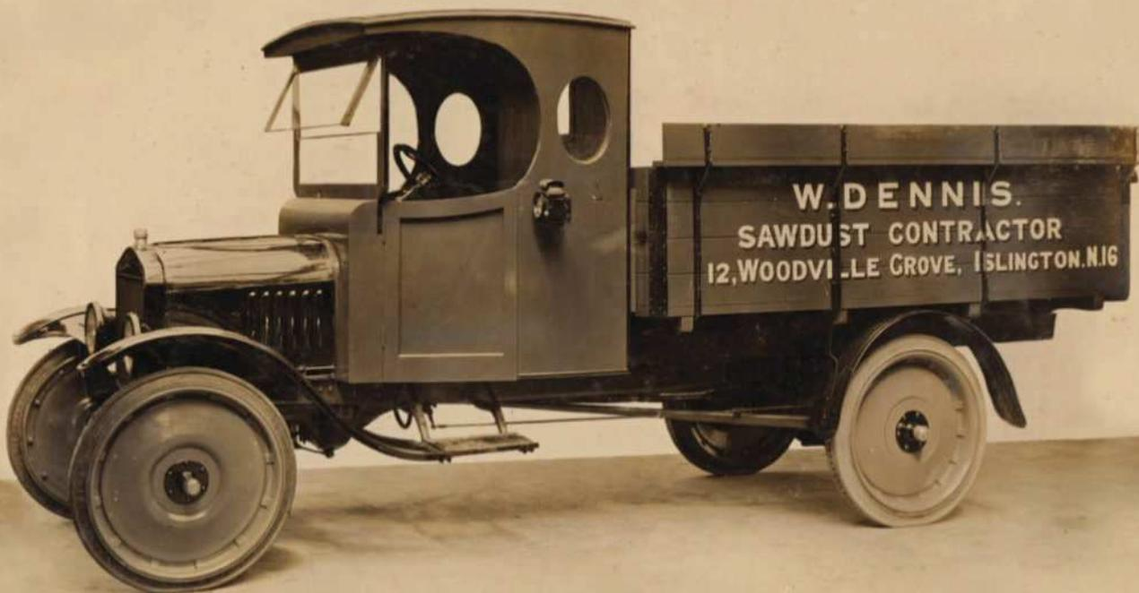
With special disc wheels fitted with solid rubber tires, and a heavy, substantial body and bed area, this truck was designed to haul sawdust. Colors most likely were bright red wheels and maroon coachwork.
