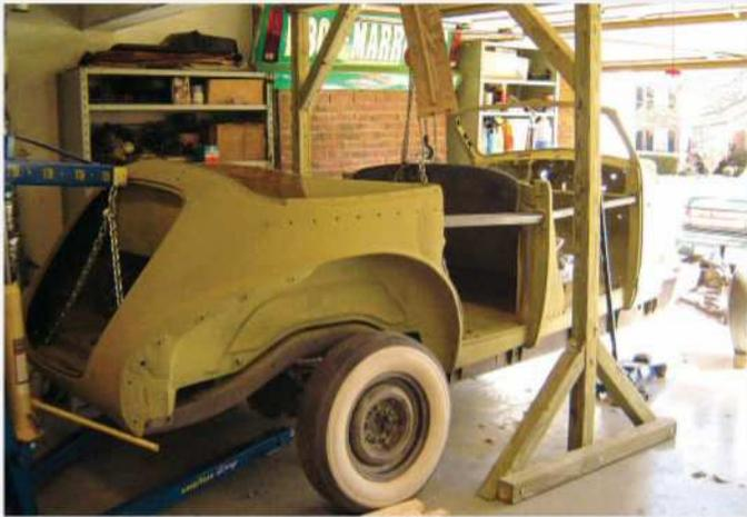
In order to hold the body once it was removed from the chassis, this gantry was made out of 6 x 6 lumber. Notice the body here has been covered in an etching primer to prevent any corrosion to the previously media-blasted surface.
