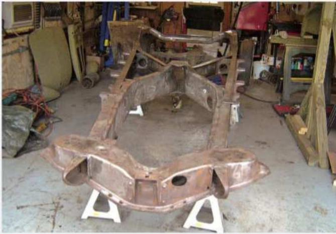
Separated from the body and with the suspension and braking components removed, the frame with Buick's strong "girder X-type" design (clearly visible here) was stripped to the bare metal for refinishing and reinstallation of the other chassis components.
