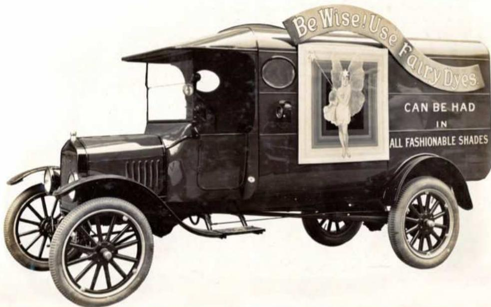
This body on a one-ton Model TT truck chassis has an elaborate ribbon-shaped sign and a huge painting of a fairy that was the logo for the Fairy Dyes company that bought the truck. Sidelamps were fitted below each oval window.
