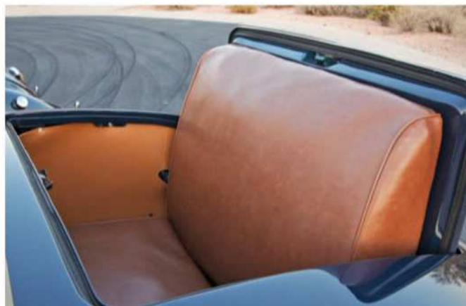
**Rumble seat was finished in the same materials as the interior. Two steps on the passenger's side simplified access.**
