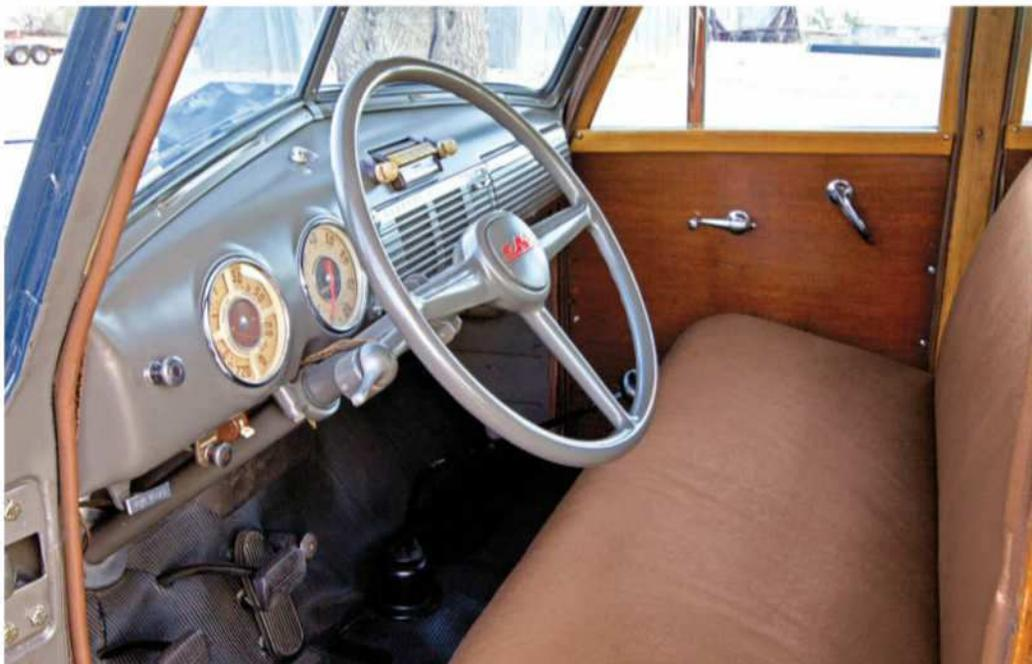
1947-'55 GM truck cabs were more spacious, better ventilated, and easier to see out of than previous haulers. Inside a wood-bodied rig, creaks and groans from the millwork are common.
