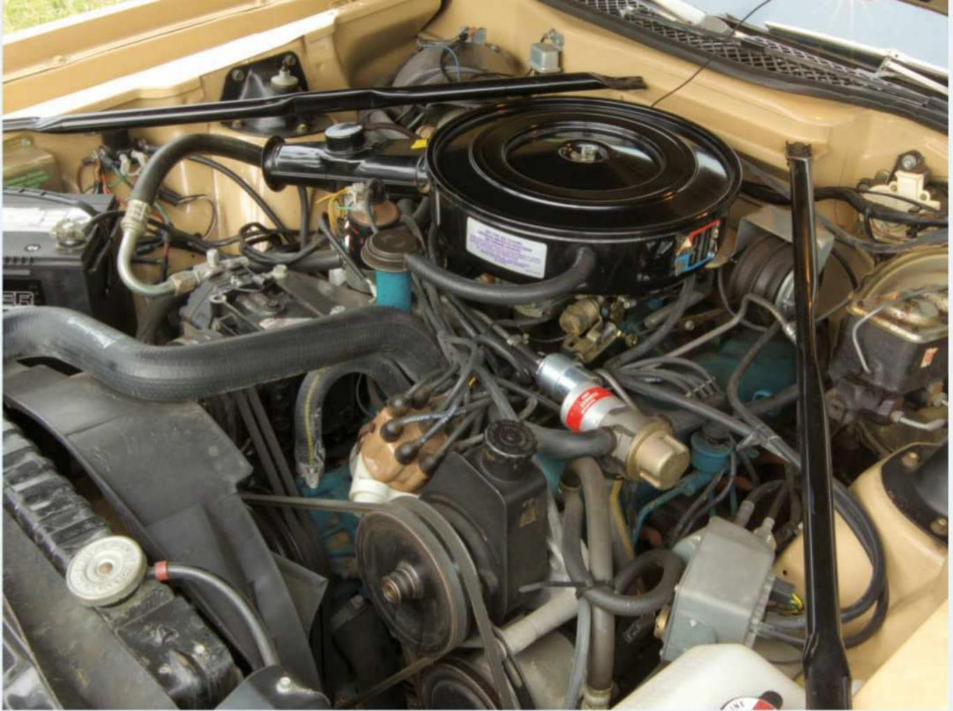
The 304-cu.in. two-barrel V-8 was standard for Matadors sold in California in the 1977 model year. Note the factory markings and decals in the 101-mile Sand Tan engine compartment. Barcelona II exterior paint schemes were Sand Tan/Golden Ginger or Autumn Red/Claret.
