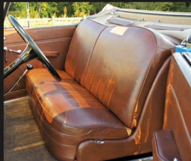
While closed Series 90 cars got plush mohair velvet upholstery, open cars received less-luxurious but more weather-resistant leather. Instrumentation included ammeter, temperature gauge, oil-pressure gauge, speedometer, and clock. "Octane Selector," like the spark levers of old (and today's computers), allowed adjustment of ignition timing based on the fuel grade onboard.
