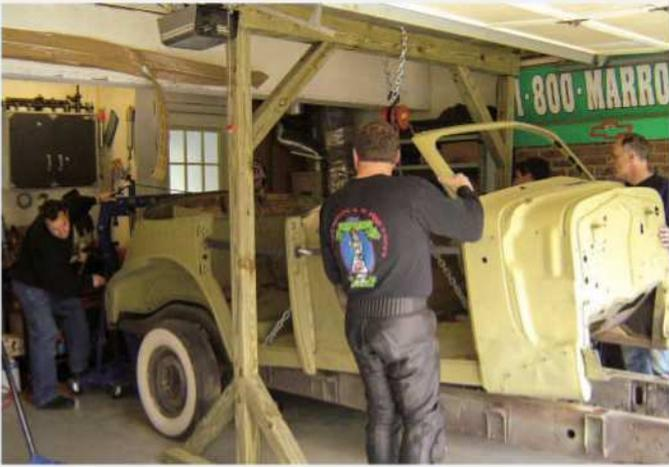
For the process of removing the body from the chassis, friends were recruited and used both the gantry and an engine hoist to make a smoother effort of the chore, and were able to roll the chassis out underneath the suspended body.
