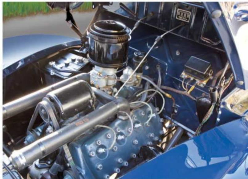
**The De Luxe model’s new “helmet” hood offered simpler access to the legendary flathead Ford V-8 engine.**
