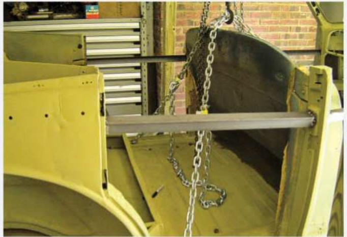
Despite the chains holding the body to the gantry (and eventually saw horses below supporting it), the convertible body, minus its doors, needed additional structural strength. So, four angle-iron supports were welded in between the door pillars.
