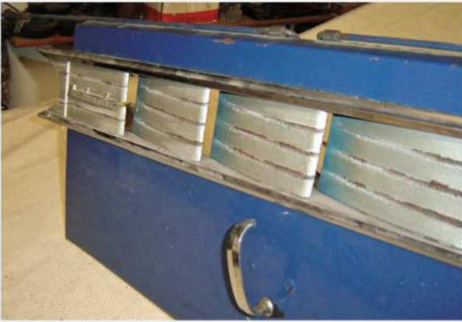
Though the car was largely complete and relatively solid, pitting of the bright work, surface corrosion and other degradation was present throughout. Likewise, an older restoration had kept the car on the road, but was not authentic.
