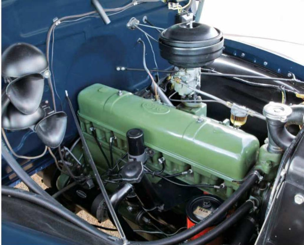
Owner-rebuilt 228 GMC six-cylinder breathes through a Carter one-barrel carburetor and was rated new at 93 hp. Oil bath air cleaner was an option, the Fram oil filter was an accessory.
