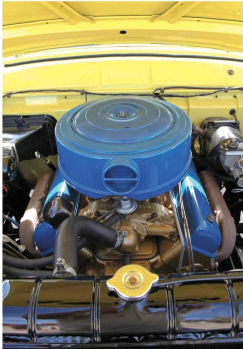
New to the 1956 model year was Ford's venerable 312-cu.in. V-8 engine, which helped Mercury set 20 performance records on Daytona's beach. Coupled with a Merc-O-Matic, it made 225 hp.
