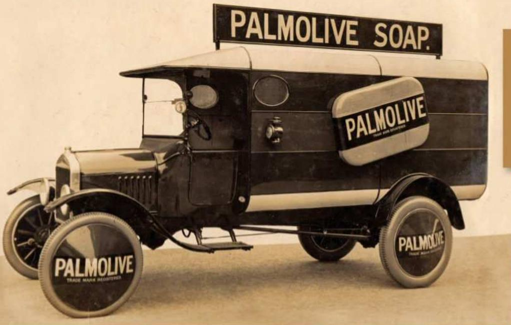
◀◀ This van featured a fancy roof sign and three-dimensional panel for the body side, along with metal discs fitted over the wood-spoke wheels. All lettering of the well-known soap company's name was done by hand. This was one of the few trucks that also had a plated radiator shell and headlamp rims.
