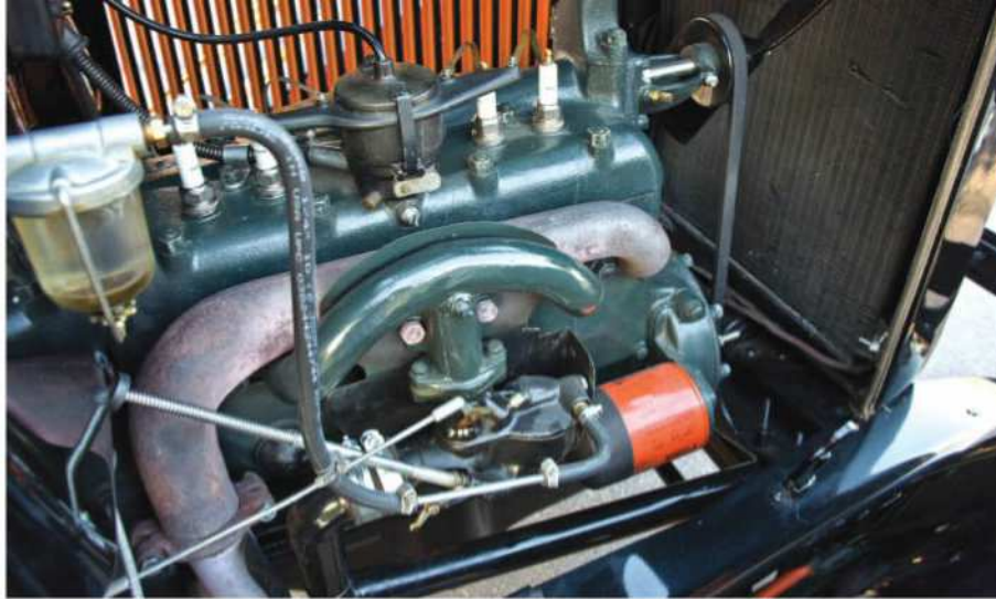
This old tanker is driven fairly regularly, so the owner has made some practical modifications including a spin-on filter and fabricated heat shields around the carburetor and manifold.
