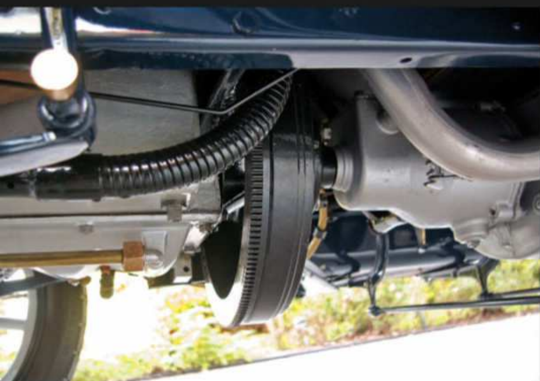
The ring gear is the only clue that this car was retrofit with electric start. Brass and pinstripe details extend under the car.
