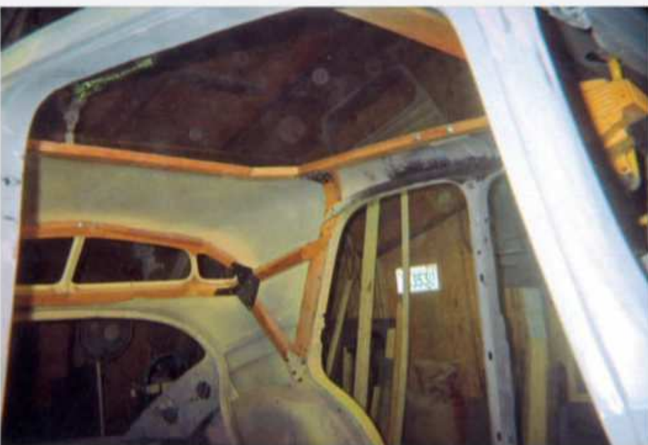
The next phase of the restoration was the body's interior framing. Original framing, exclusive to the Land Cruiser, was made from ash. Native ash was harvested, milled, and cut to final form using remnants of the original material as templates.
