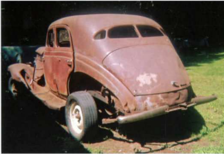
This pre-restoration image of the President Land Cruiser only hints at its condition beyond the doors. Its front end had virtually collapsed from corrosion, and the frame fractured as it was being loaded for its relocation from Massachusetts to Connecticut.
