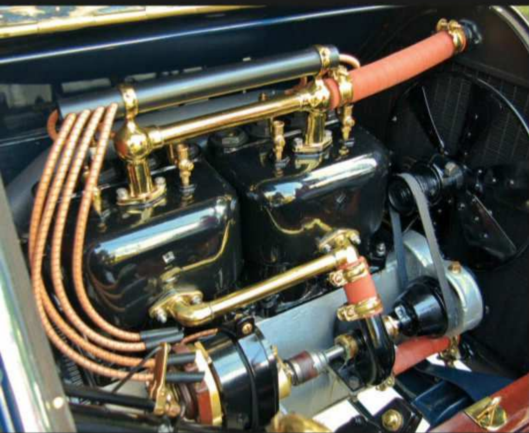
Ignition is via magneto. Note that the cylinder heads are integral with the cylinder block, but the crankcase is separate.
