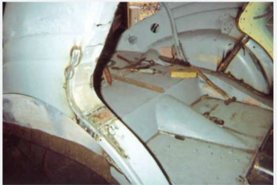
A great deal of patience was required to attain a proper body alignment, necessitated by door function. Any deviation, and none of the doors would open or close properly. After many adjustments, the seams were permanently fused using a MIG welder.
