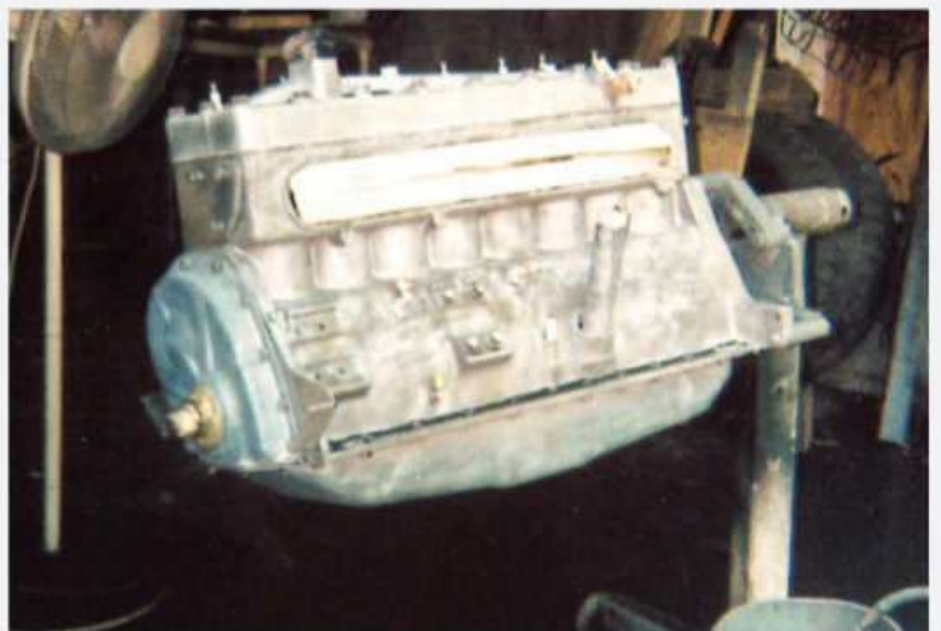
Powering the President series was Studebaker's 250-cu.in. straight-eight. Though the engine had been rebuilt years prior, a compression check and bearing inspection was performed; all was satisfactory. The 110-hp engine was cleaned and later painted.
