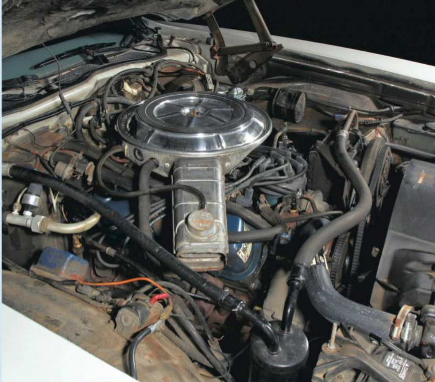
The 351 Windsor two-barrel V-8 is also original and has required only minor repairs and regular maintenance since the current owner purchased it.
