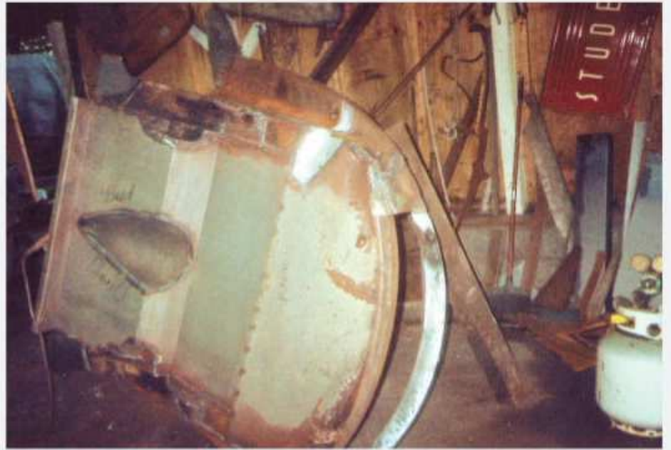
The Studebaker's restoration began with extensive bodywork that was performed one salvaged section at a time. This is the underside of the rear section, which was unique to the Land Cruiser design. New floor pans were fabricated, then MIG welded into place.
