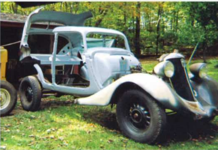
At this stage, repairs to the Studebaker's basic body shell have been completed. Each section still needs to be stitched together. A bucket loader assisted the effort and, after some tweaks, the seams were held together with several tack welds.
