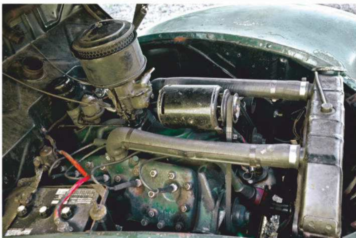
The 85-hp, 221-cu.in. flathead V-8 needed a rebuild at 85,000 miles because the block cracked while the car was inactive. The odometer now indicates about 20,000 added miles.
