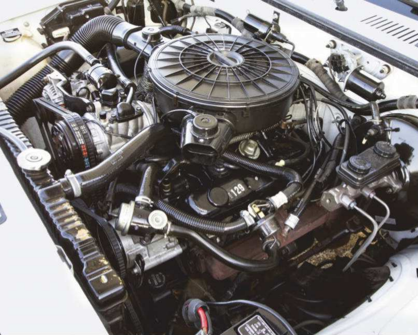
A throttle-body injected 318-cu.in. V-8 filled the Dakota's smallish engine bay. It made just 175 hp, but electric fans gave it a 5-hp edge over the standard light-truck version.
