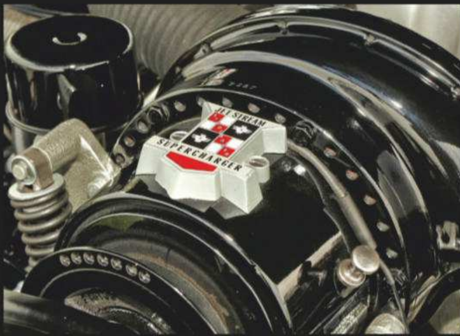
A McCulloch VS-57 centrifugal supercharger delivered compressed air to a Stromberg WWG-122A two-barrel carburetor in a cast-aluminum housing. Output of the 289 supercharged V-8 was 275 horsepower.
