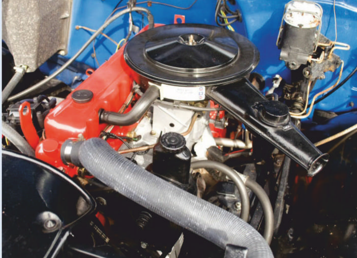
The original 250-cu.in. straight-six still powers this one-family 1972 GMC 1500. It soldiers away with its original internals, though it's had some gaskets, new paint, and an upgrade to HEI ignition.
