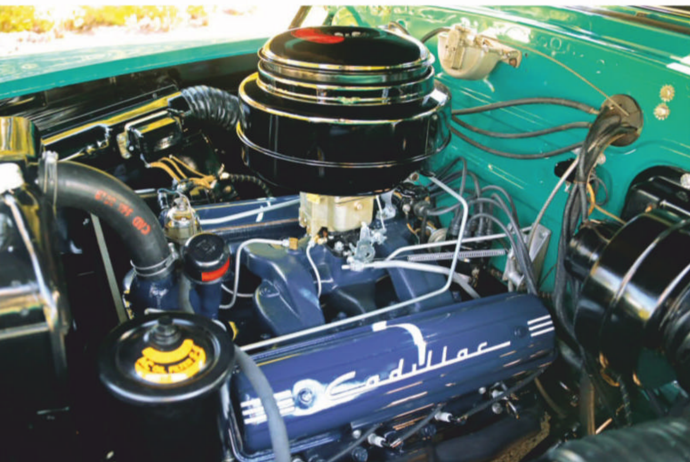
Cadillac's primary mechanical improvement for 1949 was the introduction of the 160-hp 331-cu.in V-8. It was 188 pounds lighter yet more efficient than the old flathead V-8.
