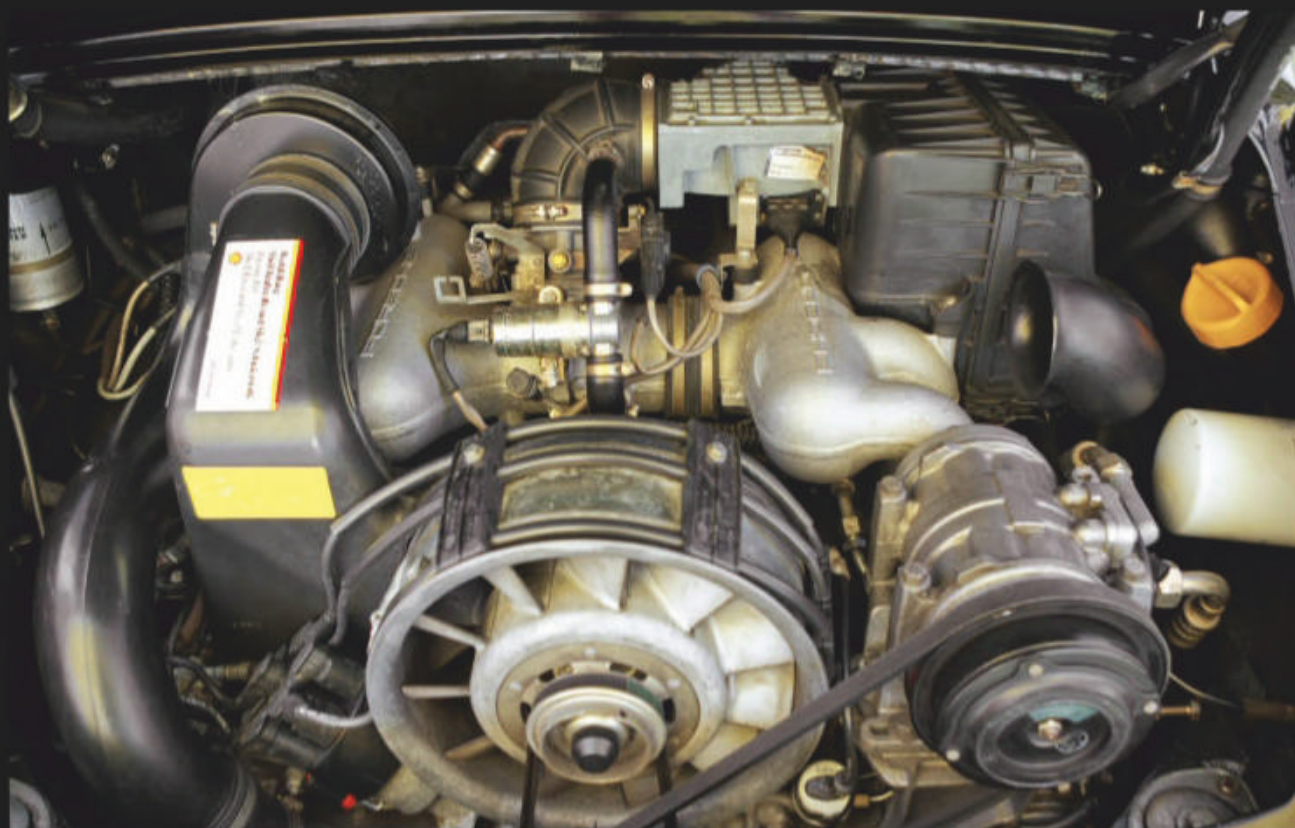
This naturally aspirated, fuel-injected 3.2-liter flat-six engine has made a reliable 214 hp, and required no more than oil changes.
