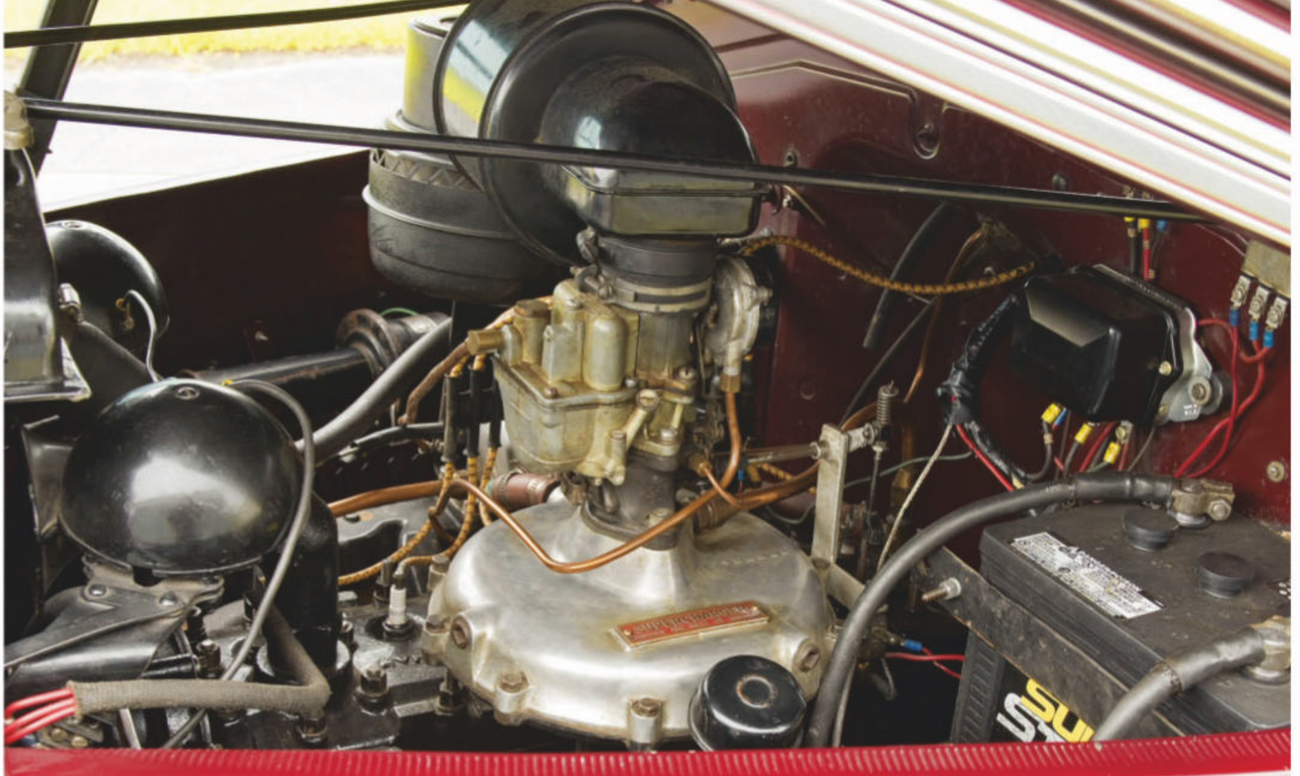
The 120-hp six-cylinder flathead has the optional supercharger featuring a 7.5-inch-diameter rotor that spins at 5.75-times engine rpm.
