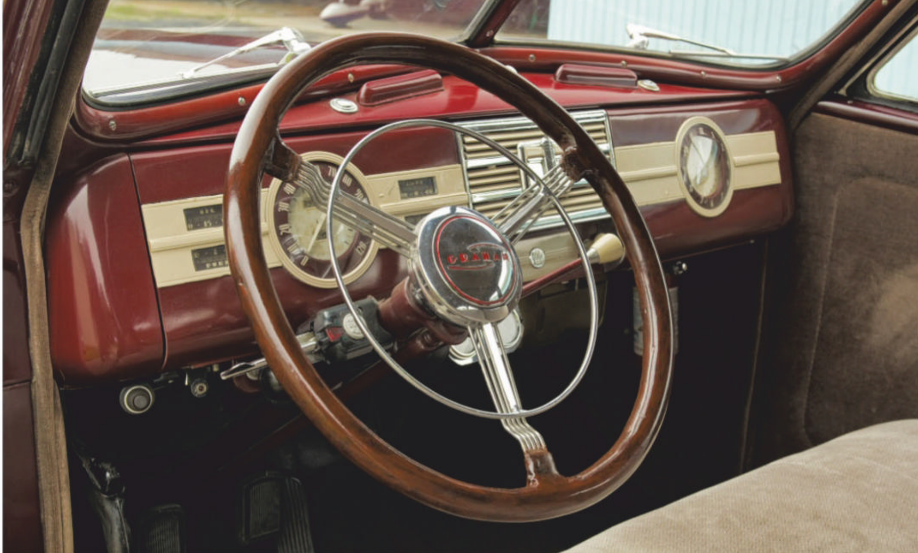
The chrome-spoke steering wheel was restored. A Graham heater was added by the owner, and the interior was reupholstered. A three-speed manual transmission was standard, and this Graham has optional overdrive.
