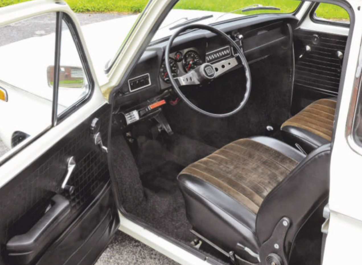
A drilled two-spoke steering wheel and large analog instruments, including an electronic tachometer, were standard 1200 TT fare, as were grippy corduroy seat inserts. This model's checkered-flag motif, seen on the front and rear emblems, was repeated on a central dash-mounted radio blanking plate.
