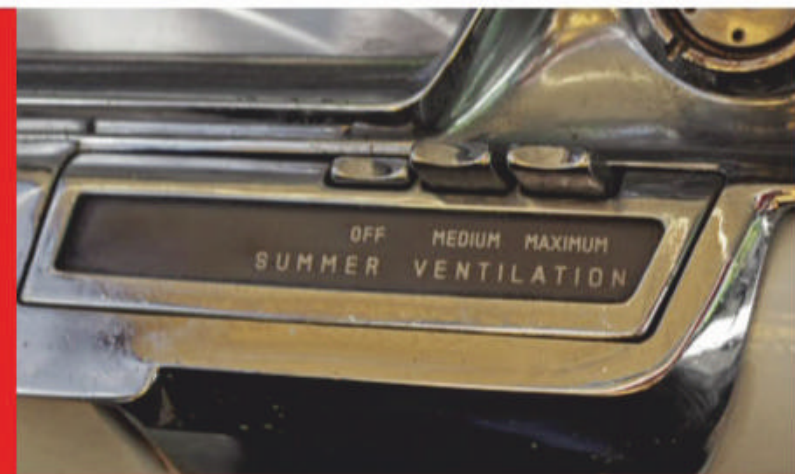
Black leather covers protect faded original seat upholstery. This car’s leaking heater core was bypassed years ago, but its ventilation fan controls still offer cooling breezes. Four generations of Szareks (and counting) have sat behind this wheel.
