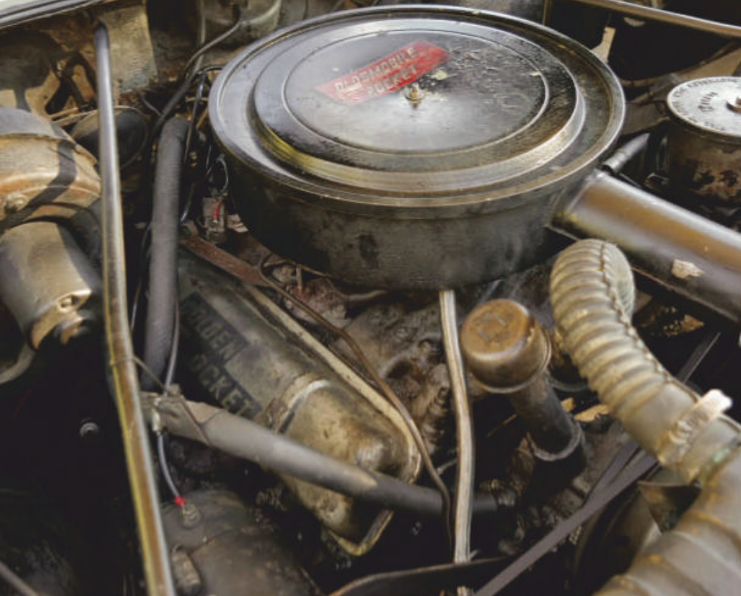
This 371-cu.in. V-8 has covered 60,000 miles in the last 61 years; its two-barrel carb was recently rebuilt. Having left the factory unencumbered, the V-8 has driven a power steering pump since 1962.
