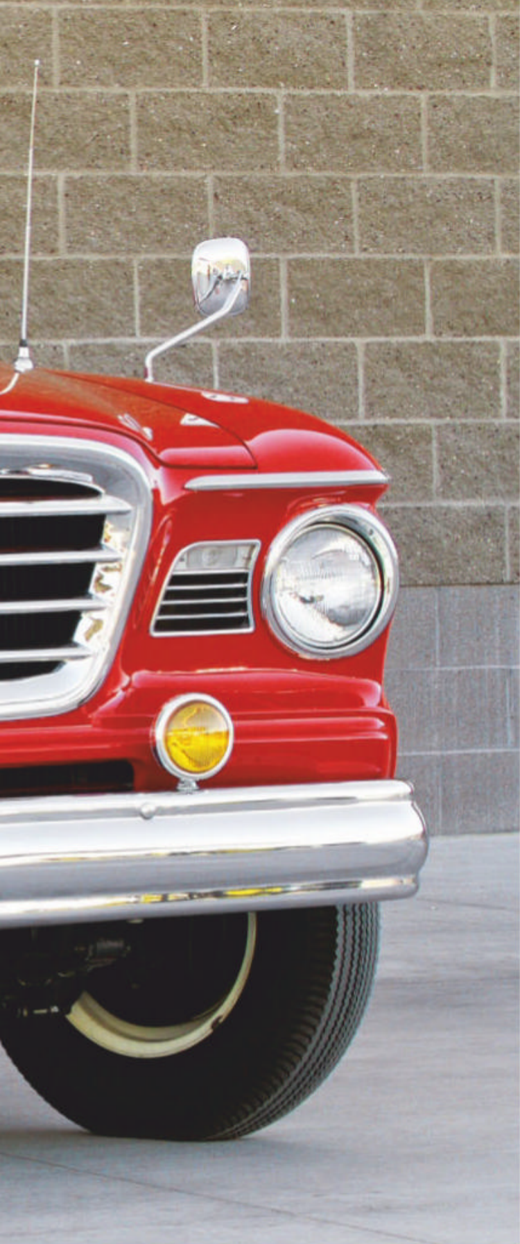
The Studebaker Lark sedan lent the Champ its cab as well as its dash. The truck used a chunkier grille and a sturdier front bumper that was mounted lower than the Lark's.
