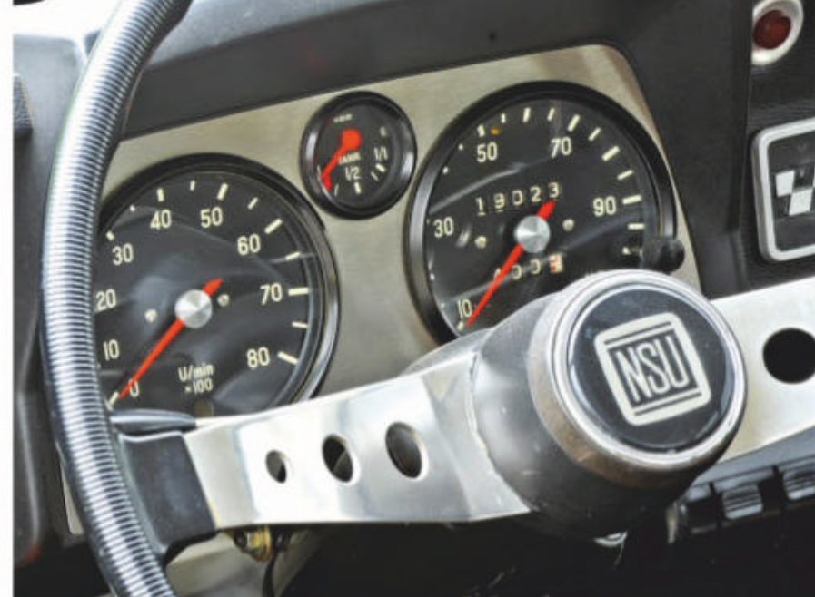
A drilled two-spoke steering wheel and large analog instruments, including an electronic tachometer, were standard 1200 TT fare, as were grippy corduroy seat inserts. This model's checkered-flag motif, seen on the front and rear emblems, was repeated on a central dash-mounted radio blanking plate.
