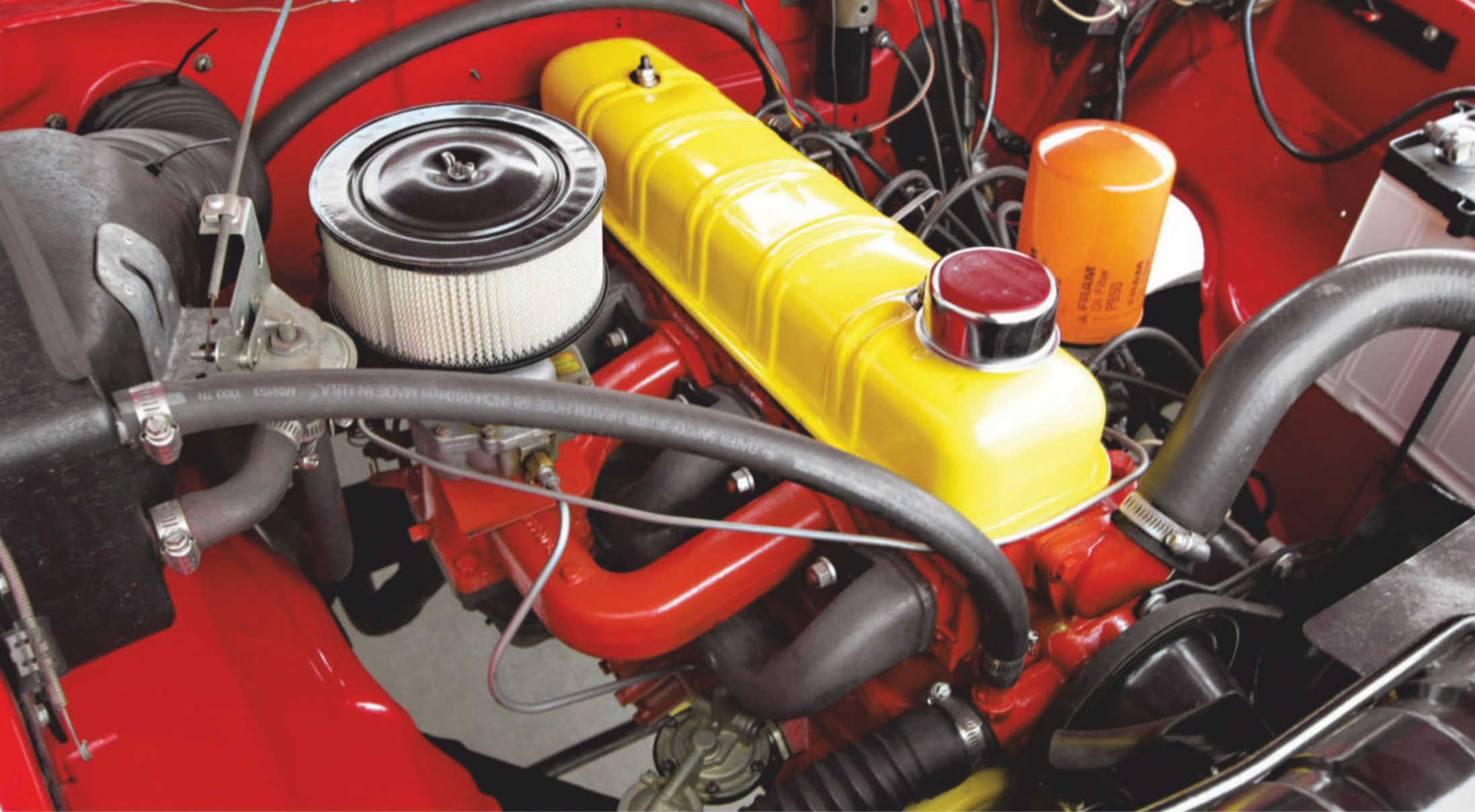
For 1961, the Champ's 170-cu.in. straight-six engine was upgraded to overhead valves. A new slab-sided bed, sourced from Dodge, didn't quite match the lines of the cab.
