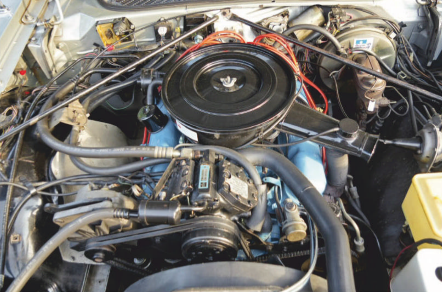
This 318-cu.in. V-8 remains equipped with all the emissions gear in place as installed in the factory in 1975, and as the current owner insists on preserving it.
