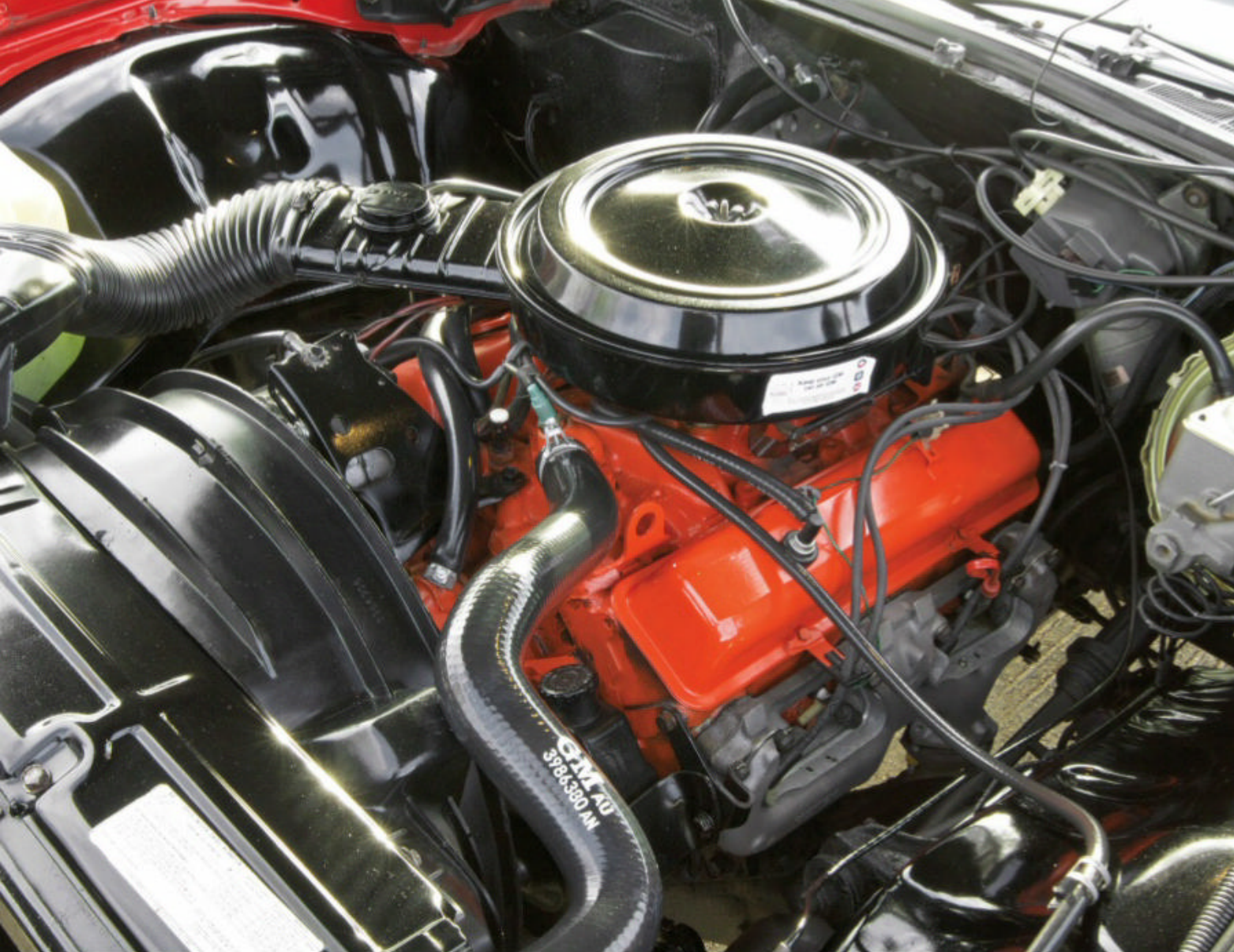
The 400 cubic-inch V-8 was Chevrolet's middle engine option for the fullsize cars in 1975; a two-barrel 350 was standard, and a four-barrel 454 was also available.
