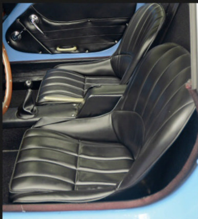
The fixed bulkhead behind the bucket seats limited their adjustability for taller drivers, a compromise forced by the engine placement. The spare wheel, battery, fuel tank, and fluid reservoirs sat under the side-hinged front hood.
