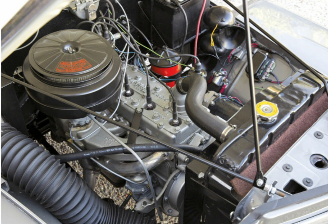
Featuring a Carter YF one-barrel carb and four main bearings, the 226.2-cu.in. "Super Hurricane" L-head straight-six engine produces 105 hp and 190 lb-ft of torque.
