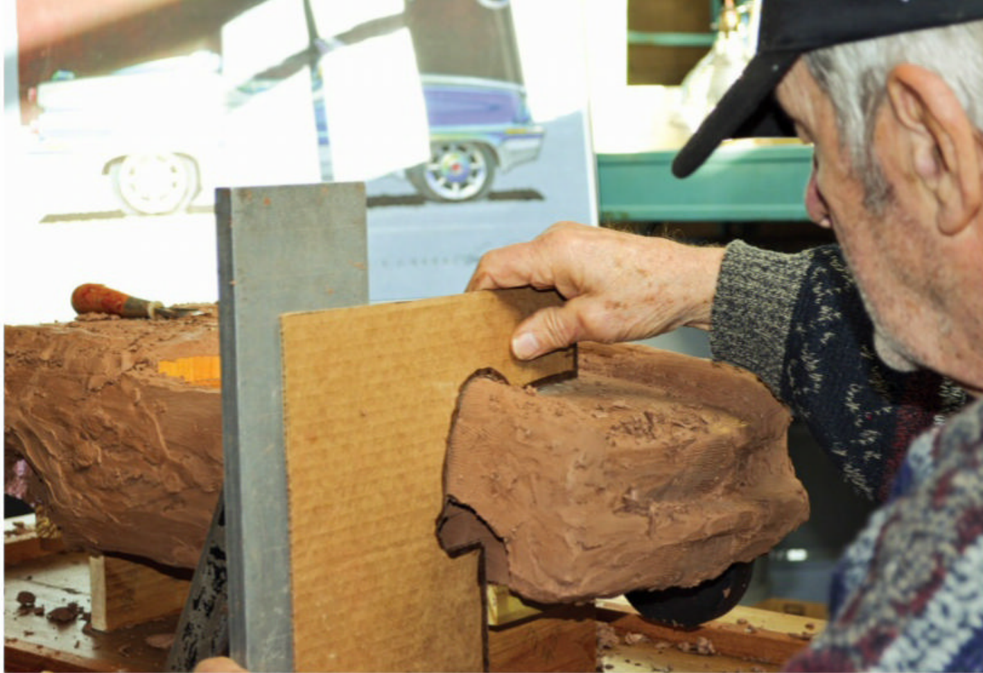
Keith Goodnough uses a handmade fixture to check the body curves.
