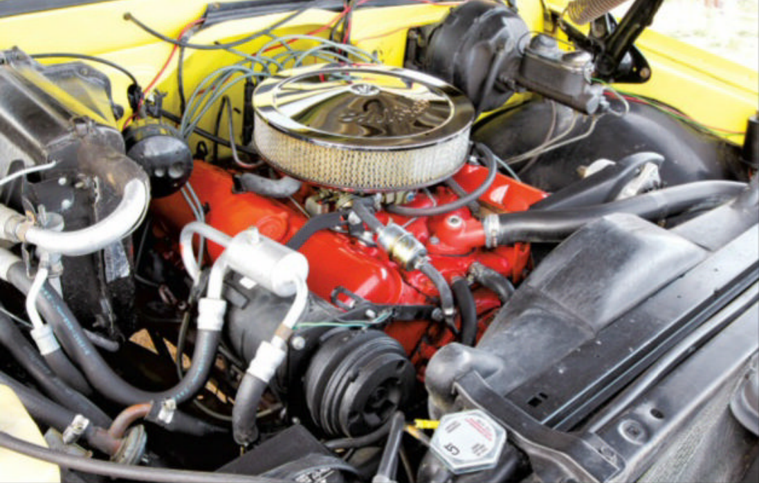
A 402-cubic-inch Chevrolet big-block V-8 moves this Longhorn, empty or loaded, with power to spare for air conditioning. An open-element air cleaner resides in place of the restrictive original. Inside, the CST package adds upholstery with simulated leather tooling, carpeting, bright pedal trim, door-operated dome lamp switches and more.
