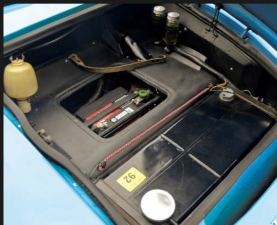
The fixed bulkhead behind the bucket seats limited their adjustability for taller drivers, a compromise forced by the engine placement. The spare wheel, battery, fuel tank, and fluid reservoirs sat under the side-hinged front hood.
