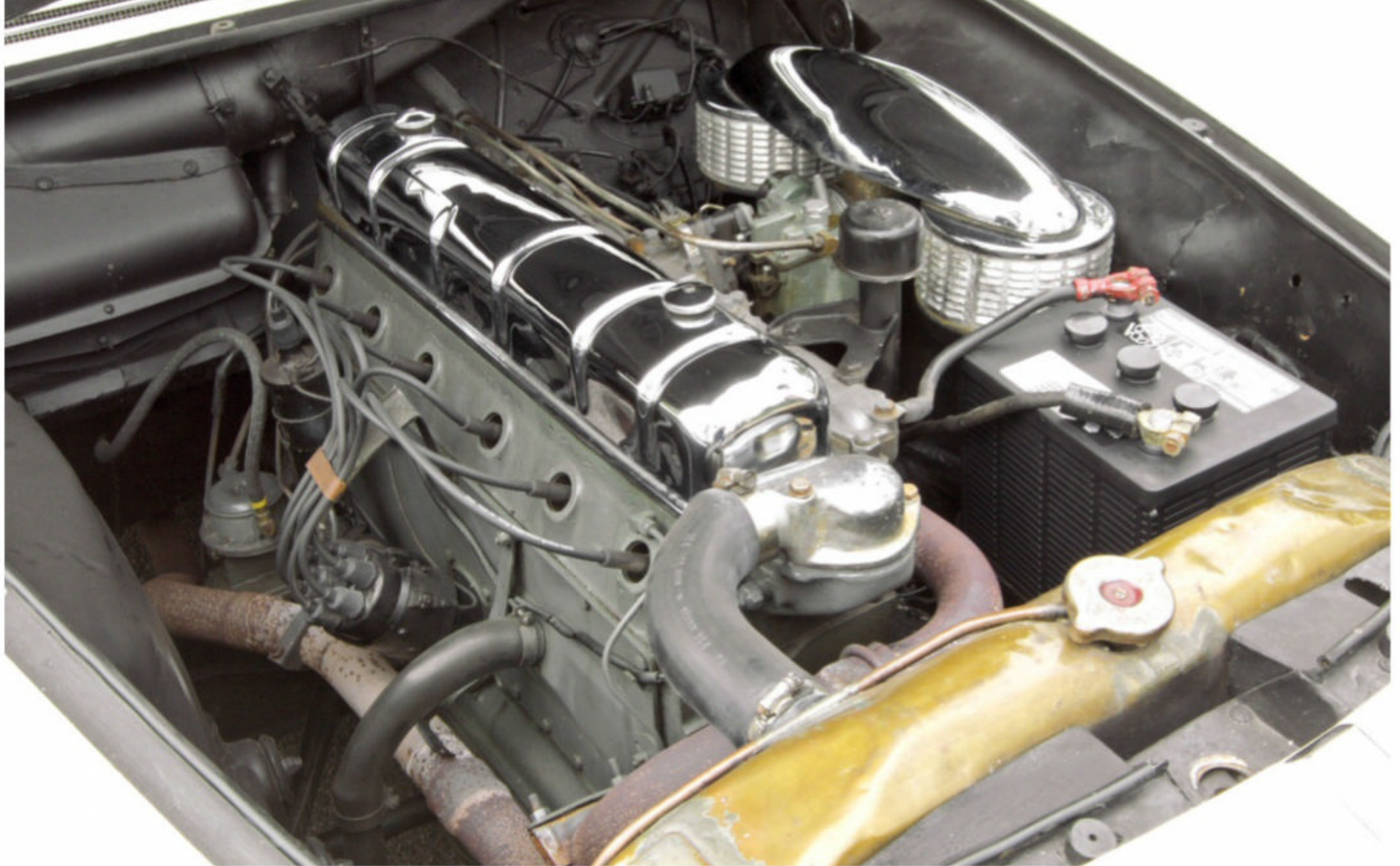
This one-off show car was built to be completely functional, and uses Nash's one-barrel-carbureted 262.6-cu.in. "Jetfire" straight-six in 130-hp tune. The OHV six sends its power to the rear wheels through a three-speed manual and torque tube drive.
