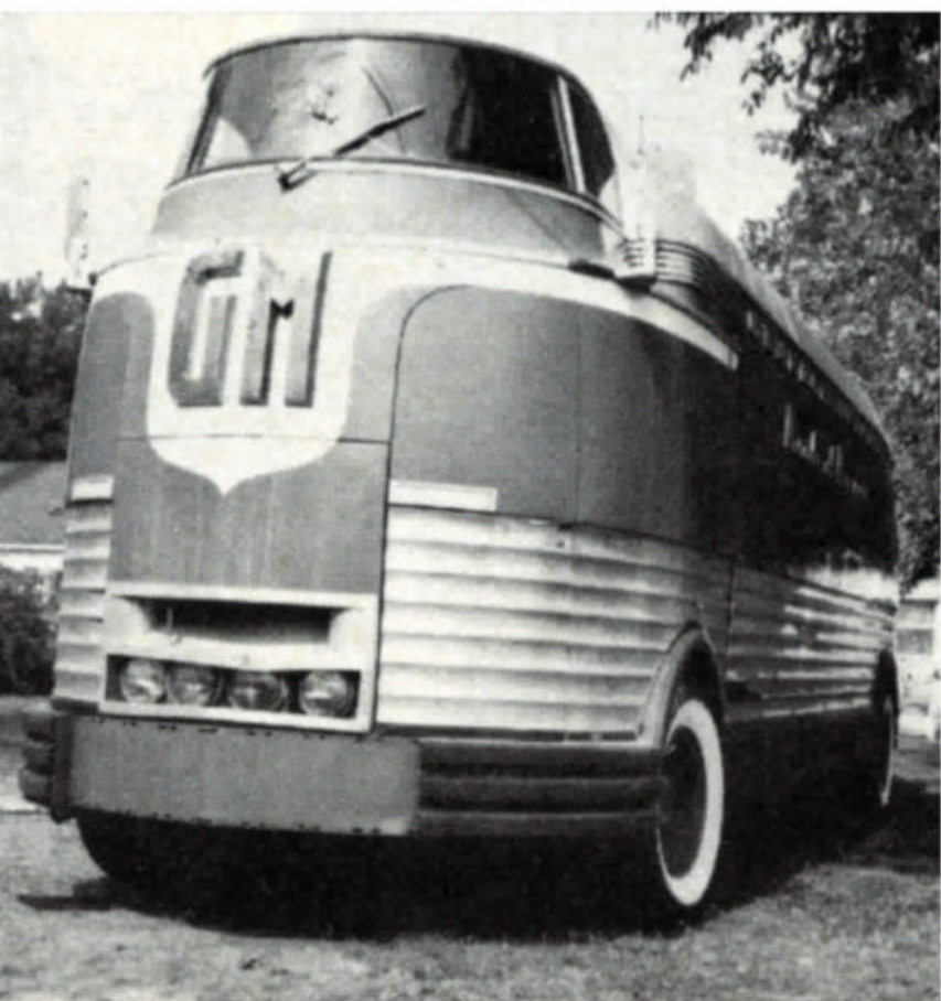
Entertainer Vic Hyde of Niles, Michigan, owns [March 1977] one of seven Parade streamliners known to survive. Stairway leads to glassed-in cockpit, which seats driver in front center and two more people on the bench behind. Lighting pod can be raised from rear roof section.
