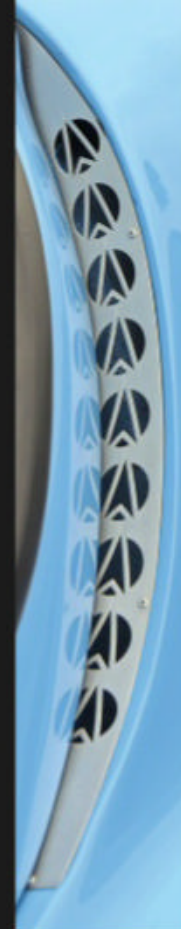
This Matra Bonnet D'Jet V sports a rare lift-off sunroof. The 70 hp from its mid-mounted Renault engine could push the light, aerodynamic car over 100 mph. Stamped aluminum C-pillar vents sported a pattern of Matra emblems.
