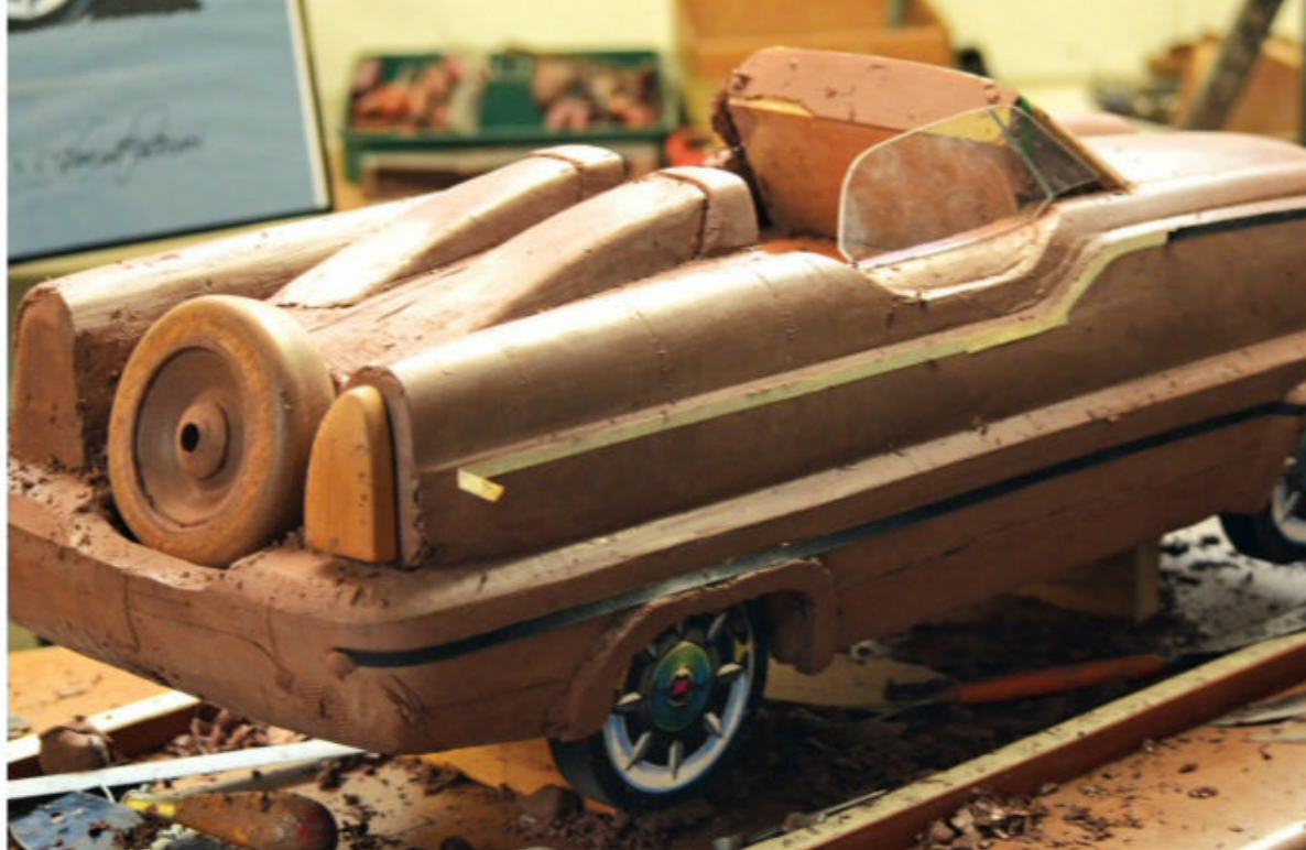
In this rear \frac{3}{4} view, you can see the small hand-carved wooden shape used as bases for the windshield and taillamps.
