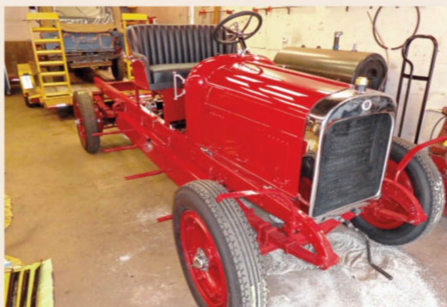
Final assembly is underway, with the engine, transmission, and pump installed, along with the completed suspension and brake systems. New wiring was also installed. Note that several pieces of trim are in place, finished in chrome versus nickel.
