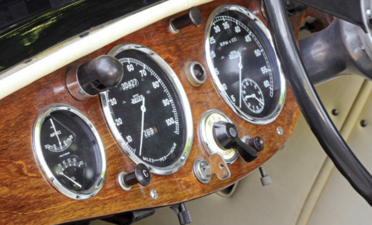
In the traditional British solid wood instrument panel, the Jaeger speedometer and tachometer are flanked by ammeter, oil pressure, and fuel gauges.
