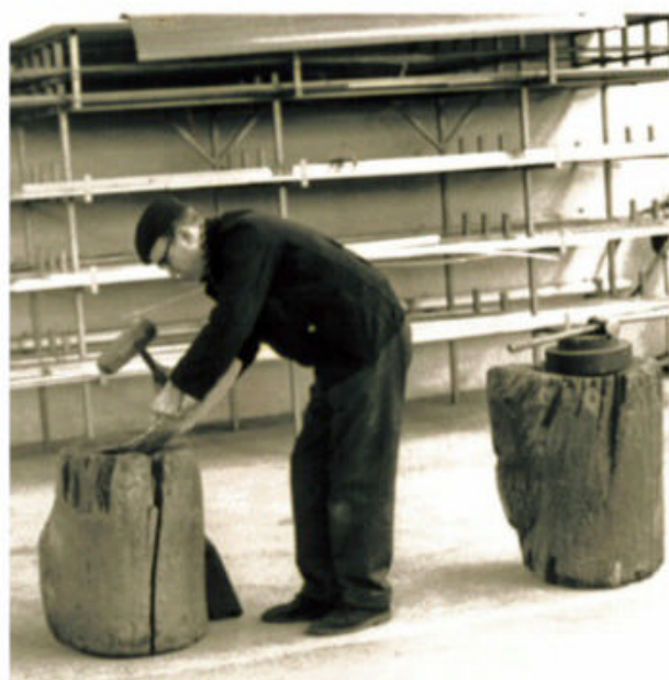
After the public's rousing reaction to the AMX concept, it was decided to build an actual running version of the car. The job was handled by the Italian coachbuilder Vignale. Shown here is one of Vignale's craftsmen hand hammering a sheet of metal using a stump.
