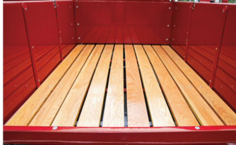
New oak decking graces the hose bed. Hidden below is an extra two-shelf compartment just deep enough for extra firefighting tools.
