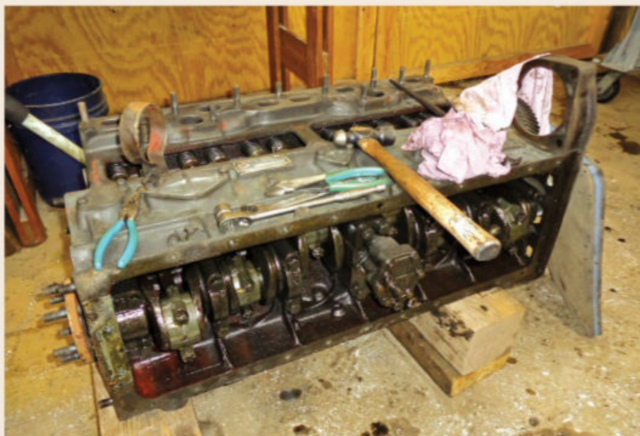
Seagrave utilized a Continental six-cylinder engine in its Suburbanite line, and, although this unit is from the 1932 model year, its architecture is similar to the original engine. Close inspection determined that the engine did not require rebuilding.
