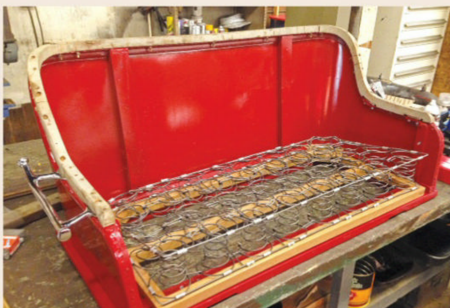
The Seagrave's seat during its restoration. The springs have been reconditioned and mounted to a new wooden base frame. Matching the factory build traits, horse hair will fill the void before new leather upholstery completes this subassembly.
