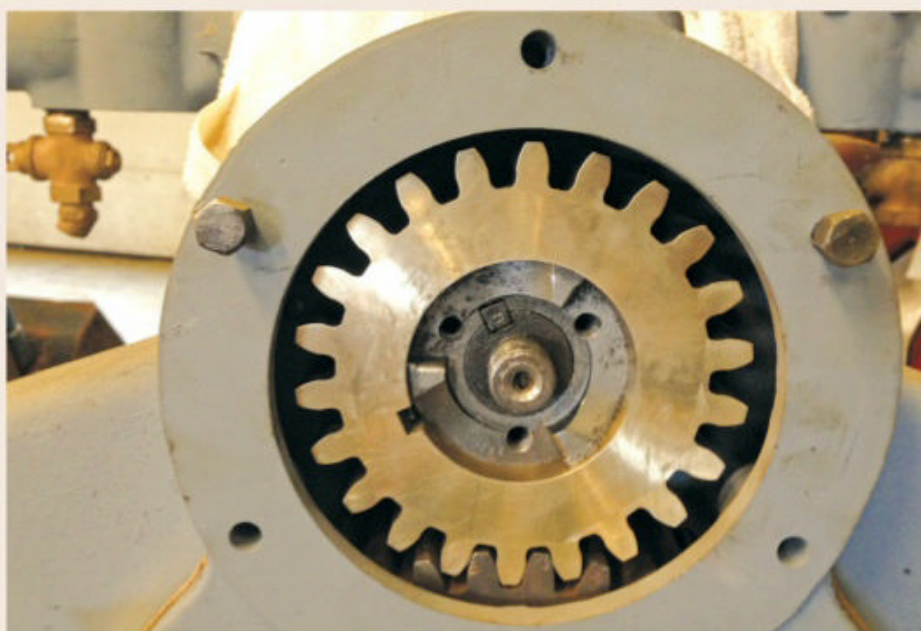
Here the new water pump drive gear is installed. The straight-tooth cog was custom-fabricated from bronze. Like the original gear, this is a sacrificial part designed to take a load yet fail under catastrophic duress to prevent damage elsewhere within.
