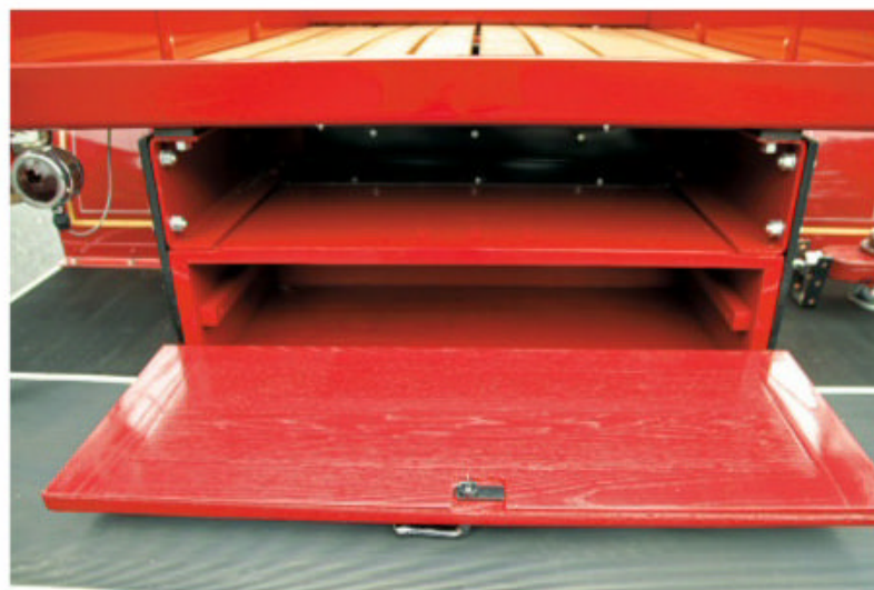
New oak decking graces the hose bed. Hidden below is an extra two-shelf compartment just deep enough for extra firefighting tools.
