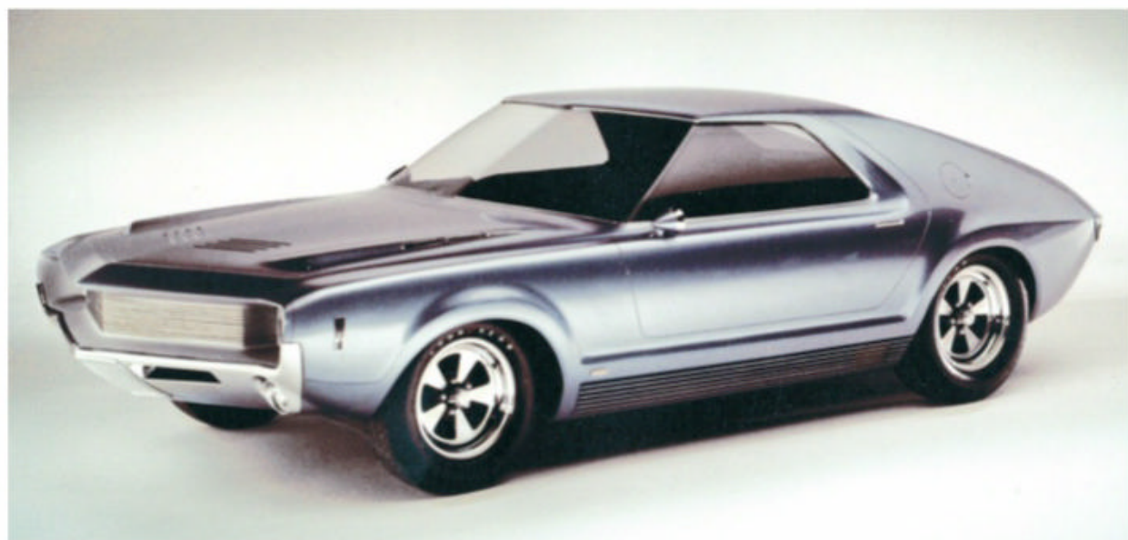
The original AMX concept, built as a non-running fiberglass "pushmobile." The cantilever roof and cockpit-style doors were both popular features, but were impractical for production.
