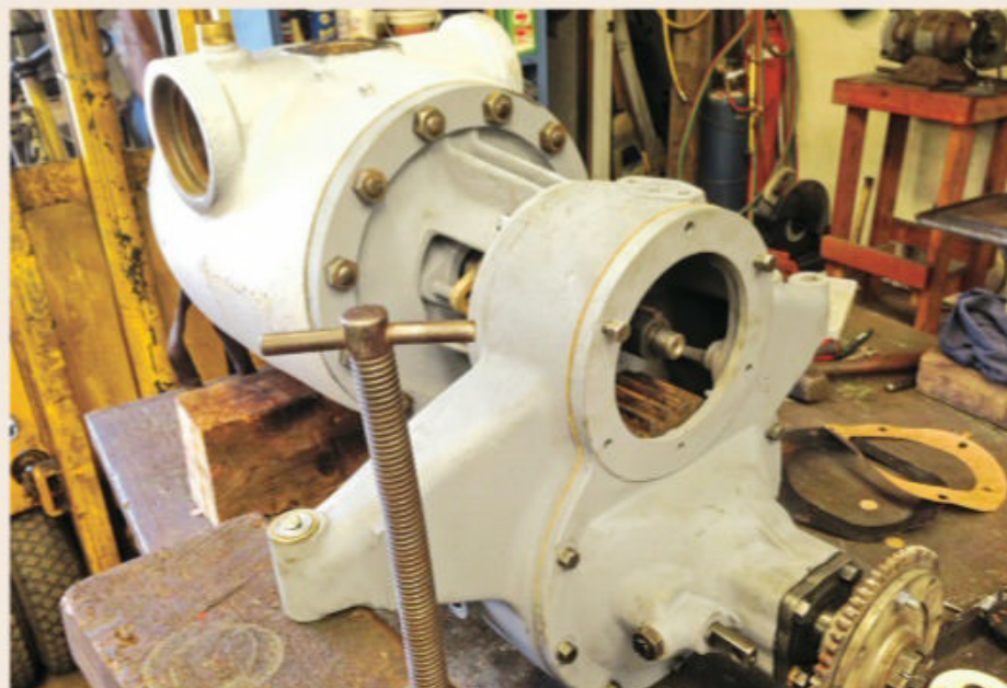
This is the Seagrave-designed, single-lever 500-gpm water pump cleaned and under inspection on a work bench. New seals and bearings helped rebuild the unit; however, it also required a new drive gear after the original was found in pieces.
