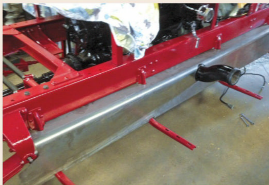
One of only three exterior metal parts that needed to be fabricated was the right-side splash apron. The damaged original was used as a pattern, and the replacement was test-fit multiple times—as seen here—prior to receiving primer and paint.
