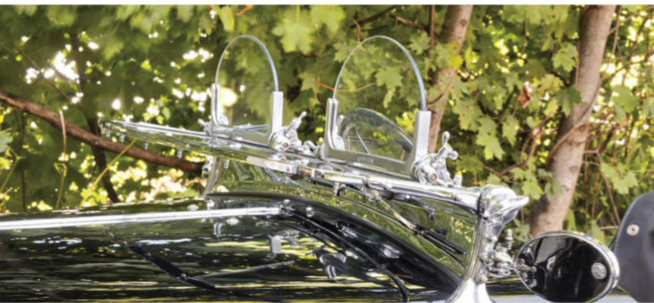
The fashionable pair of Brooklands racing-style aeroscreens help deflect the oncoming wind when the windshield is folded down; they adjust to any angle.
