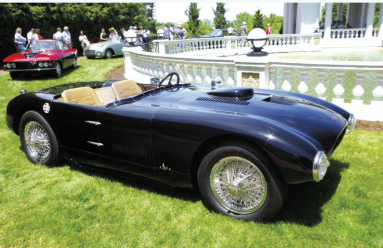
With a 331-cu.in. Cadillac V-8 under its louvered and blistered bonnet, this 1953 Allard JR roadster is one of seven built, and was shown by owner James Taylor.
