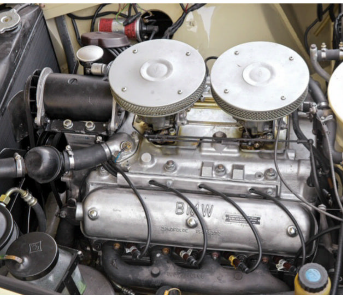
The 140-hp BMW V-8 shared a general concept with American V-8s, but displaced just 3.2 liters and was of aluminum-alloy construction.
