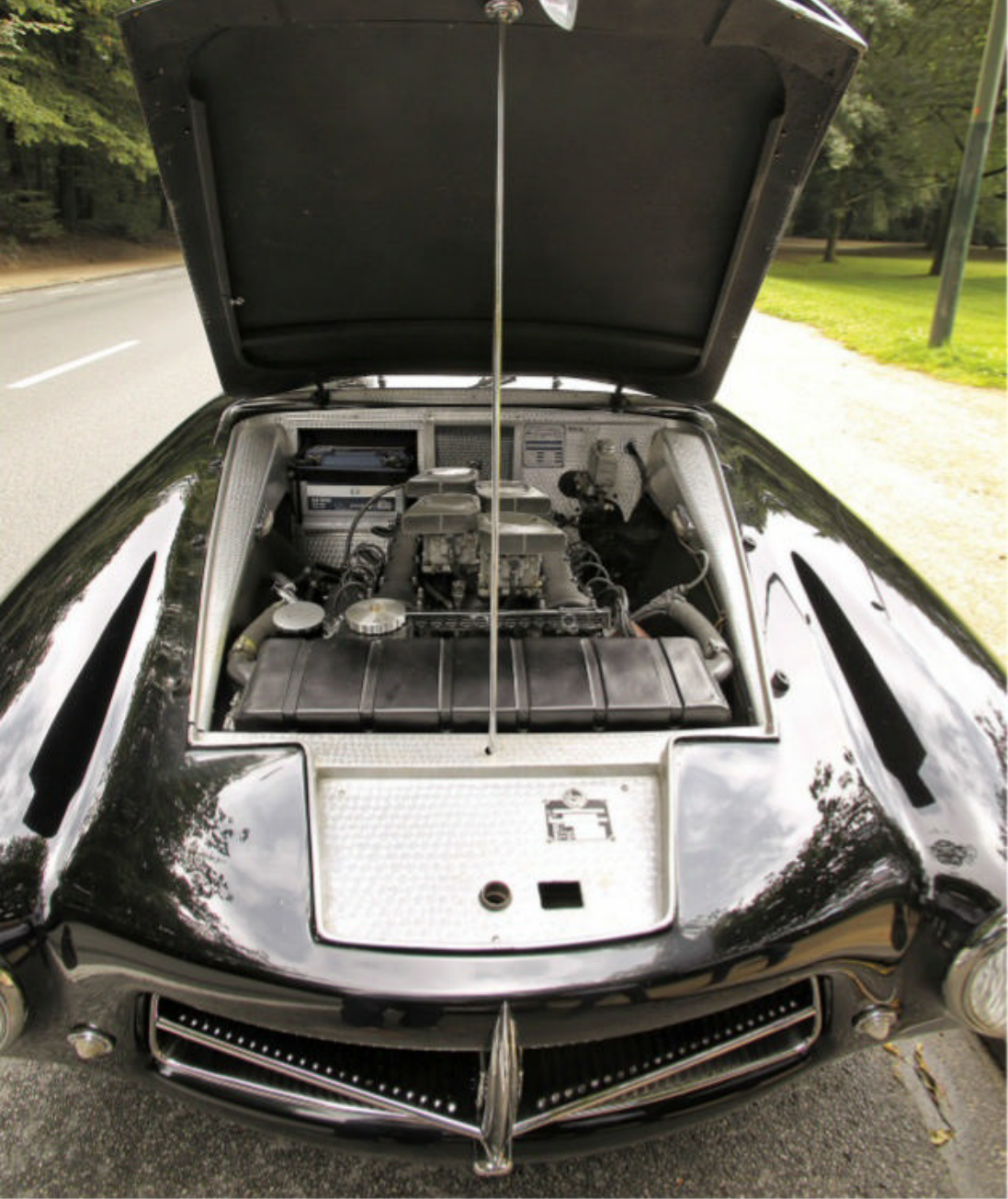
The 2.8-liter quad-cam V-8 engine powering the Pegaso Thrill owes much to former Alfa Romeo engineer Wilfredo Ricart's previous experience in European racing; this example sports four Weber DCF carburetors, while some other Z-102s were fitted with a supercharger.
