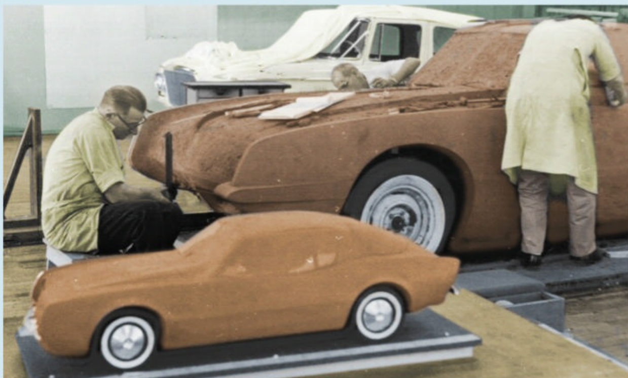
Among the ideals chased by Loewy's designers was Jaguar's own timeless icon, the E-Type. After the Loewy team created a quarter-scale model, a full-scale clay mockup was created for executive review in Studebaker headquarters in South Bend.
