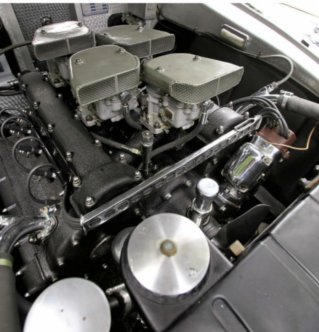
The 2.8-liter quad-cam V-8 engine powering the Pegaso Thrill owes much to former Alfa Romeo engineer Wilfredo Ricart's previous experience in European racing; this example sports four Weber DCF carburetors, while some other Z-102s were fitted with a supercharger.
