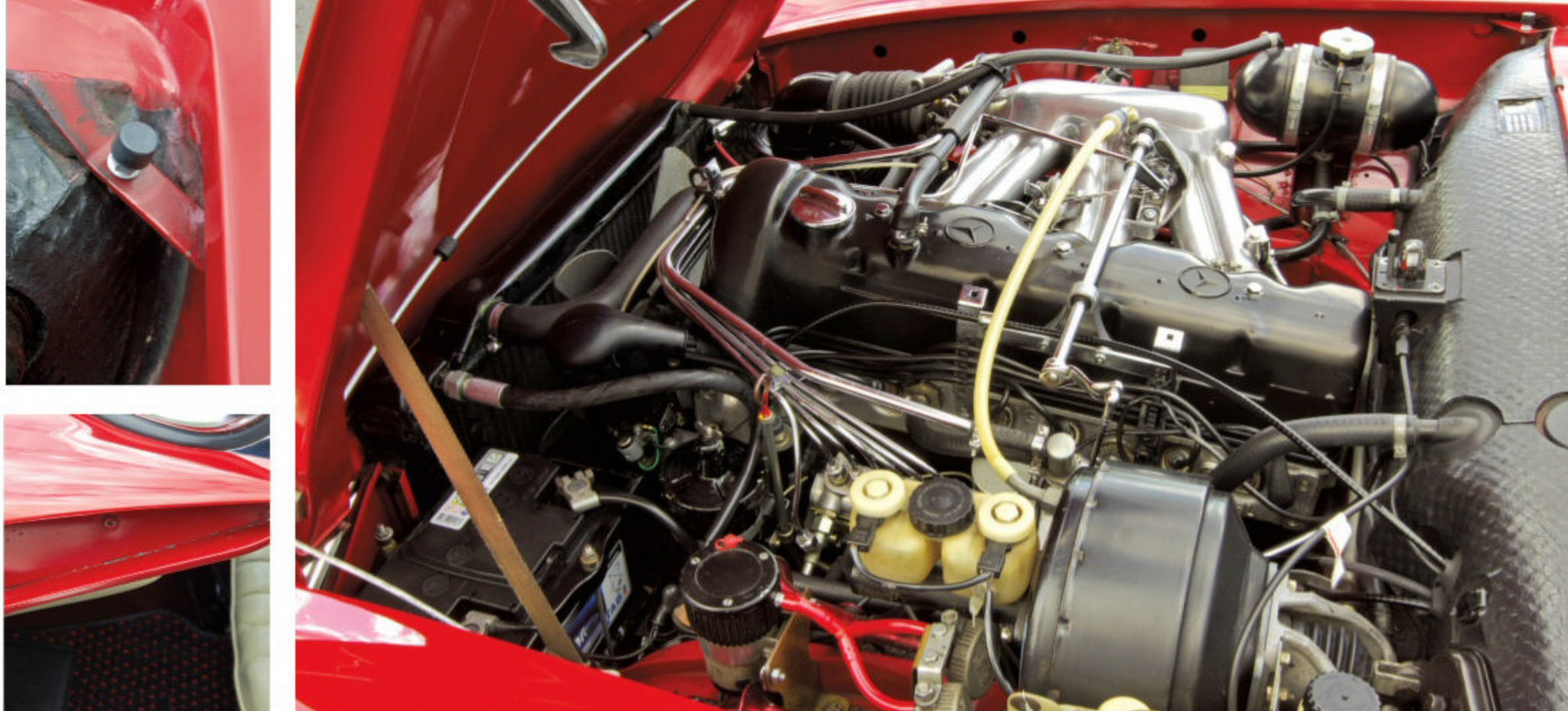
Carefully finished jambs hide factory spot welds; painted, polished, and chromed engine components show this car was built for display.
