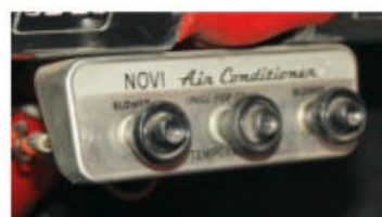
Packard originated automobile air conditioning before World War II, so its presence here seems only natural. Like other systems of the era, the Novi air conditioner occupied a portion of the trunk and fed cool air to passengers via clear ducts on the package shelf.
