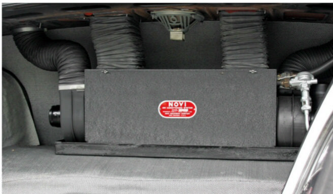
Packard originated automobile air conditioning before World War II, so its presence here seems only natural. Like other systems of the era, the Novi air conditioner occupied a portion of the trunk and fed cool air to passengers via clear ducts on the package shelf.
