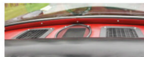
Packard originated automobile air conditioning before World War II, so its presence here seems only natural. Like other systems of the era, the Novi air conditioner occupied a portion of the trunk and fed cool air to passengers via clear ducts on the package shelf.
