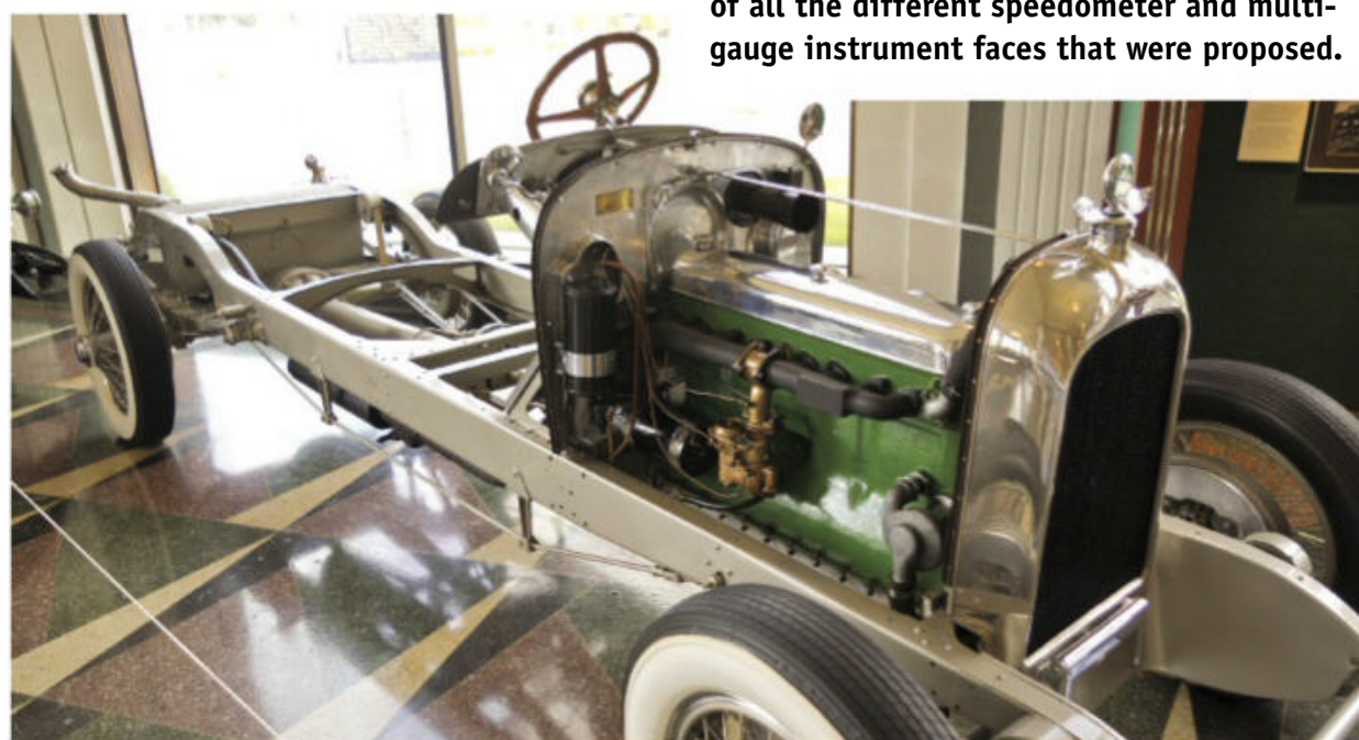
Body-less chassis is that of a 1926 Duesenberg Model A, featuring a 90-hp, 260-cu.in. overhead-cam straight-eight. Engine (left) is a 12-cylinder Duesenberg-built Bugatti engine with twin upright cylinder heads.
