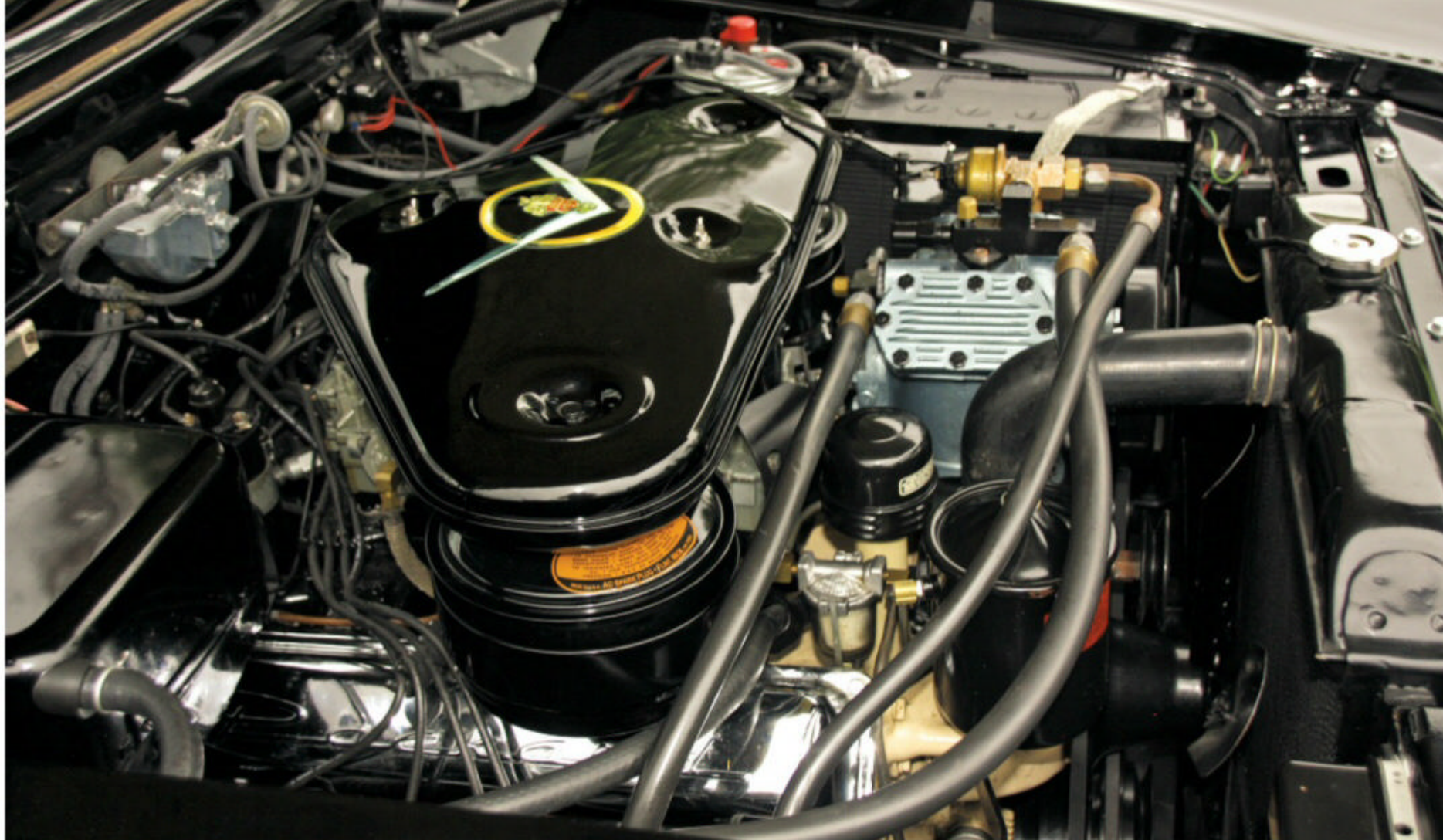
The dual-quad, 275-hp, 352-cu.in. V-8 was standard on Caribbean convertibles and optional on other senior Packards. The original buyer of this car spared no expense when fitting it out and thus opted for the most-powerful engine as well. Note the “batwing” air cleaner.
