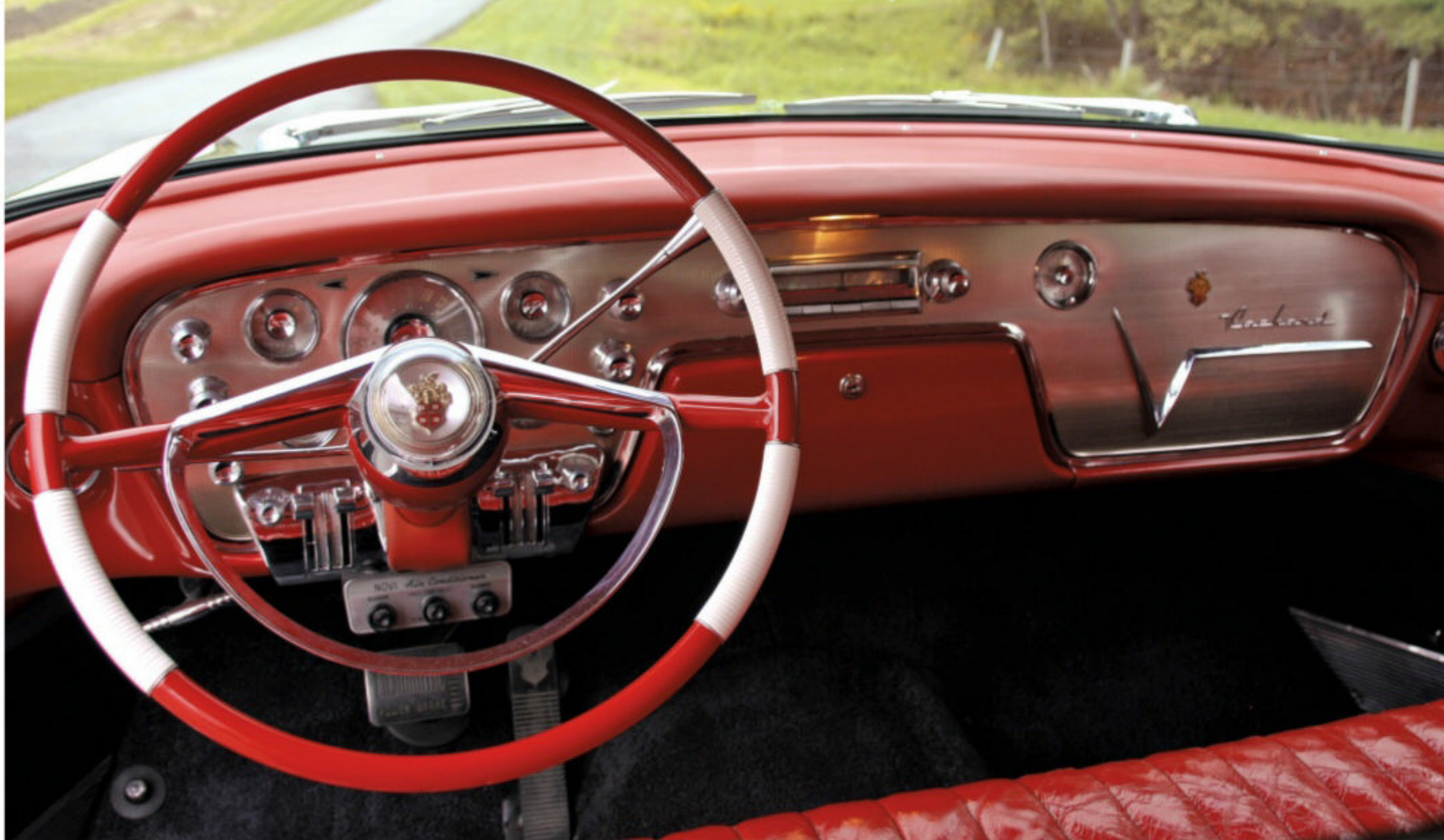
Brushed stainless and red make for a handsome, modern (for 1955) combination on the dash of the Four Hundred. Note that gear selection is made via a lever—pushbuttons would be an option the next year. Novi air conditioning controls are located below the steering column.
