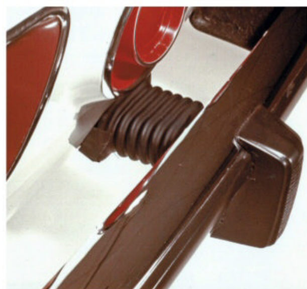
Nixon's unique "freestanding bumpers" used a flexible rubber form to dress-up the bumper brackets.
