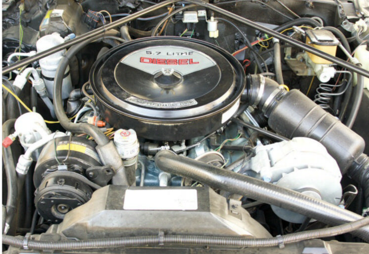
The only passenger car diesel V-8 on earth in 1980 was the Oldsmobile-built LF9-code. The 120 hp, 220 lb-ft V-8 was standard in Seville in 1980
