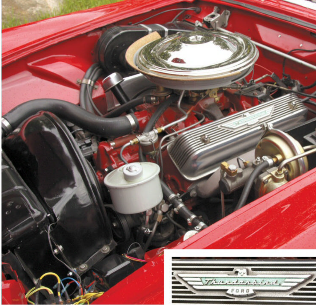
The floor shifter controls Ford's revised-for-1955 Fordomatic, which now started in first gear rather than second gear. The 198-horsepower V-8 was standard with the automatic transmission.
