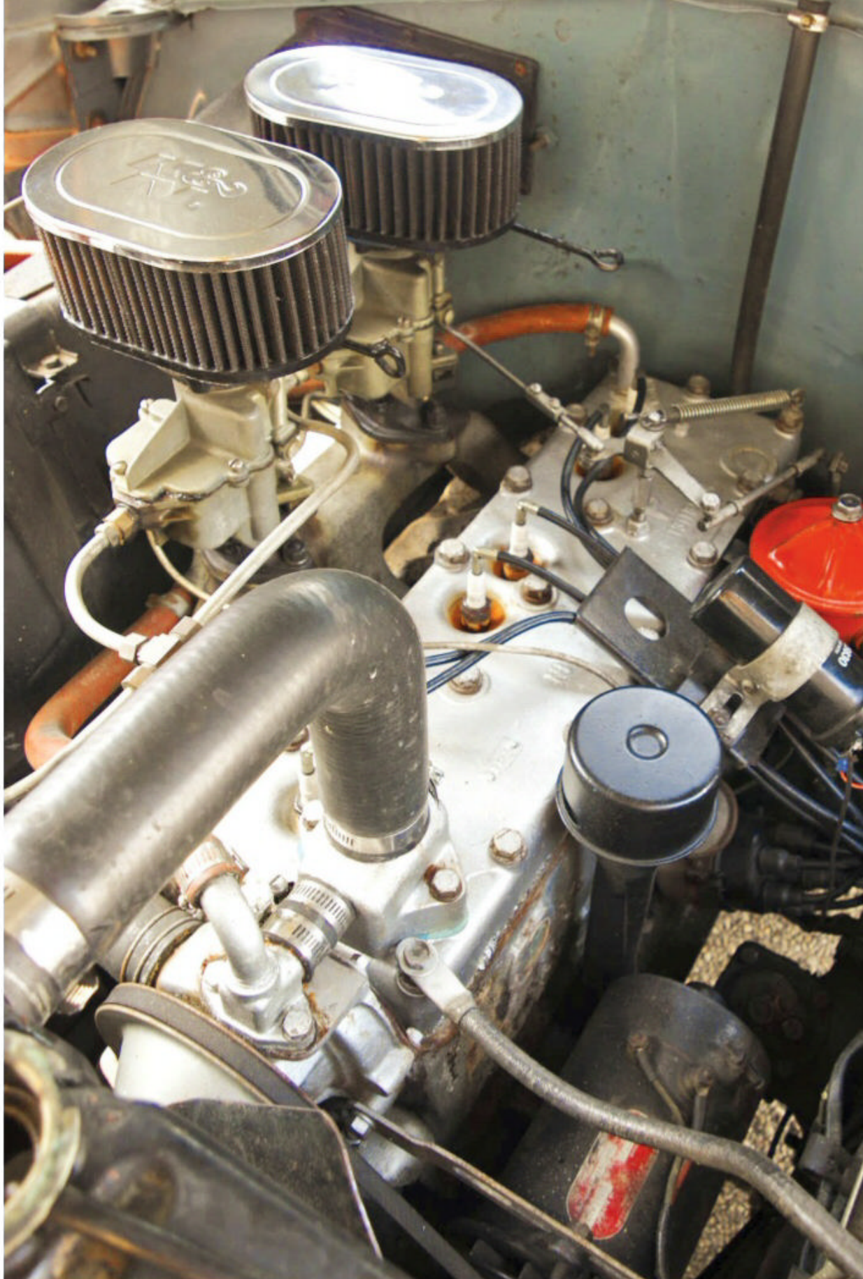
The original 97-hp, 218-cu.in. flathead six-cylinder was replaced with a 230-cu.in. six from a 1958 Dodge equipped with aftermarket speed parts—intake manifold, camshaft, and header.
