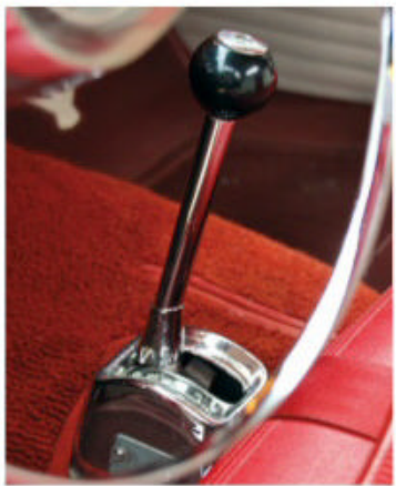
The floor shifter controls Ford's revised-for-1955 Fordomatic, which now started in first gear rather than second gear. The 198-horsepower V-8 was standard with the automatic transmission.
