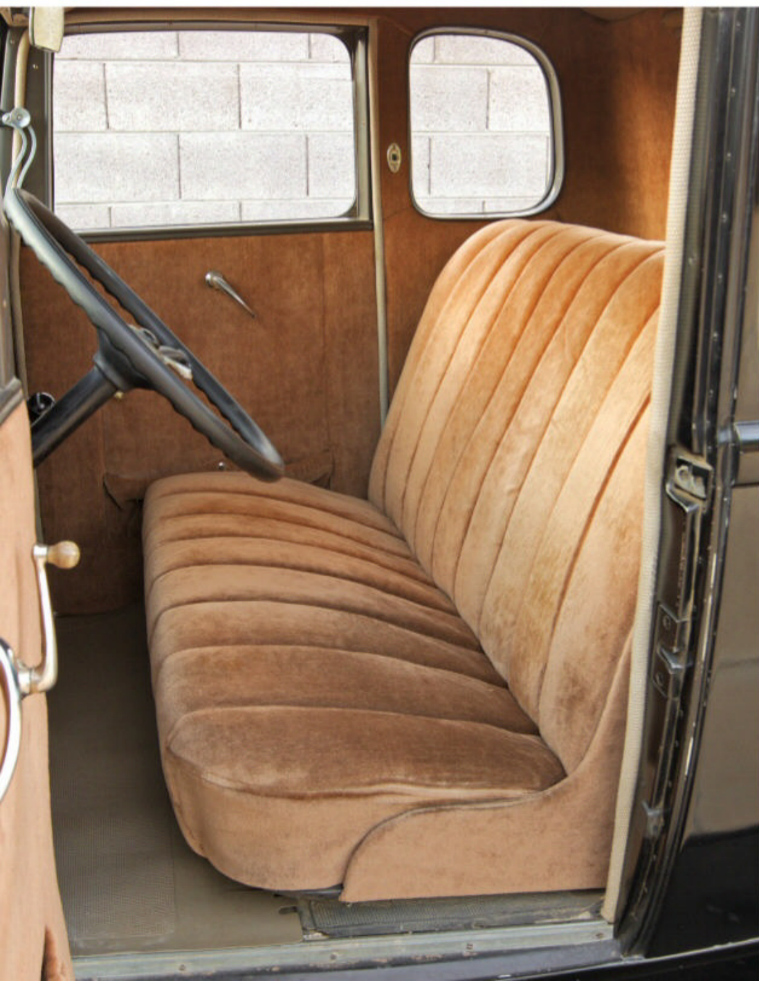
The original material worn threadbare decades ago; leftover Ford material was reused to reupholster the interior to factory specifications. Clearly read gauges live in a centrally located engine-turned panel. Eighty miles per hour seemed optimistic in the four-cylinder Model B.
