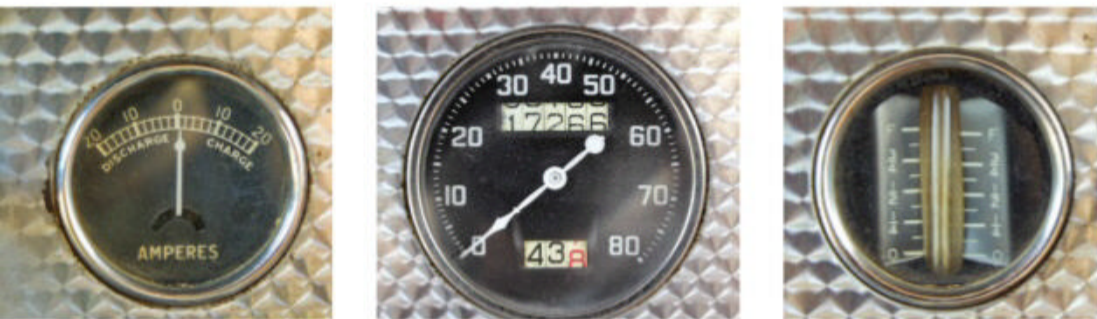
The original material worn threadbare decades ago; leftover Ford material was reused to reupholster the interior to factory specifications. Clearly read gauges live in a centrally located engine-turned panel. Eighty miles per hour seemed optimistic in the four-cylinder Model B.
