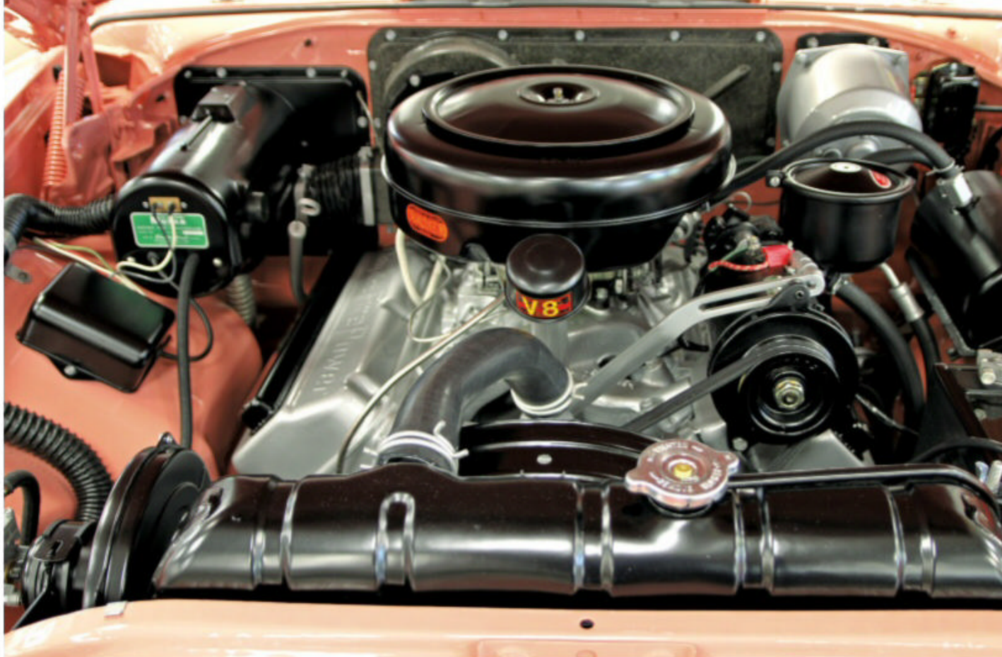
The original 354-cu.in. Hemi V-8 engine was rebuilt to factory specifications, save for a .020-inch overbore to smooth the cylinder walls and optimize engine longevity.
