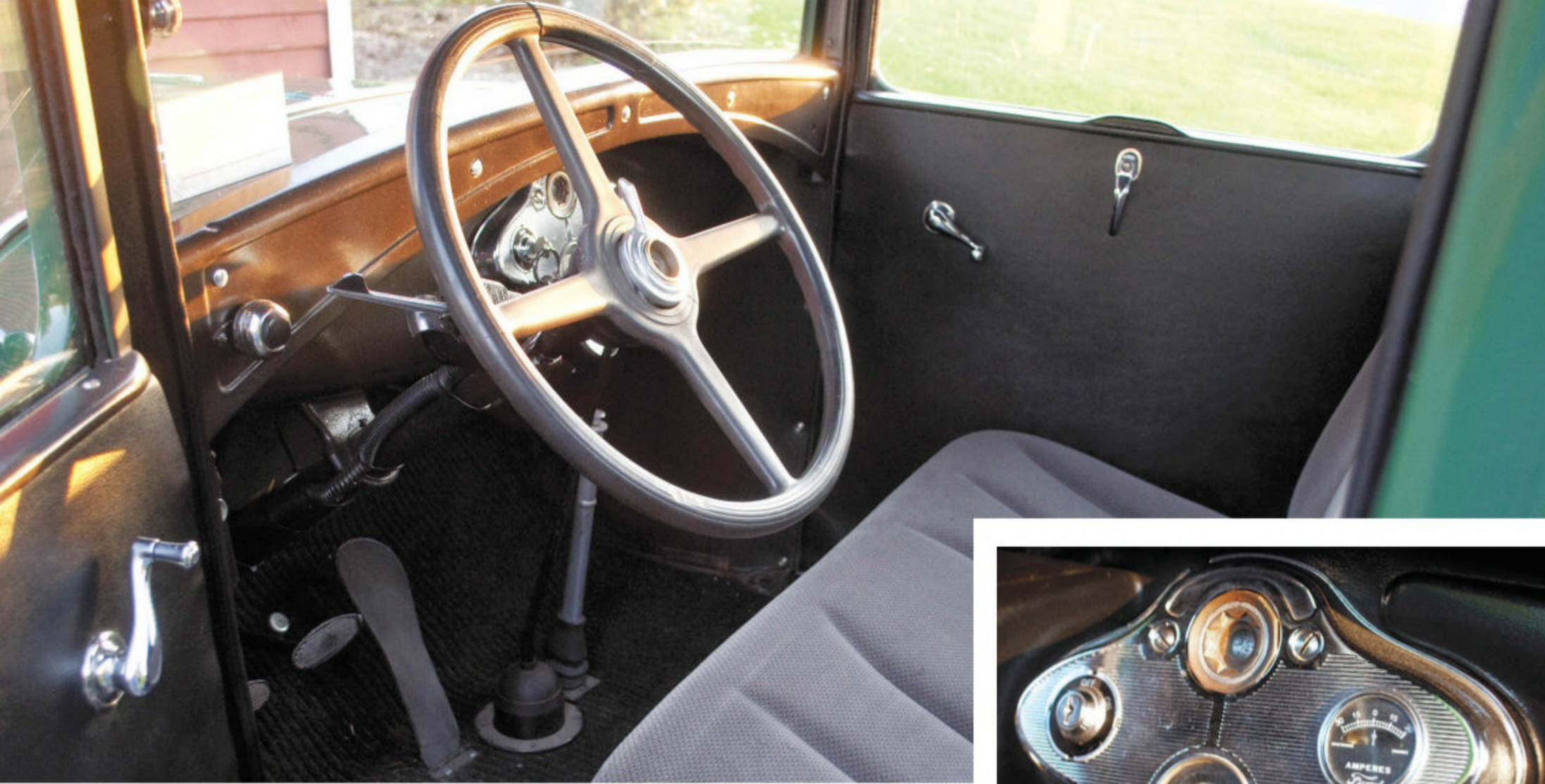
A mid-row seat from a Dodge Caravan stands in for the original bench and offers a little more driver comfort. The speedometer has been unofficially radar certified. Top speed? 45 mph.
