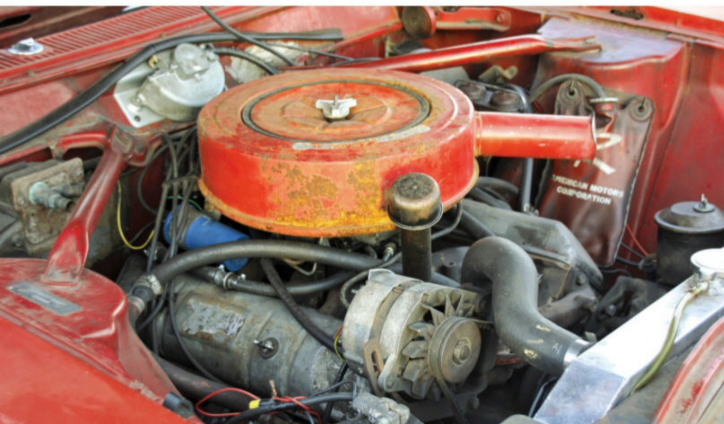
The four-barrel, 270-hp, 327-cu.in. engine is the first-generation AMC V-8, which dates back to 1956. After a year back on the road, it cried out for renewal and was rebuilt.
