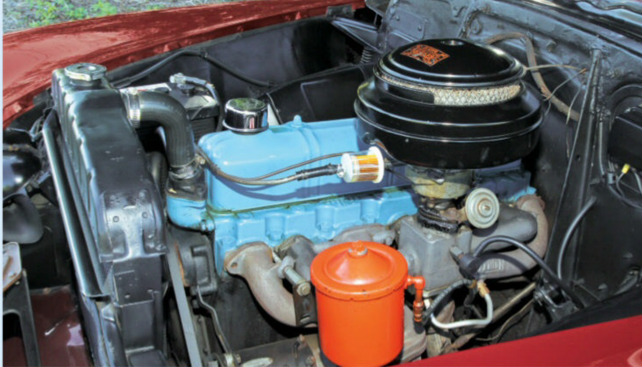
Ordering an automatic transmission also delivered a larger, more powerful engine for 1951. This Powerglide-equipped Styleline retains its original 105-hp 235.5-cu.in. straight-six.
