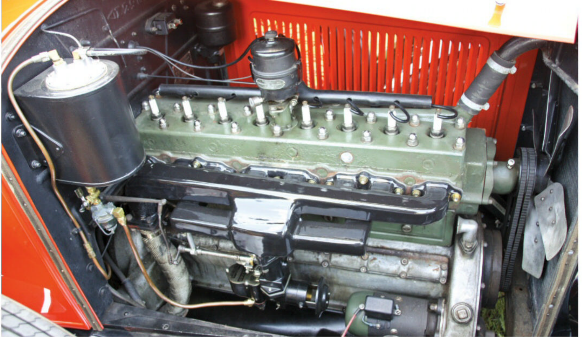
The Packard straight-eights of 1930, a 1924-vintage design, still featured a separate aluminum crankcase. Packard had discontinued straight-sixes after 1928, and the Twin Six (V-12) after 1923. The black canister on the firewall is a Stewart-Warner vacuum fuel pump.
