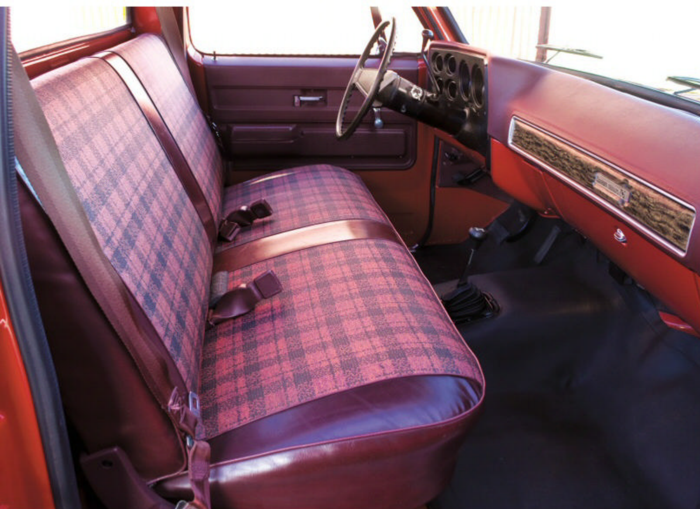
The interior still boasts its original plaid upholstery, which was standard issue on Custom Deluxe trucks. Four-wheel drives with automatics were equipped with a full-time transfer case, so the lever on the floor offered: High, Low, High Lock, and Low Lock.
