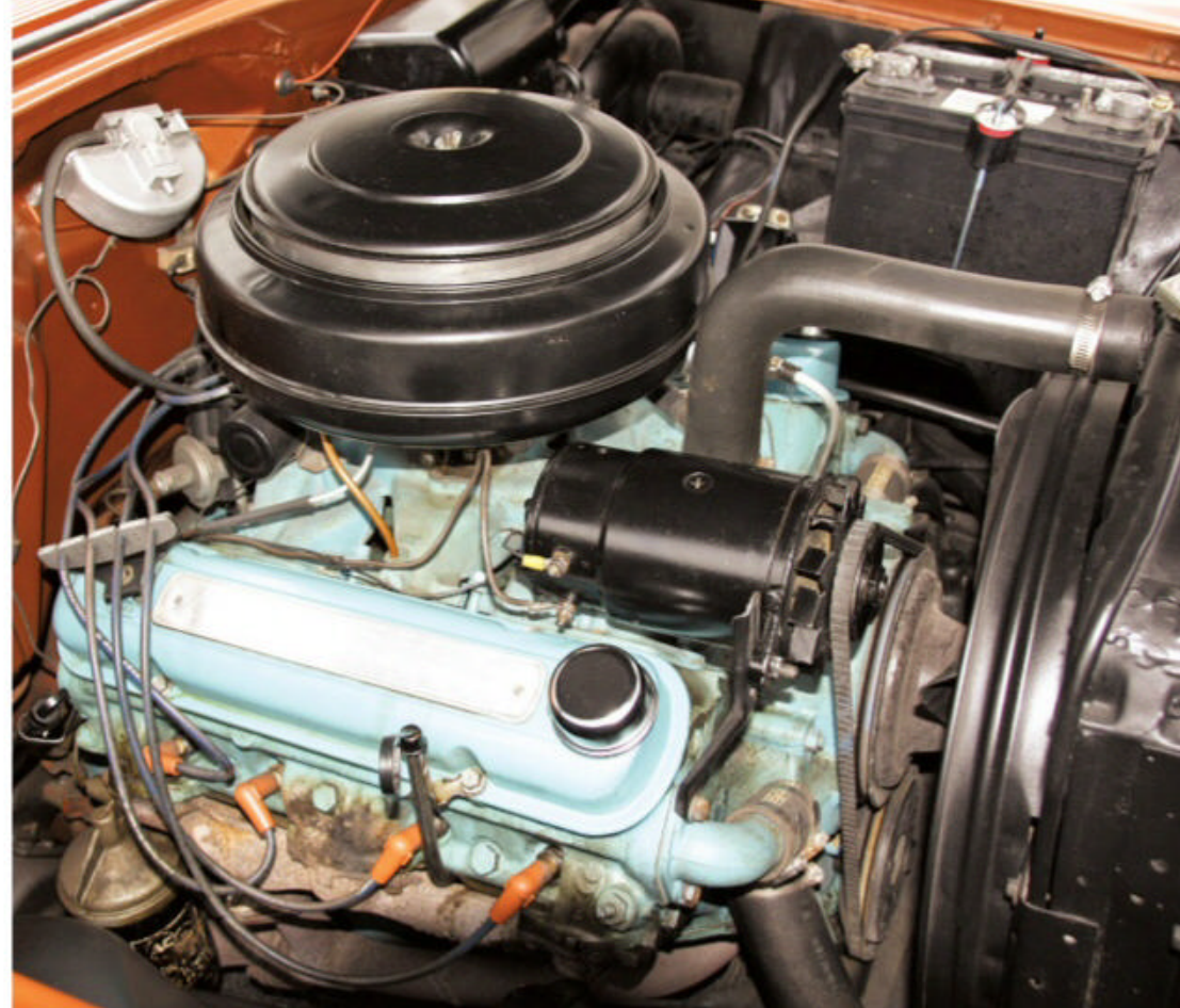
The Strato-Streak V-8 would form the basis for Pontiac V-8 engines through 1981, including the GTO's 389. Note the oil filter (below right) — something that wasn't standard equipment on Chevrolet until 1956 — and the large black fresh-air heater box on firewall.
