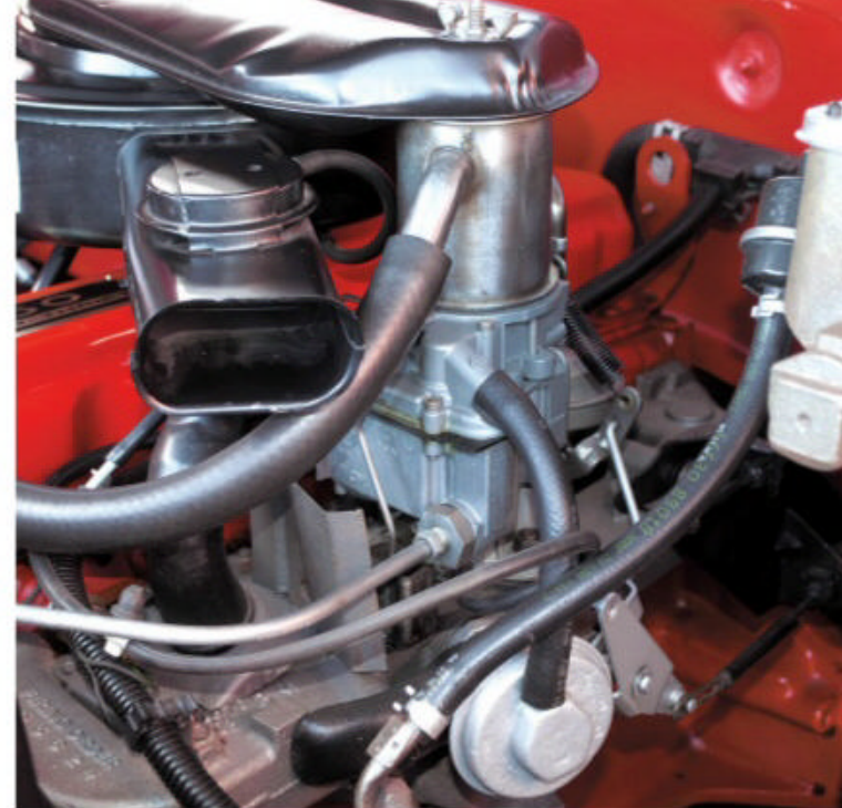
This truck is powered by its original 250-cu.in. inline-six, and breathes through a one-barrel carburetor. The 250 was the base engine for this truck, but it was optioned up with power steering, power brakes, and an automatic transmission.
