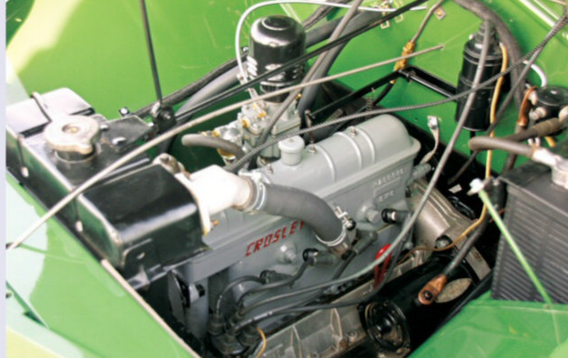
The SOHC four-cylinder engine was developed during World War II and initially built using a brazed-together sheetmetal block.
