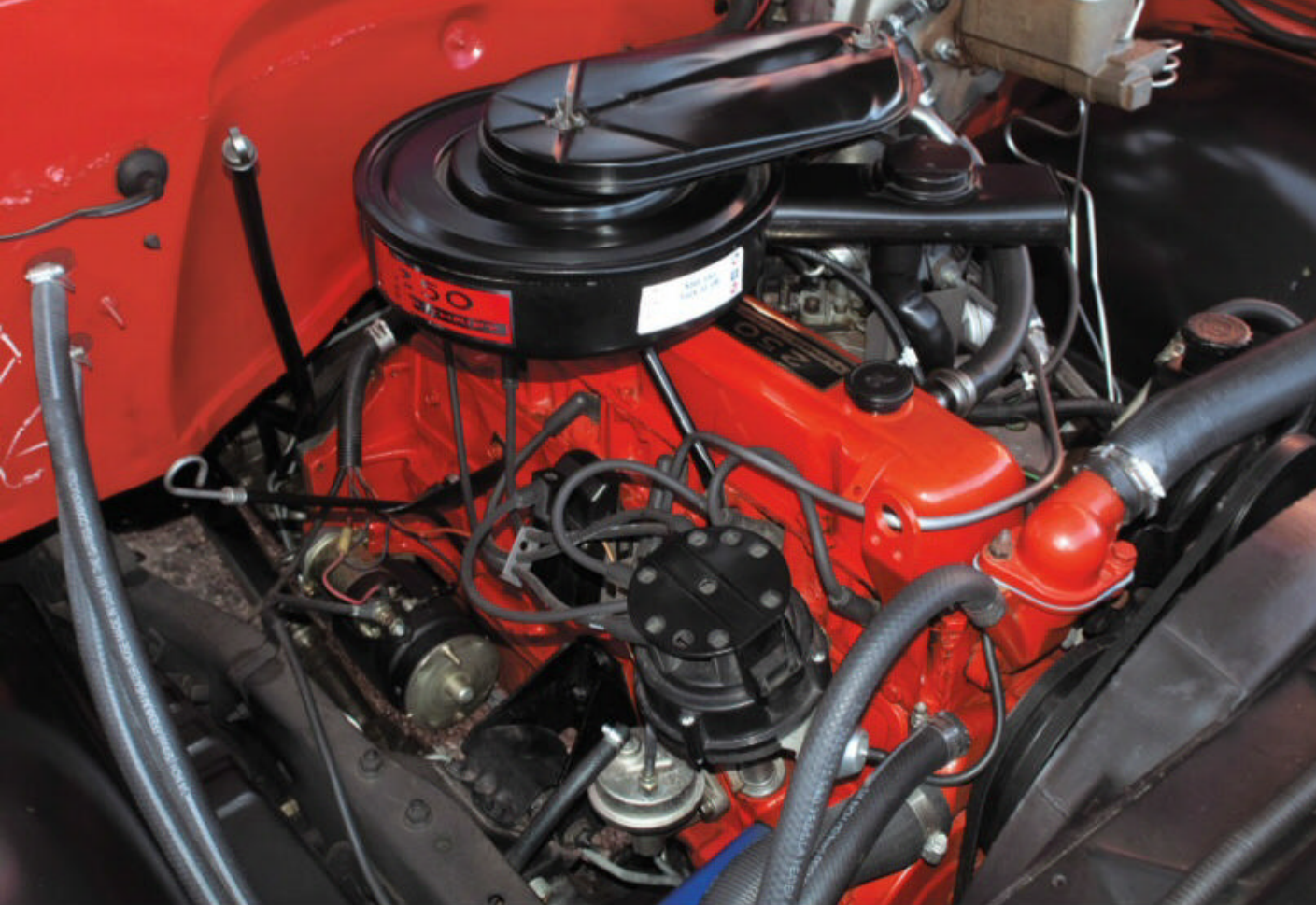
This truck is powered by its original 250-cu.in. inline-six, and breathes through a one-barrel carburetor. The 250 was the base engine for this truck, but it was optioned up with power steering, power brakes, and an automatic transmission.
