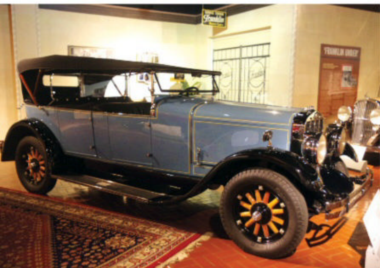
Featuring four-wheel hydraulic brakes, this 1928 Series 12B Sport Touring was one of the new “Airman” models; it was designed by Ray Dietrich.
