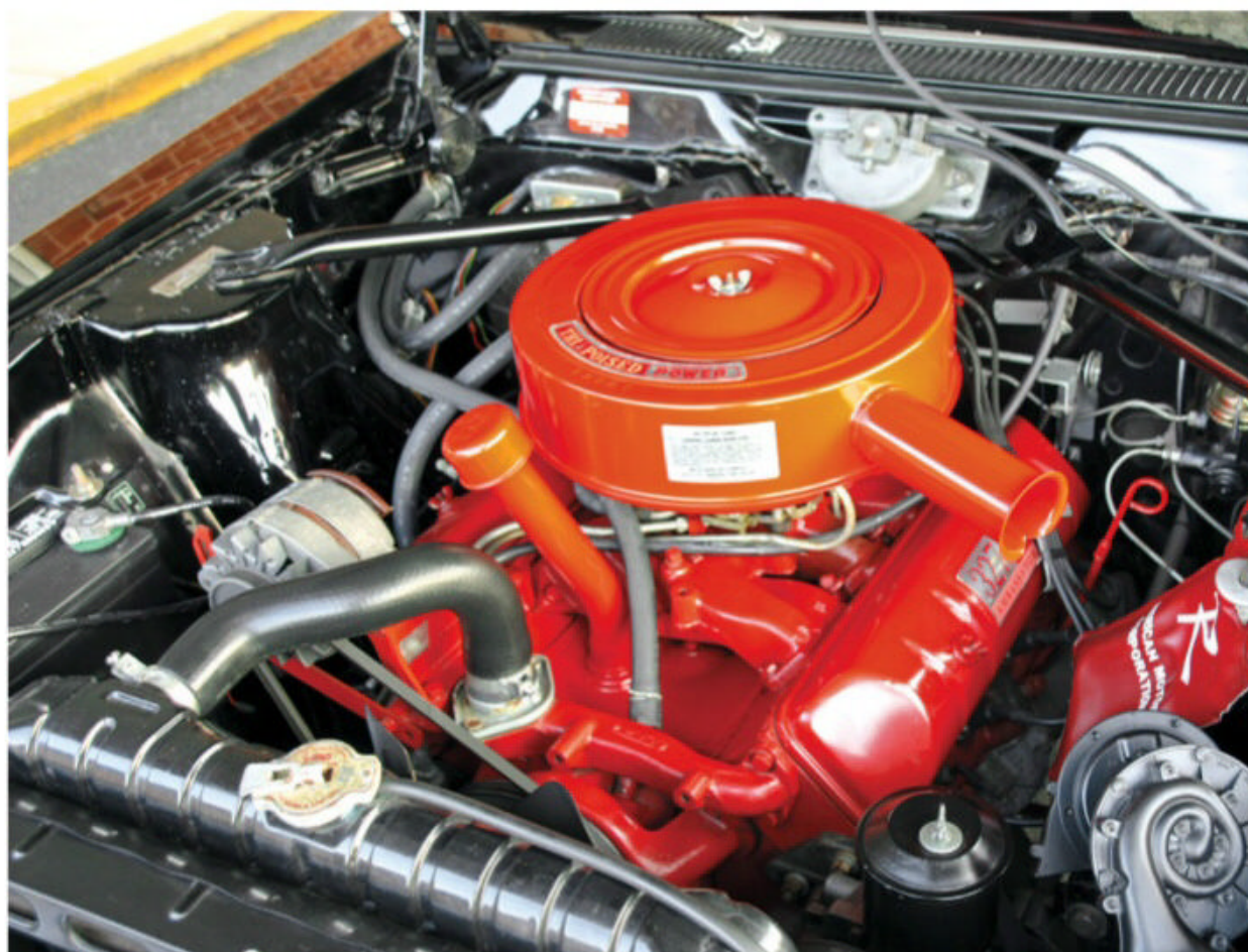
Rambler's hottest V-8 was stock: 1964's 270-hp, four-barrel 327-cu.in. V-8 moved the 3,213-pound hardtop with authority. The cylinder heads were machined .010 for a slight bump in compression.
