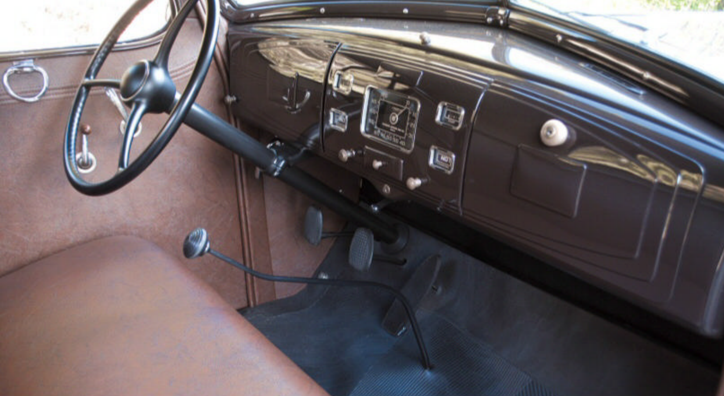
A floor-shifted three-speed was standard, Selective Automatic Shift was optional. "Quick-vision" speedometer is surrounded by gauges for gas and temperature. "Teleflash" warning lamps monitor oil pressure and charging.
