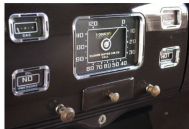
A floor-shifted three-speed was standard, Selective Automatic Shift was optional. "Quick-vision" speedometer is surrounded by gauges for gas and temperature. "Teleflash" warning lamps monitor oil pressure and charging.
