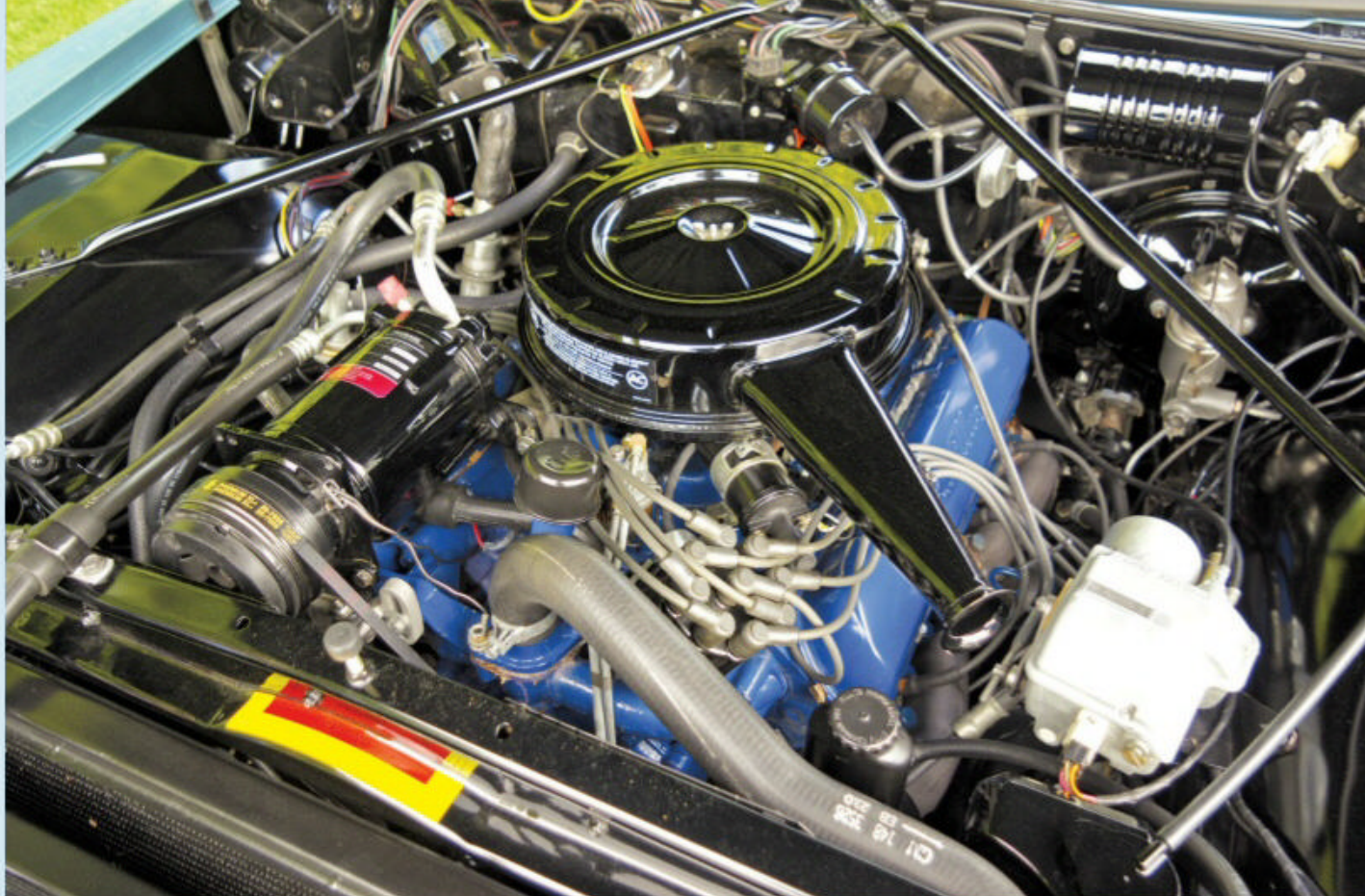
A low-mileage 340-hp 429-cu.in. four-barrel V-8 was rebuilt to stock specifications and detailed to concours condition. Underhood decals were replaced, although the owner had to have some decals reproduced.
