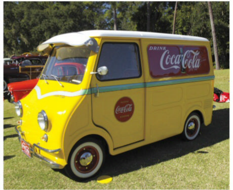
Attracting spectators throughout the day was this cute 1958 Goggomobile TL400 Transporter. Owned by Billy and Sue Paul from Longwood, Florida, it's powered by a 400-cc two-stroke two-cylinder with a pre-selector four-speed.
