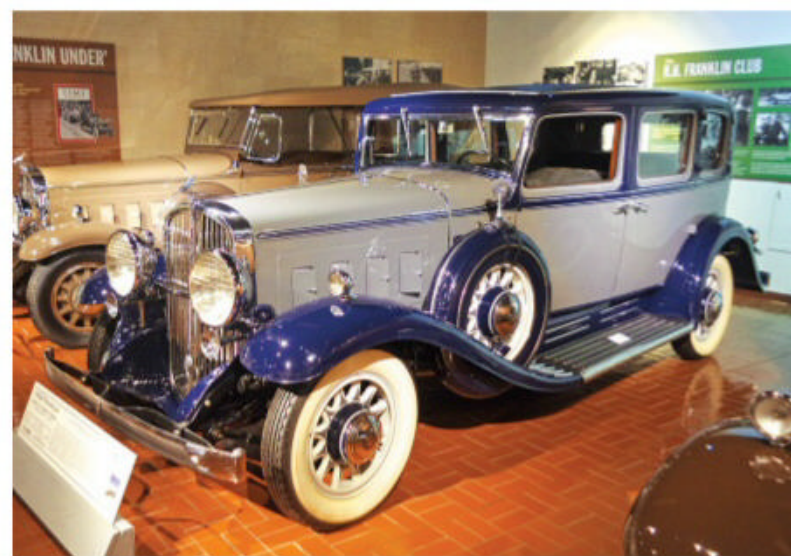
Utilizing air bleed from the cooling fan, the "supercharged" 274-cu.in. straight-six gives this 1932 Series 16 "Airman" sedan 100 horsepower.
