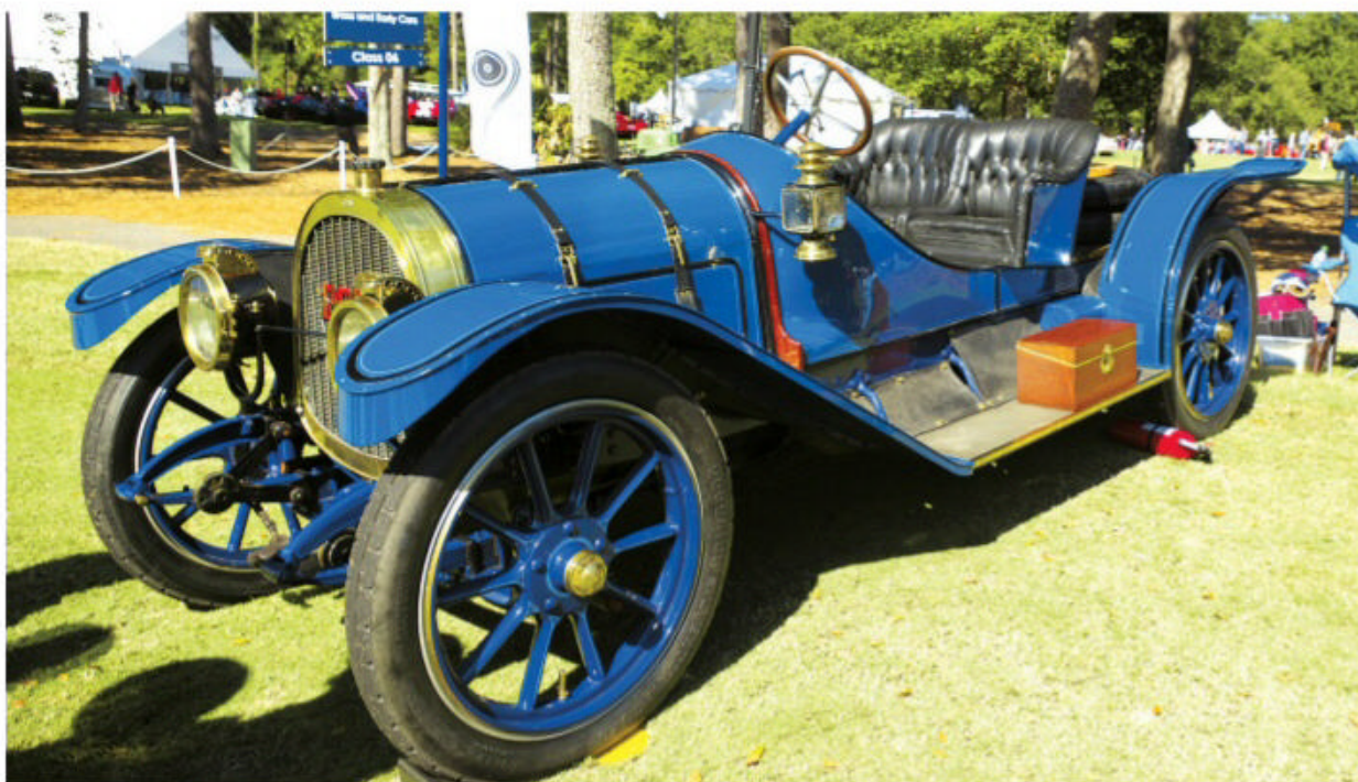
As its name implies, this 1911 Pope-Hartford Portola Roadster was built in Hartford, Connecticut, and is one of three known to exist. With a 50-hp four-cylinder displacing 450 cu.in. under the long hood, it's owned by David Peeler of Weddington, North Carolina.
