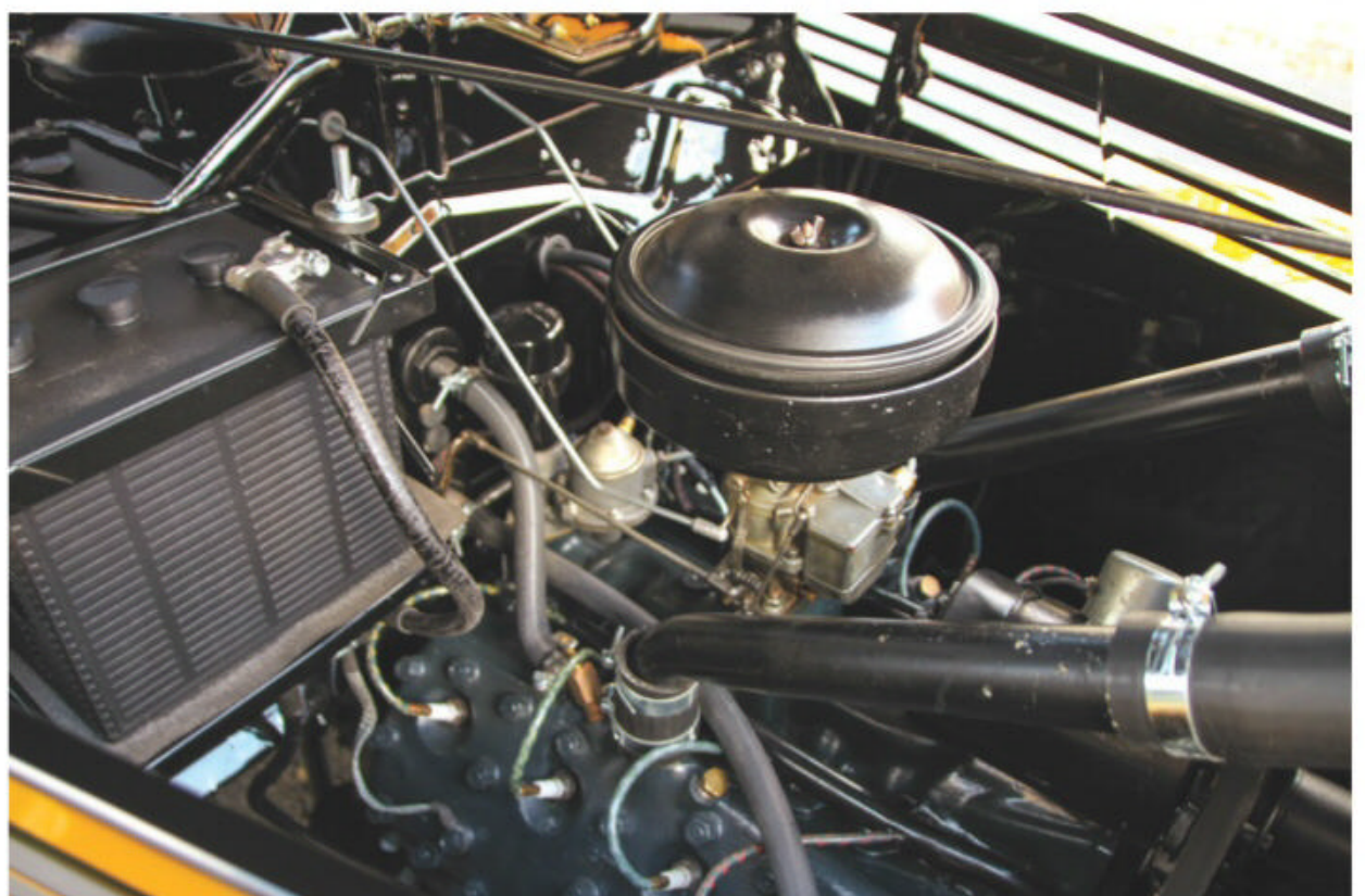
Below the Tonner's new-for-1938 front-opening hood, the 85-hp, 221-cu.in. "flathead" V-8 sits low and somewhat snugly against the front-end metal.
