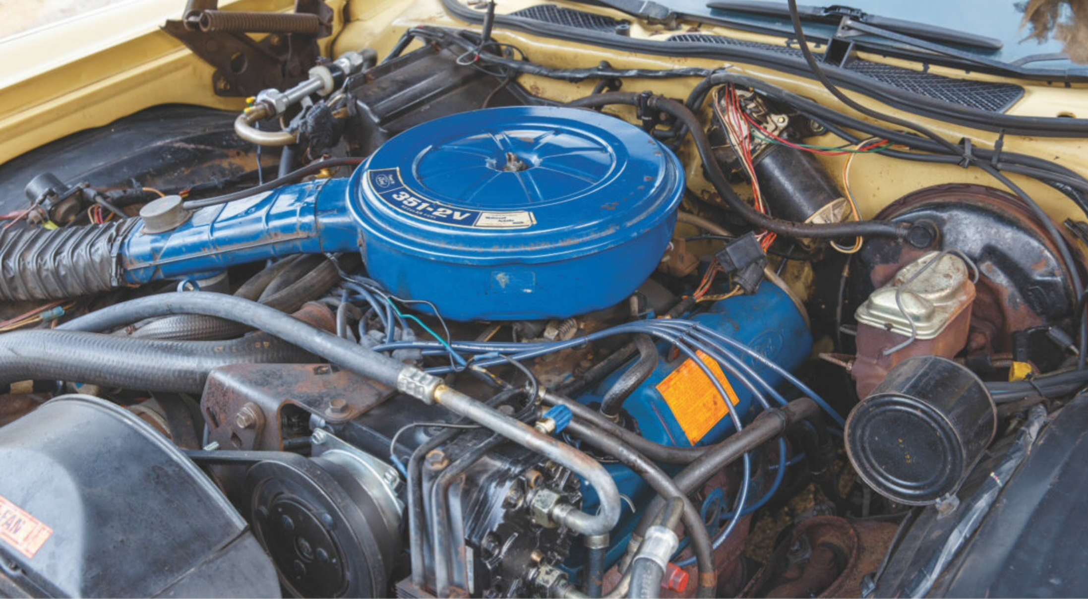
The 162-hp 351-2V Cleveland V-8 was the engine with lowest output of four choices for 1974, but does a competent job of propelling the car.
