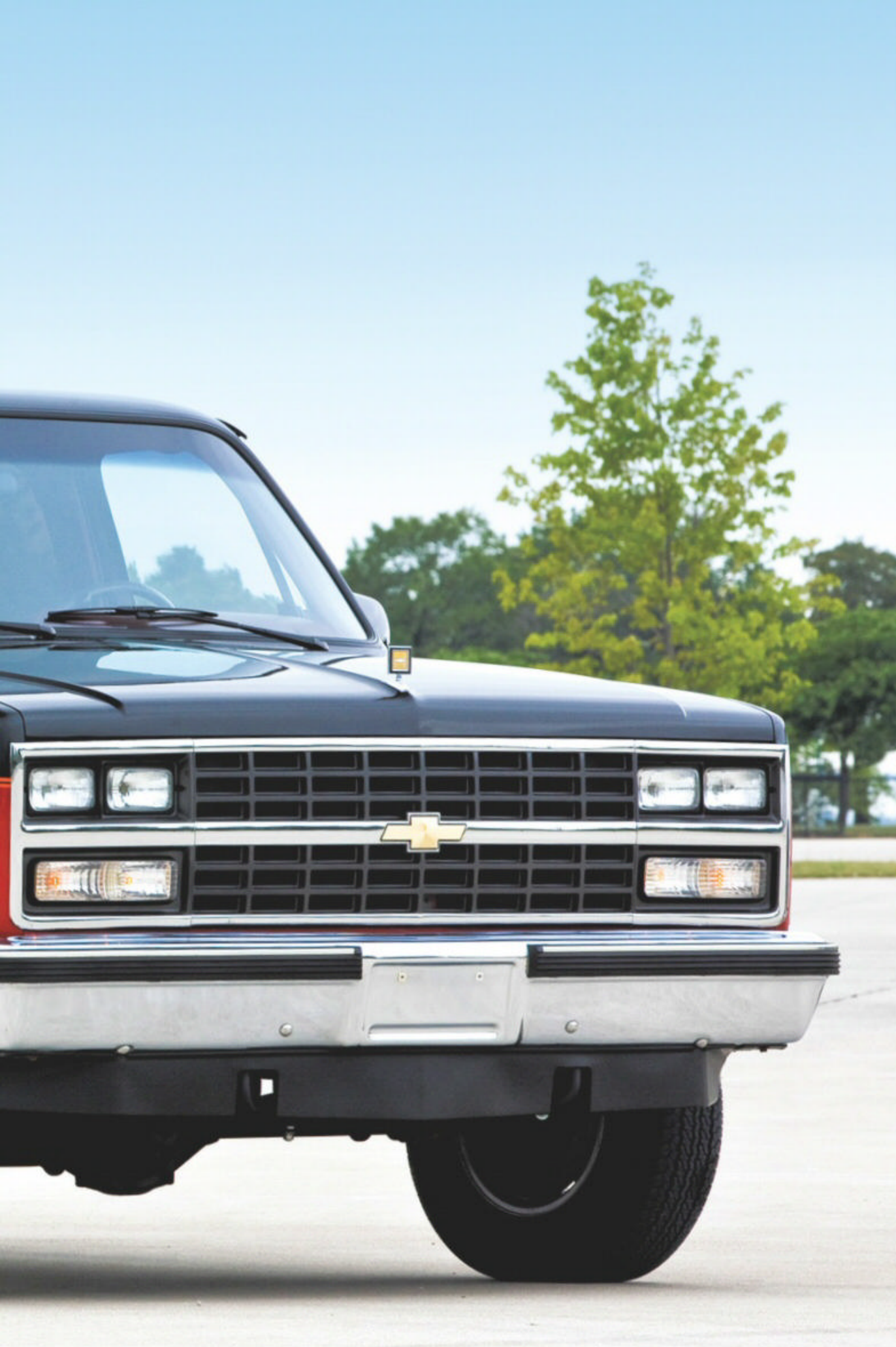
This two-tone Onyx Black and Fire Red 1990 Chevrolet Suburban is part of General Motors' collection and nicely optioned with the Silverado package, extra-cost aluminum wheels, and more. Under the hood is a throttle-body injected 350-cu.in. V-8 rated at 210 horsepower, paired with a four-speed automatic transmission.
