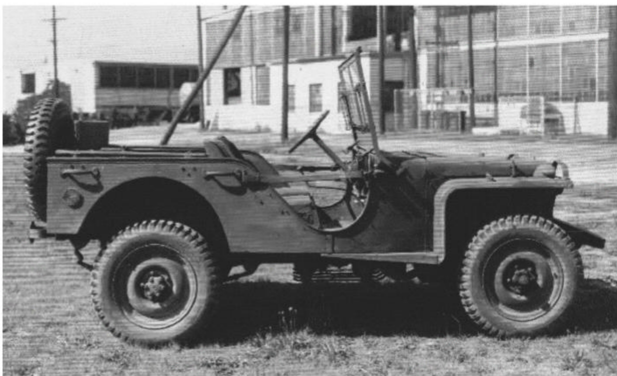
With World War II approaching Checker tried to earn additional business doing modifications of military Jeep vehicles, as depicted here with this modified 1941 Bantam Jeep with Checker-installed four-wheel steering.
