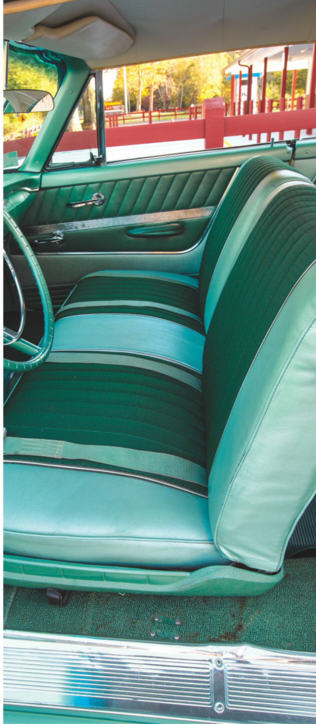
Spacious Ford interiors of the early '60s can be quite beautiful. Starliner features vinyl upholstery with pleated shimmer nylon inserts. Shimmer comes courtesy of silver Mylar threads.
