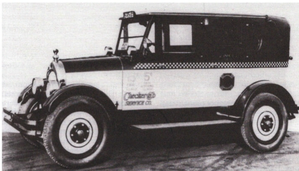
The 1926 Model F is easy to spot because of its unique slanted windshield, a feature used for this one-year only model.
