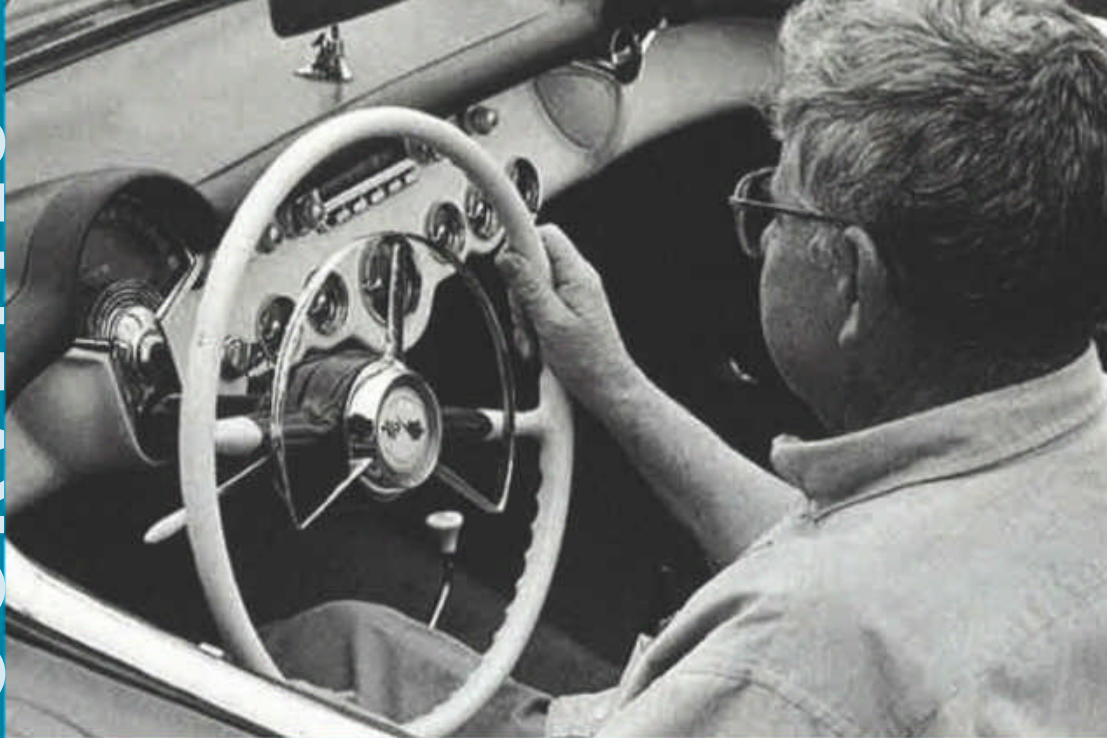
Symmetrical instrument layout makes oil and amp gauges difficult for driver to see. Baffling Powerglide control comes out of side of tunnel-like early Austin-Healy shifters.
