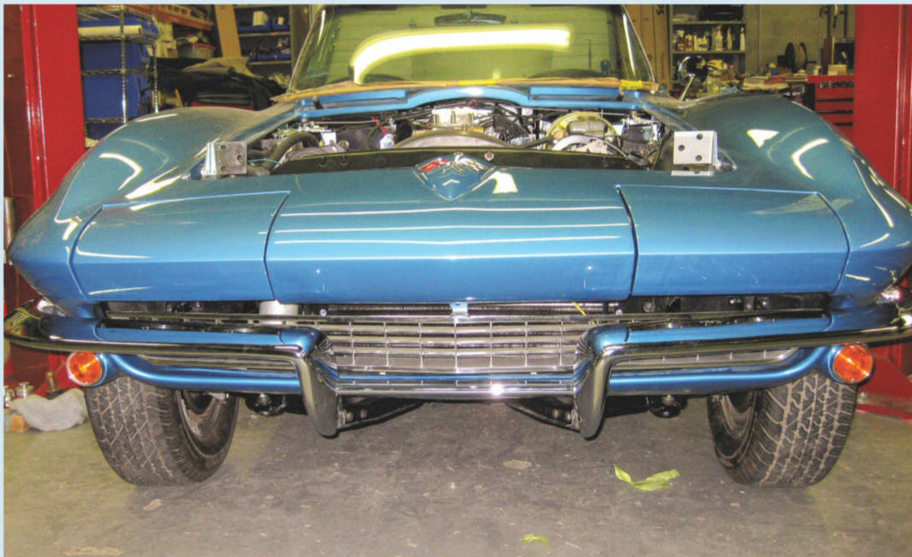
As the high-end restoration of this Sting Ray progressed to nearing completion, the grille was installed, as were the re-chromed front bumper assembly and crossed-flags emblem. The hood was bolted on next.
