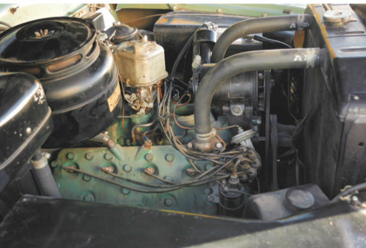
Mercury's famed flathead V-8 displaced 255.4-cu.in. in 1951, and produced 112 horsepower and 206 lb-ft of torque. With so few miles showing, this engine has never been apart for service.
