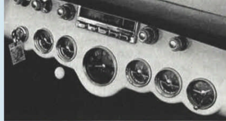
Symmetrical instrument layout makes oil and amp gauges difficult for driver to see. Baffling Powerglide control comes out of side of tunnel-like early Austin-Healy shifters.
