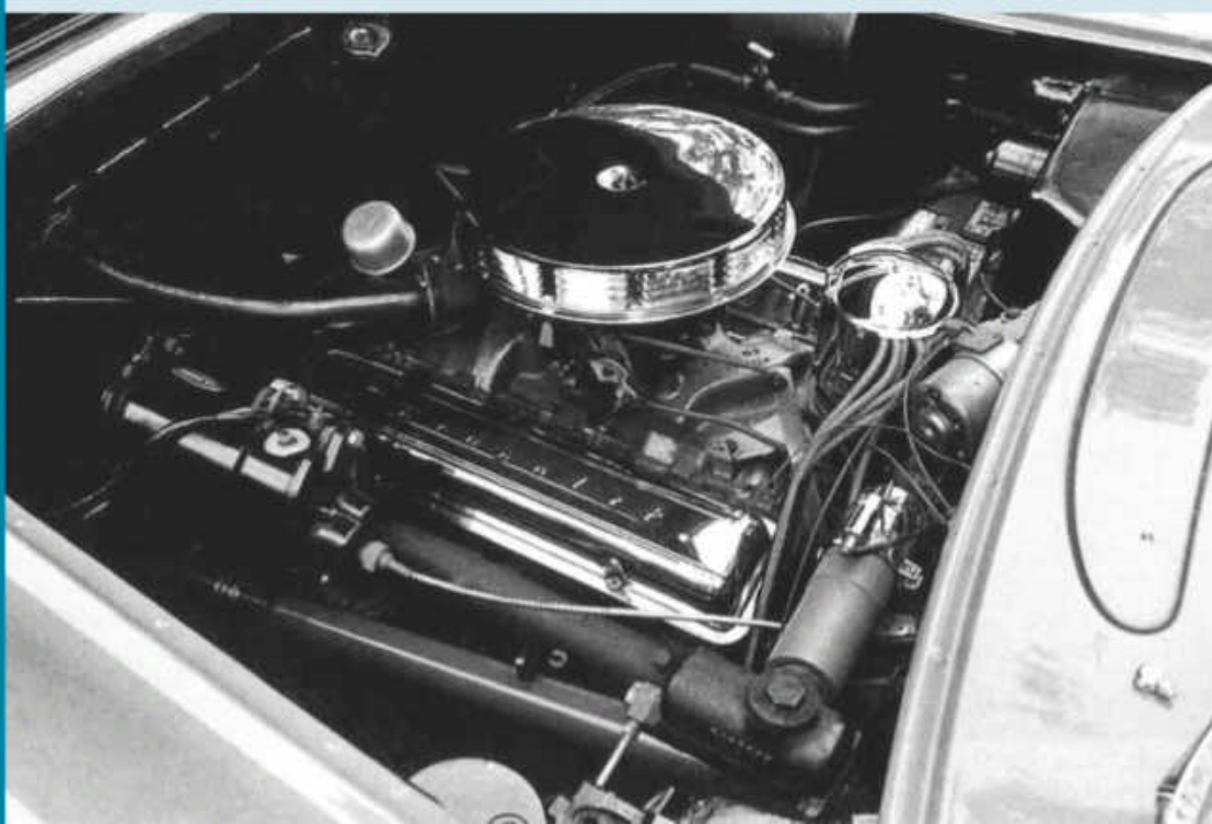
driveReport car has been personally autographed by its chief creator. Chromed valve covers distinguish Corvette engine from Chevy passenger car V-8s.
