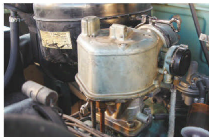
Mercury's famed flathead V-8 displaced 255.4-cu.in. in 1951, and produced 112 horsepower and 206 lb-ft of torque. With so few miles showing, this engine has never been apart for service.
