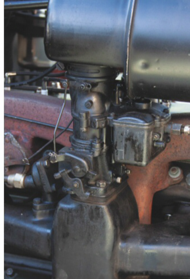
The 384.4-cu.in. eight was rebuilt with new pistons, valves, and poured Babbitt bearings. The Stromberg carburetor was simply adjusted.
