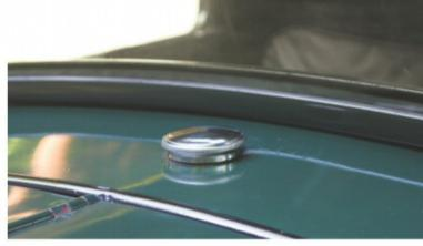
Ford still used a gravity-fed fuel system in 1931, so the tank was still hidden below the top of the cowl. The Model A pickup's cabin is best described as utilitarian, decorated with only a few necessary gauges. An aftermarket turn signal system was added in the name of safety.
