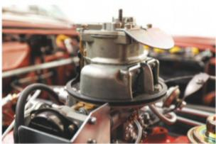
The supercharged engine is the core of what makes this car special. Because the original was missing, Don had to recreate it by seeking out everything, right down to the special rubber washer that helps seal the top of the blower bonnet.
