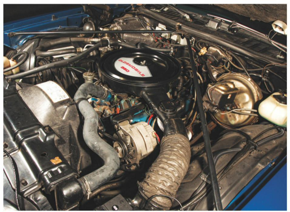
Oldsmobile's four-barrel 350 (the Rocket name was retired by then) was rated at 170 net horsepower for 1976, and could only be mated to a Turbo 350 automatic transmission. Air conditioning was an option. This 35,000-mile original is untouched save for hoses and fluids.
