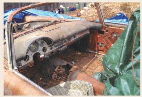
This is the Thunderbird's cockpit, pre-restoration. The previous owner had painted the engine compartment black, probably when he first installed the Corvette 283, but the original Thunderbird Bronze paint is still visible on the door structure.
