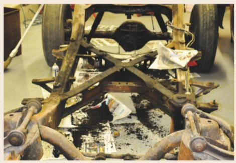
"This was the dirtiest part of the restoration, but not too hard to do," Don says. Along with four muscular friends, Don lifted the body off by hand and moved it aside for later. Then the frame was treated to scraping, cleaning, and media blasting.
