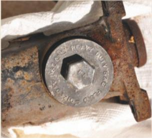
The original Bendix Brakes master cylinders had a zinc cap that was prone to seizing on the threads of the cast-iron body. Don found the correct pieces for his car and spent days gently persuading the cap off using heat, leverage, and penetrants.
