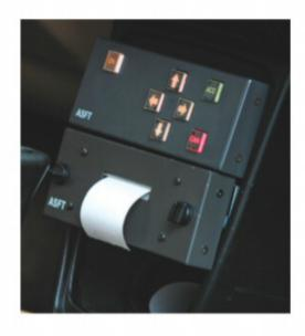
to 100 mph. A torque sensor read the resistance against the chain drive, and fed this information to an onboard computer that transmitted in real time to Air Traffic Control, which in turn relayed runway condition codes — 0 to 6, with 6 being dry and good braking—to incoming and outgoing pilots.
