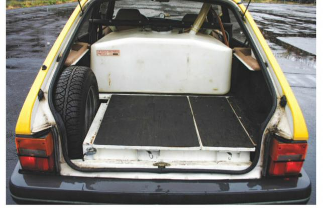
SFT #244 was built with the optional water tank and rear suspension air shocks, the latter of which would be inflated to 30 psi/2.1 bar. The right-side floor hatch hides a jack storage compartment and measurement computer, while the left hatch reveals the friction-testing fifth wheel assembly. This unit raises and lowers hydraulically, and its 8-inch wheel is fitted with an aircraft-type tube tire with a specific rubber compound.
