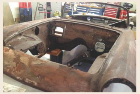
The engine compartment, exterior, and underside of the hood (but not the sound deadener in the trunk) were stripped and scraped by hand over the course of several "long and nasty" weeks. The hard work made it easier for the media blaster to avoid damaging the metal.
