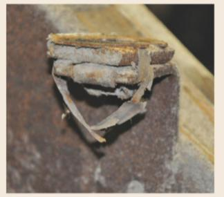
Before removal, Don documented every shim, measured them with a caliper, and stamped numbers on each. A sketch indicated the original location of each shim, permitting reinstallation a year later after they had been media blasted and cadmium plated.
