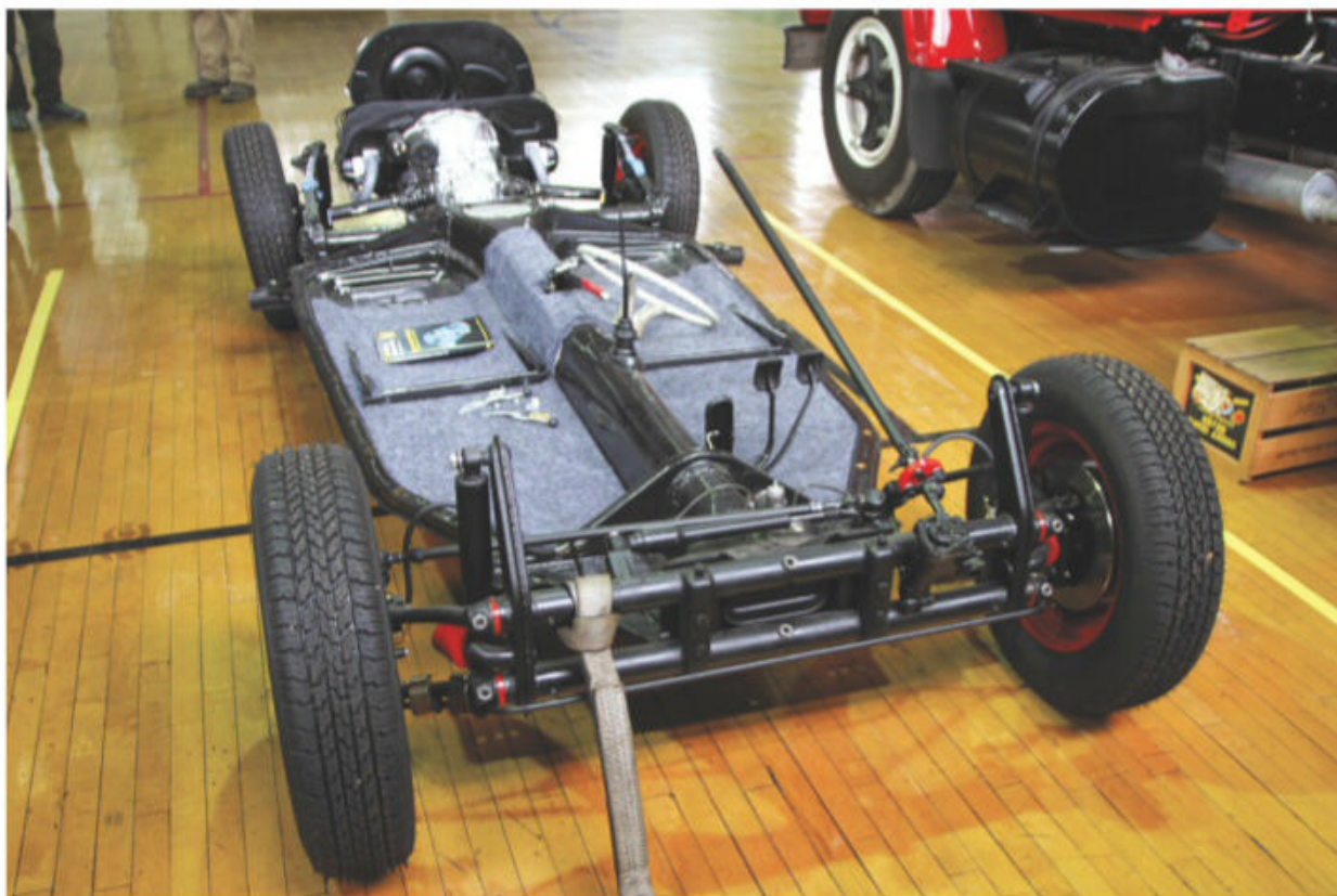
One of the more difficult restorations was a 1965 Volkswagen Sunroof Sedan, its chassis seen here. The challenge wasn't the car's design, but rather finding parts that fit correctly.
