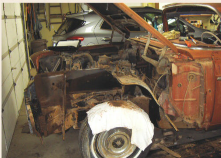
Careful measurements of panel gaps were taken before the front sheetmetal was disassembled. Those measurements wouldn't prove as useful as hoped, but the metal ended up being in great shape. Five bolts secured the front inner sheetmetal assembly.
