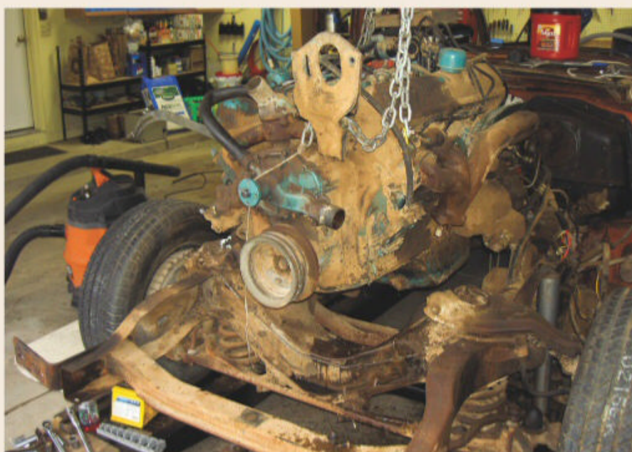
The 364-cu.in. "nailhead" was covered in oil and desert dust, and came out after a hidden transmission shift linkage bracket was found and freed. The V-8 would be transferred to an old welding cart for support so its condition could safely be evaluated.
