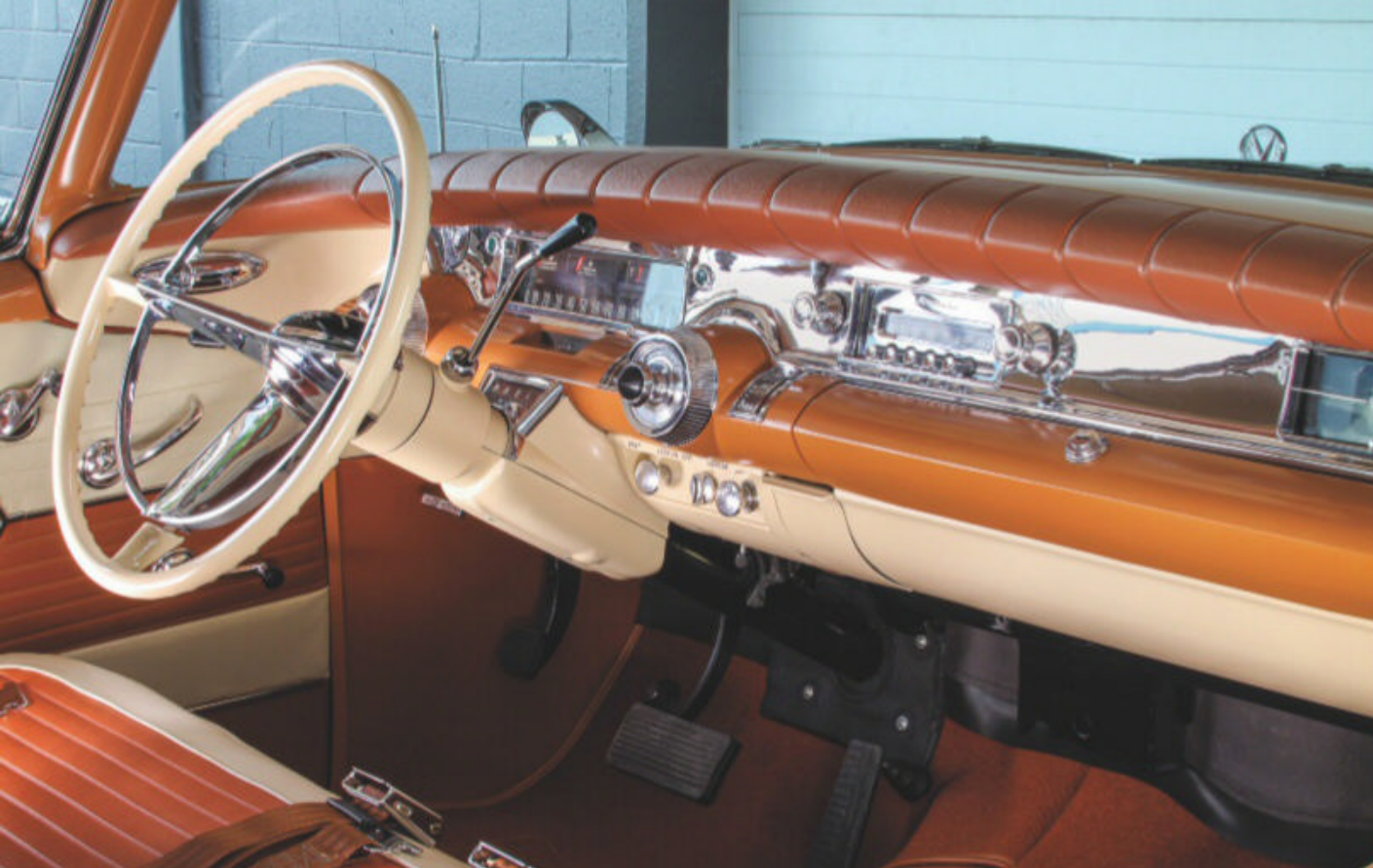
Jet Age influence was seen in Buick's turbine blade-styled lighting and vent control bezels, plus vent control sliders like "T" handle throttles. Carpeted load floors and seatbacks were unique to Caballero.
