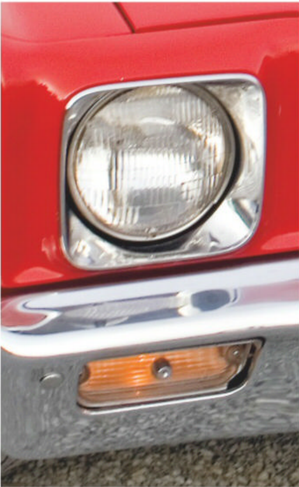
LEFT: For 1970, the headlamp bezels have a rounder shape and the signals in the bumper are round. RIGHT: For 1971, the bezels were squared up and the signals became rectangular. For 1972 (not shown), the signals were vertical and in the outer edges of the grille.
