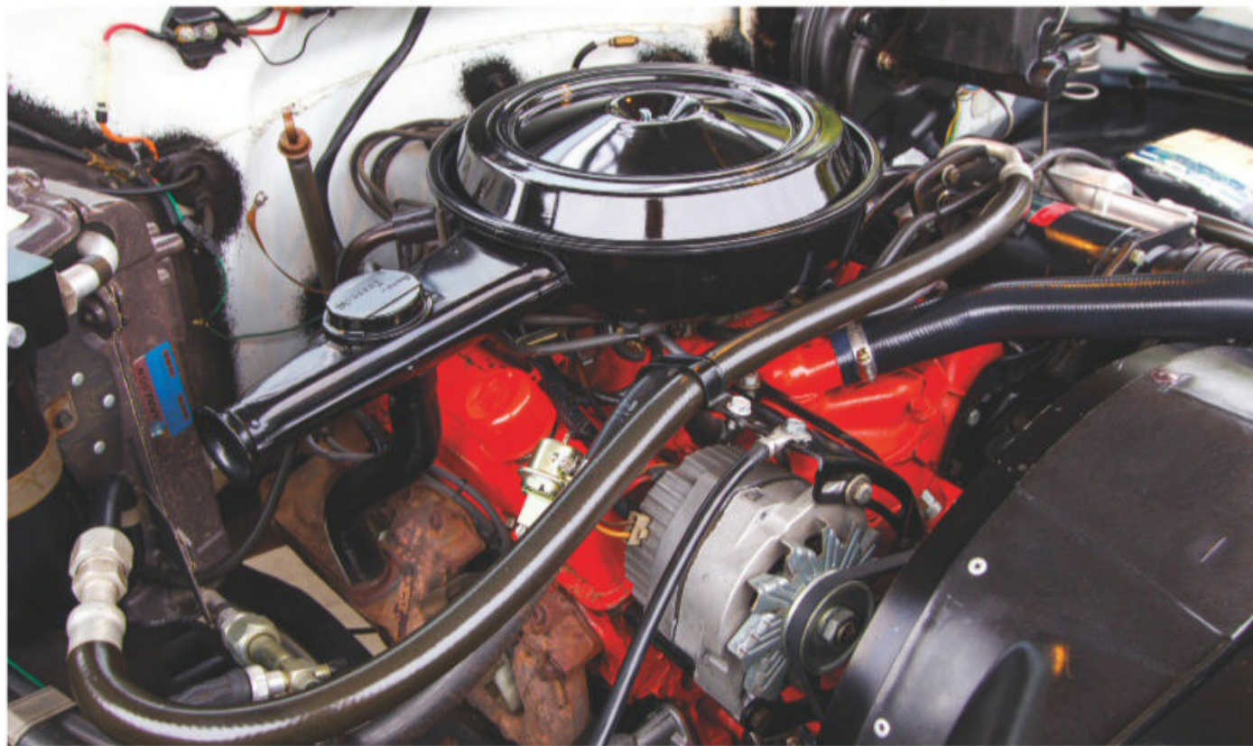
The Blazer's four-barrel 350 has never been rebuilt, nor has the Turbo Hydra-Matic 350 transmission or any other drivetrain component. Notice the lip pop-riveted around the inside circumference of the radiator shroud, which Bill installed to increase the fan's efficiency.
