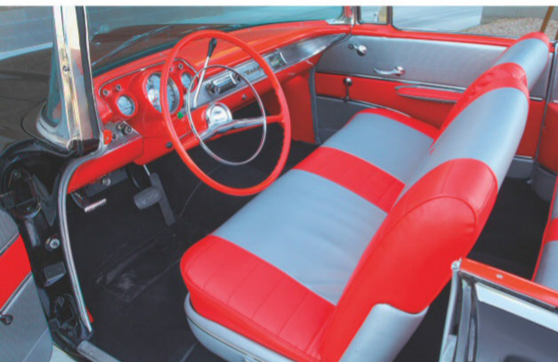
An all-new instrument panel, with a round speedo replacing the previous seashell shape, backs a two-spoke tiller. Far edges of the dash are now raised; too many complaints of smashed knees?
