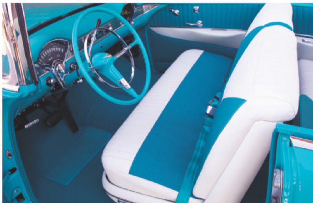
If it ain't broke, why fix it? Save for door panels and upholstery patterns, the '56 interior was largely a carryover from 1955. This example is an automatic with power brakes and aftermarket lap belts.
