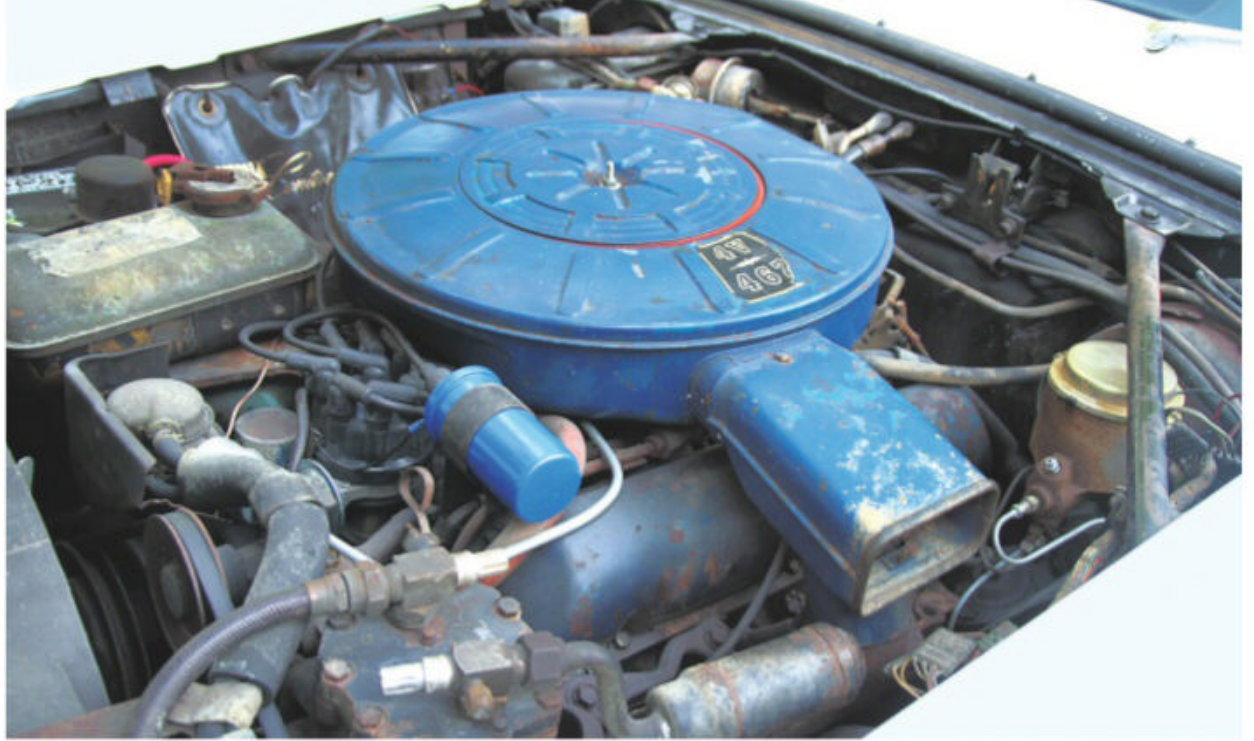
The Lincoln's original 430-hp 462-cu.in. engine didn't crack during decades of storage; a basic tune-up had it running like new.
