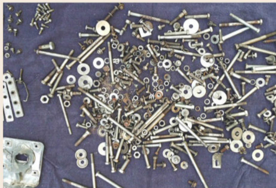
Wherever possible, original fasteners were reused, prepped for replating with original or current equivalent coatings by degreasing and tumbling or glass bead abrasive cleaning. Plating services were provided by Williams Finishing and Mid-States Plating Co. in Michigan.
