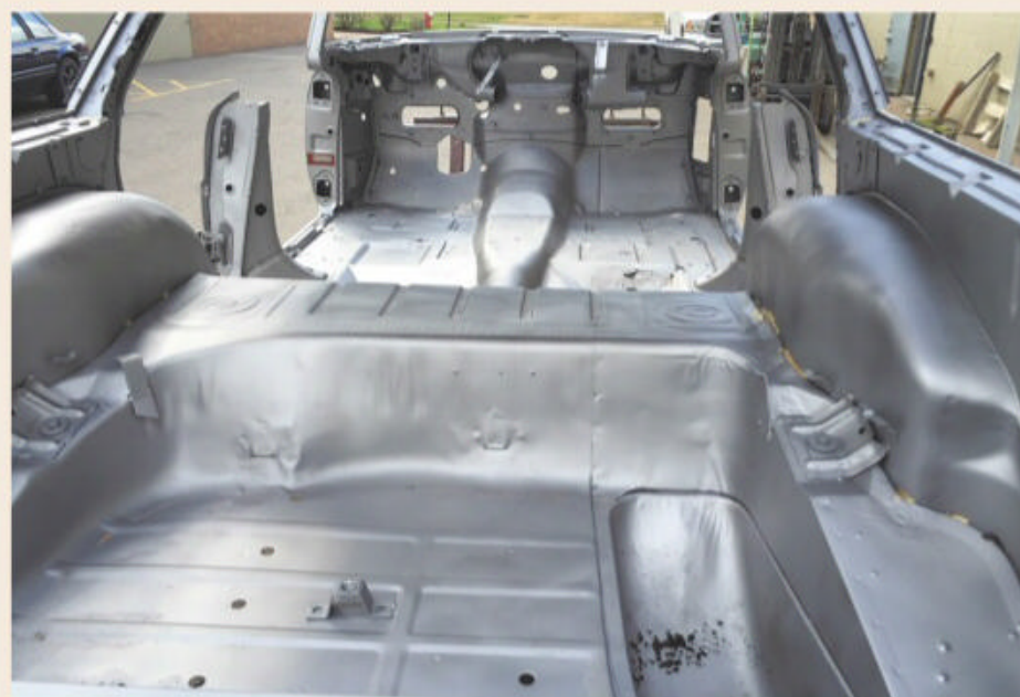
The body went to SS Stripping in Sterling Heights, Michigan, for abrasive cleaning and priming; desert notwithstanding, leaves, dust, and debris had rusted areas of the floorpans, wheel wells, and inner rockers. SS Stripping powder coated the frame, suspension, and driveline parts.
