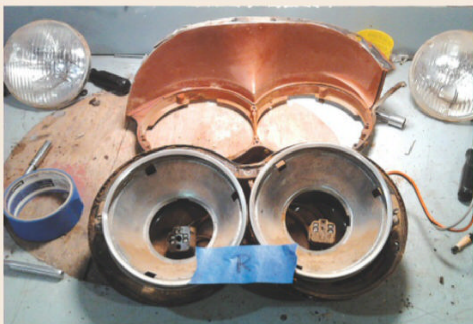
The painted headlamp adapters, located above the headlamps and under the eyebrow of the fenders, were removed and kept as paint master samples. The new paint spray-out panels were an exact match to the car's factory applied metallic Garnet Red color.
