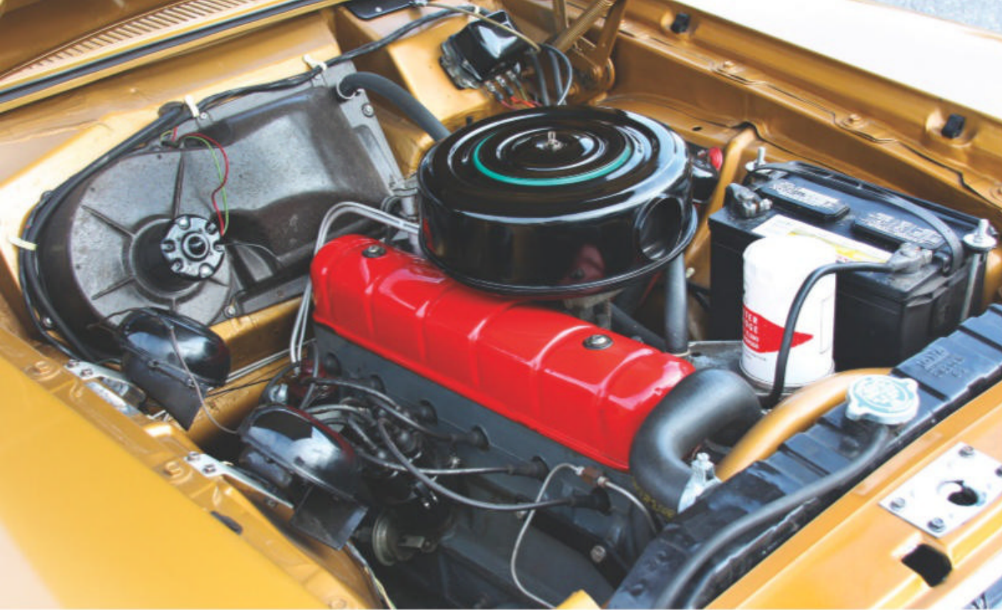
The 195.6-cu.in. OHV inline-six has roots going back to flathead designs before World War II. By 1962, it was rated as high as 138 hp, when topped with a two-barrel carburetor.
