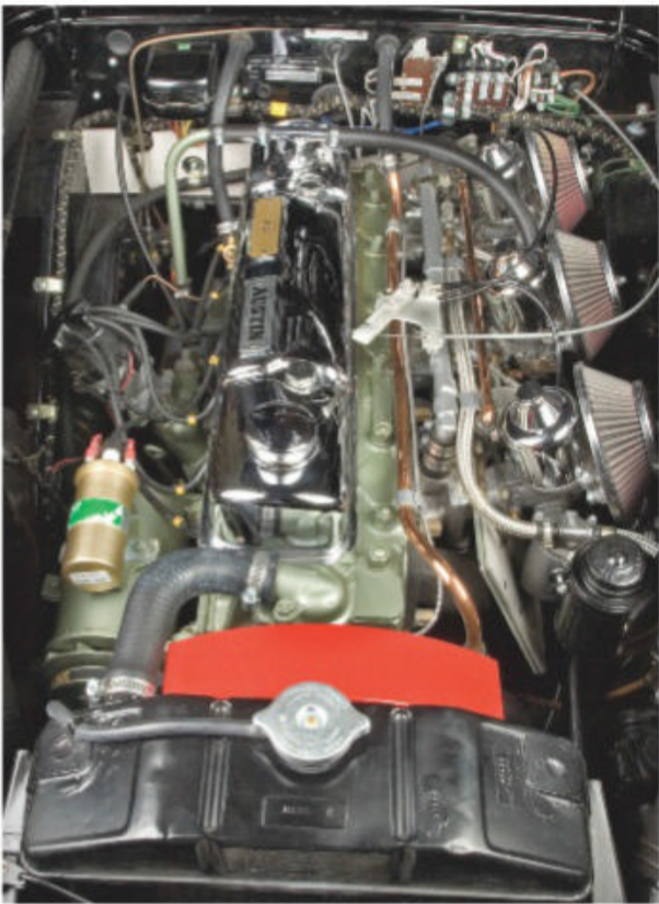
The 2,912-cc straight-six engine used in all 3000s is notably powerful, largely reliable, and enjoys great parts availability. It differed in carburetion and camshafts over the course of its nine-year life, and ultimately made 150 hp and 173 lb-ft of torque.
