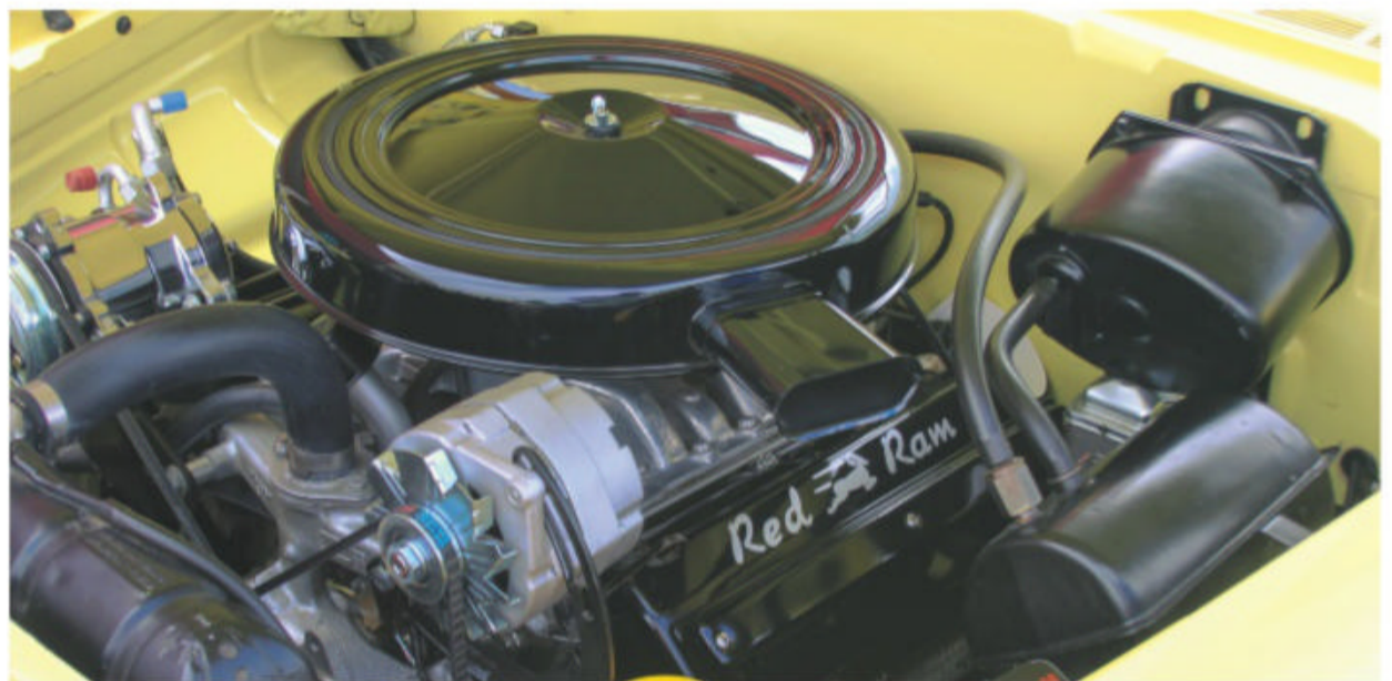
The 325-cu.in. V-8 made 285 horsepower with two-barrel carburetion and supplied ample power. The Delco-style alternator is a retrofit, as is the compressor for the upcoming A/C system.
