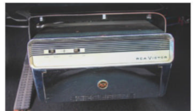
An RCA record player was a rare option not found on many cars of this era. The 45-rpm player held 13 records and played them upside down, so that the weight of the record kept the needle from skipping.
