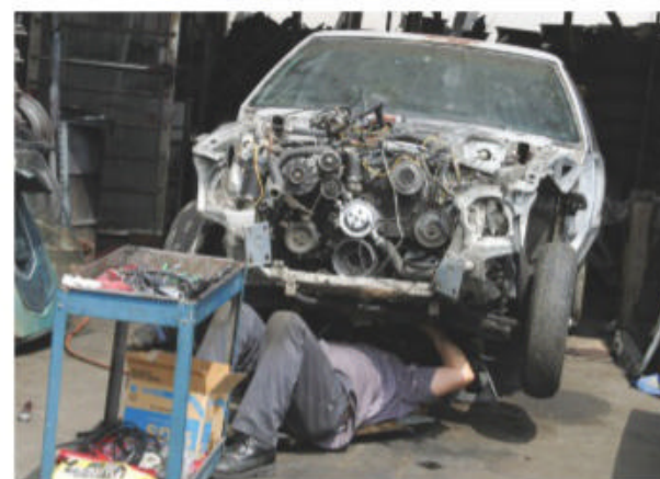
Always use jack stands rated for at least 2 to 3 tons and positioned beneath the frame rails (or other solid jacking points), with a backup system in place should the stands fail.
