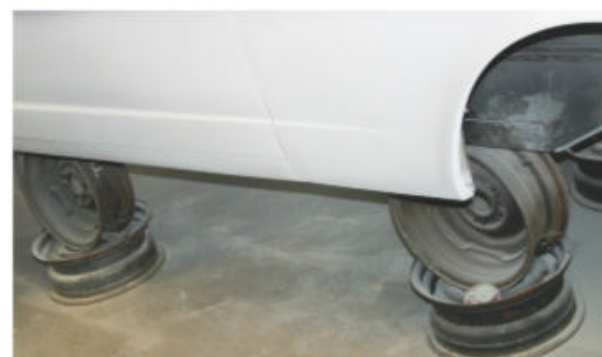
There are many approaches to supporting automobiles — some quite dangerous, like this one. Salvage yards are fond of using wheels for vehicle support — don't try this at home. Use jack stands as a more solid means of support.
