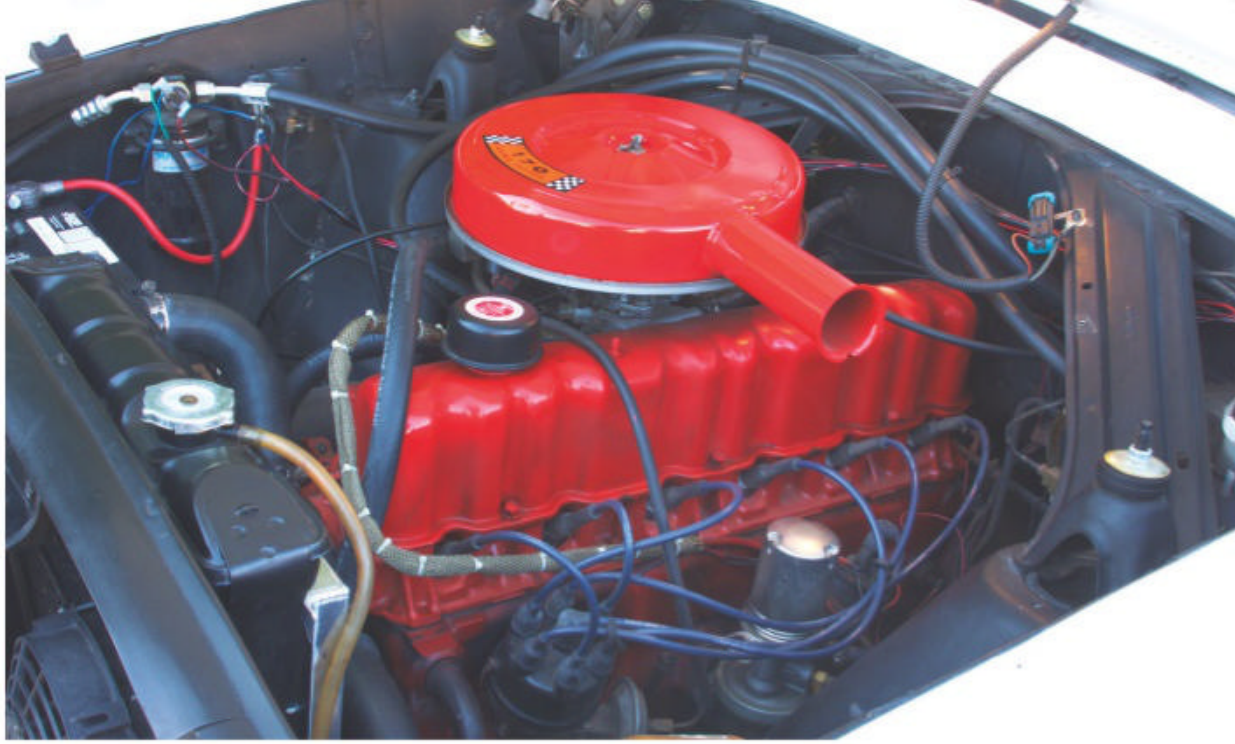
A replacement 170-cubic-inch inline-six, rated at 101 hp, now shines between the shock towers; a contemporary A/C compressor is hidden low beside the block.
