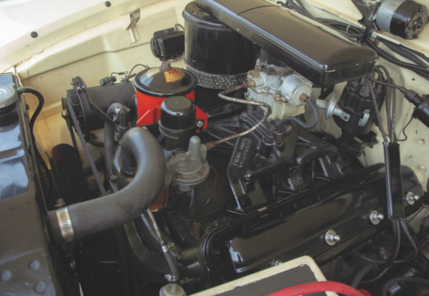
Studebaker's V-8 engine debuted in the 1951 Commander. It remained in production through the 1964 model year, growing from 233 to 304 cu.in., and moving from a single two-barrel carburetor to available dual-quad and supercharged induction. The bullet nose on 1951 models is different from the similar 1950 unit.
