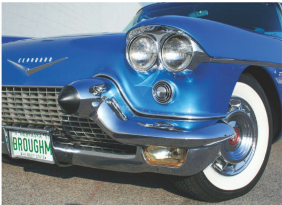
The Brougham was the first GM car to utilize quad headlamps, which would not become standard in the industry until 1958.
