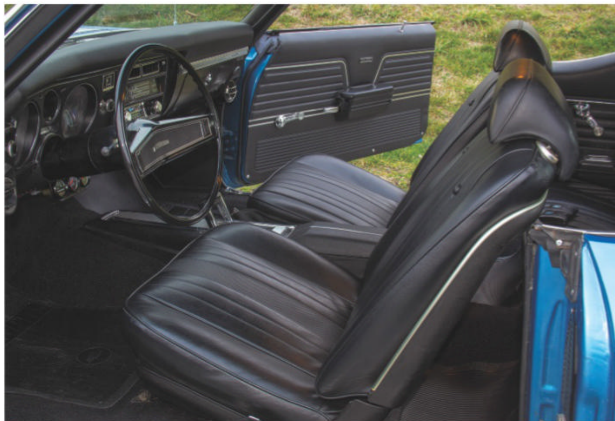
The instrument panel and rear seat are original; the dash pad, carpet, and door panels were replaced; and the front seats were reupholstered by Weimann's Interiors in Delmont, Pennsylvania. Dennis will soon swap the aftermarket radio for the stock AM/FM unit from his first Malibu.
