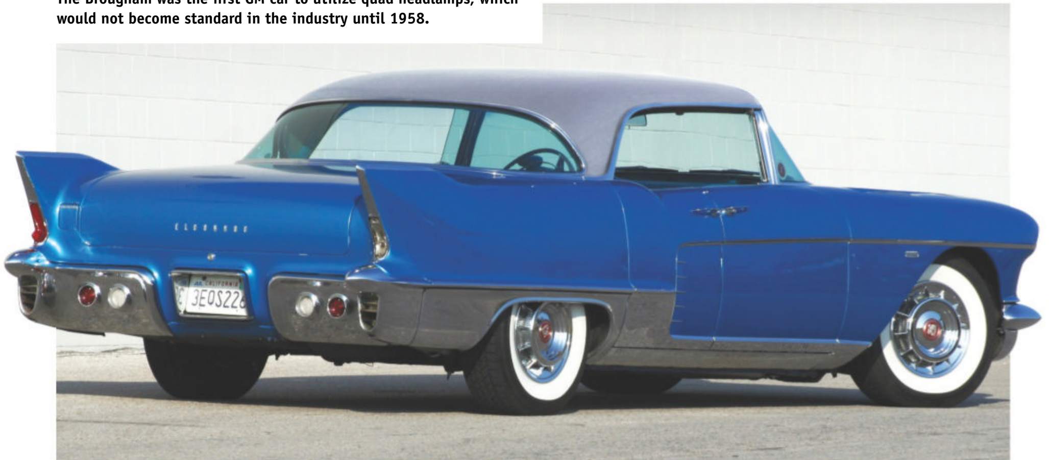
A unique feature for the Brougham was its stainless-steel roof. This motif was originally seen on the 1953 Orleans and 1954 Park Avenue show cars — the first a four-door pillarless hardtop, and the other a four-door sedan — but both used polished aluminum roof panels instead of stainless steel. A few days prior to this photoshoot, Gus broke a taillamp lens and spent the next several weeks in search of an NOS replacement.
