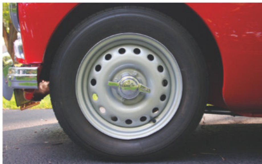
Mk II De Luxes sported leftover MGA Twin-Cam 15 x 4-inch Dunlop steel wheels fronting four-wheel disc brakes. These wear era-correct Michelin X radials.
