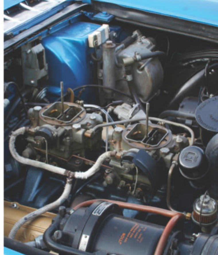
Cadillac's powerful 365-cubic-inch V-8 with dual Carter four barrels was employed to move this heavy beast down the road.
