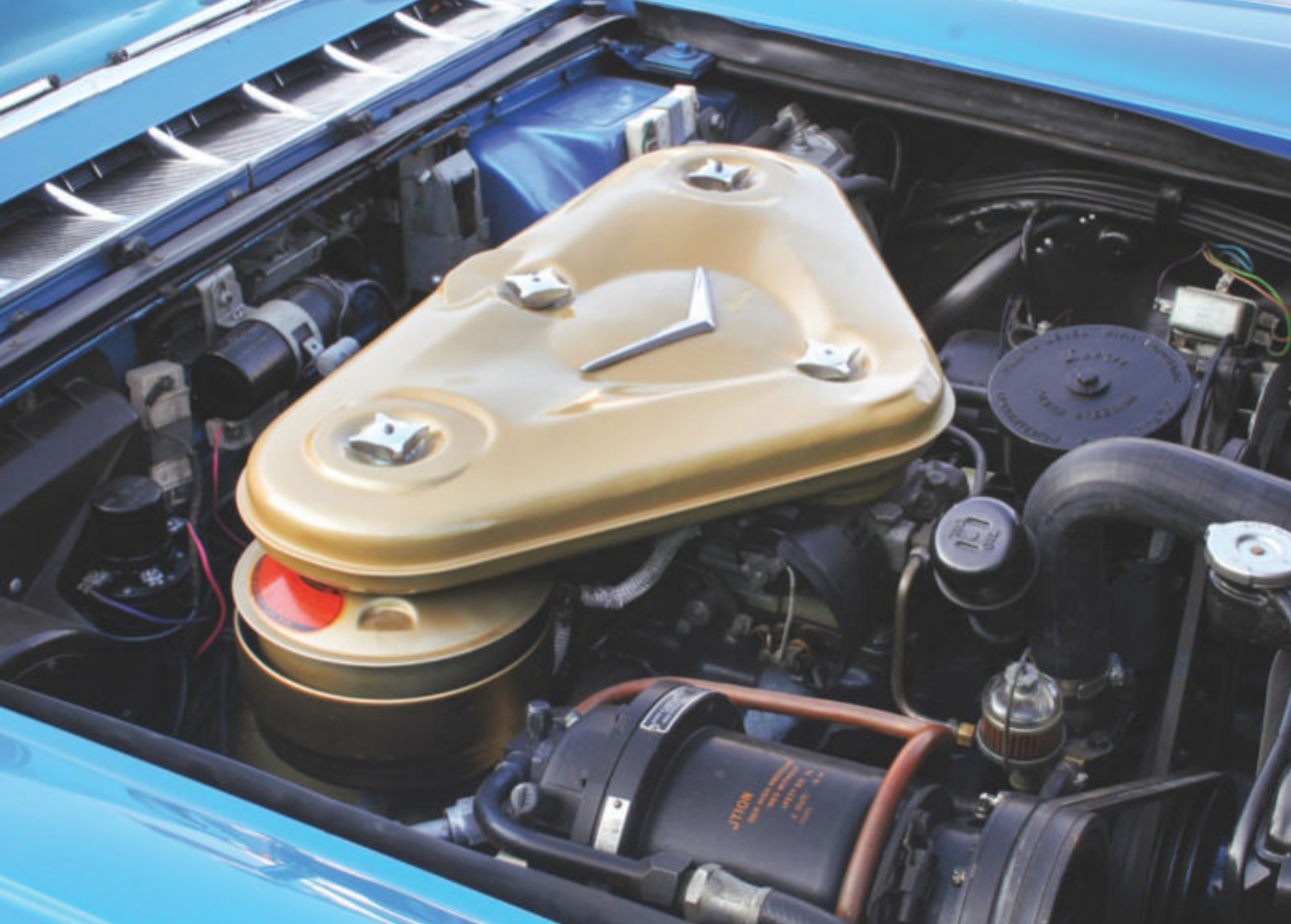
Cadillac's powerful 365-cubic-inch V-8 with dual Carter four barrels was employed to move this heavy beast down the road.
