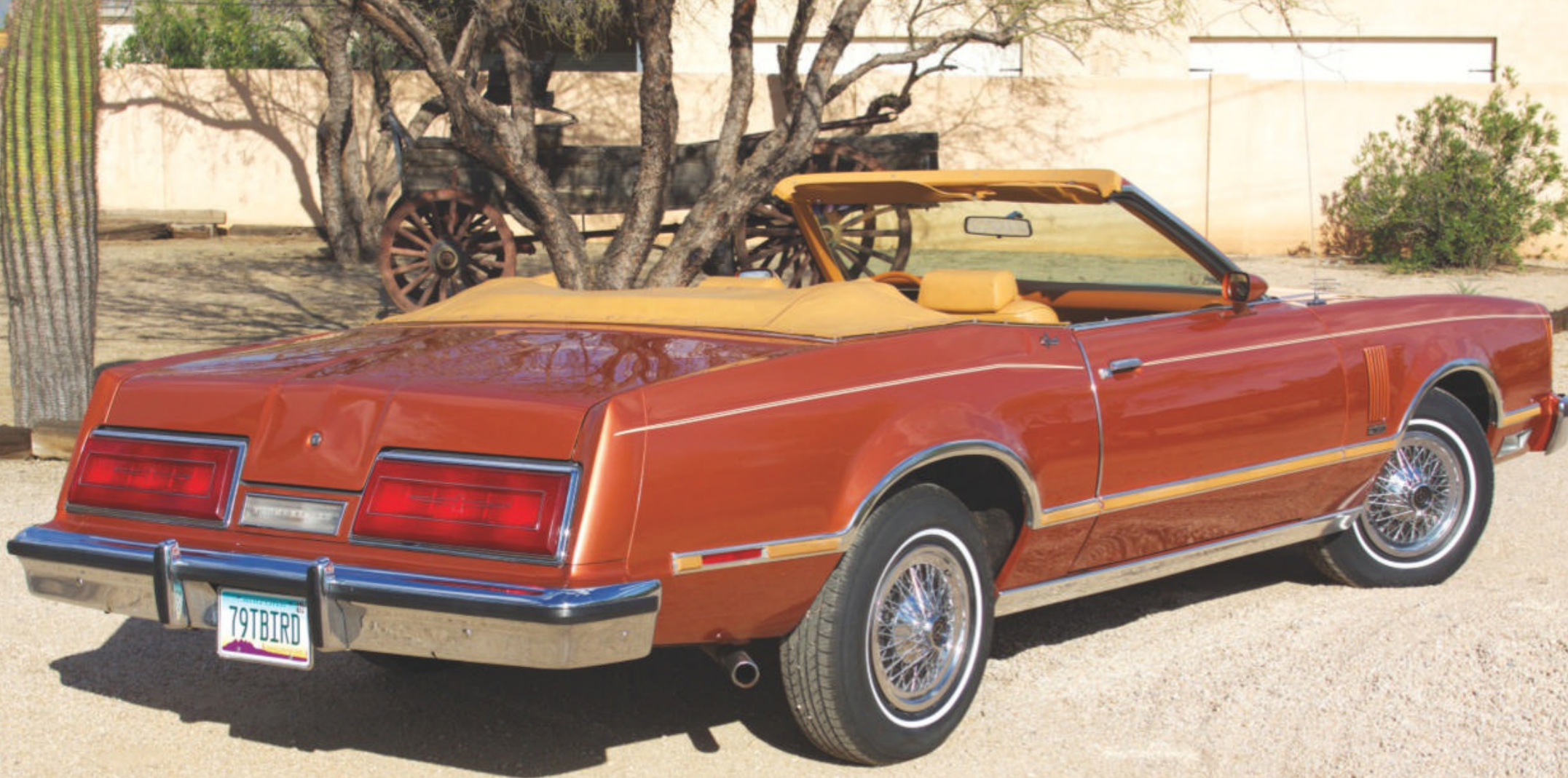
Above, the snap-in tonneau cover didn't sit quite flush but looked well finished; eliminating the roof amplifies the rear-quarter curves. Below, the erected soft top featured a velcro-clasp plastic rear window and a massive blind spot that didn't exist on coupe versions.
