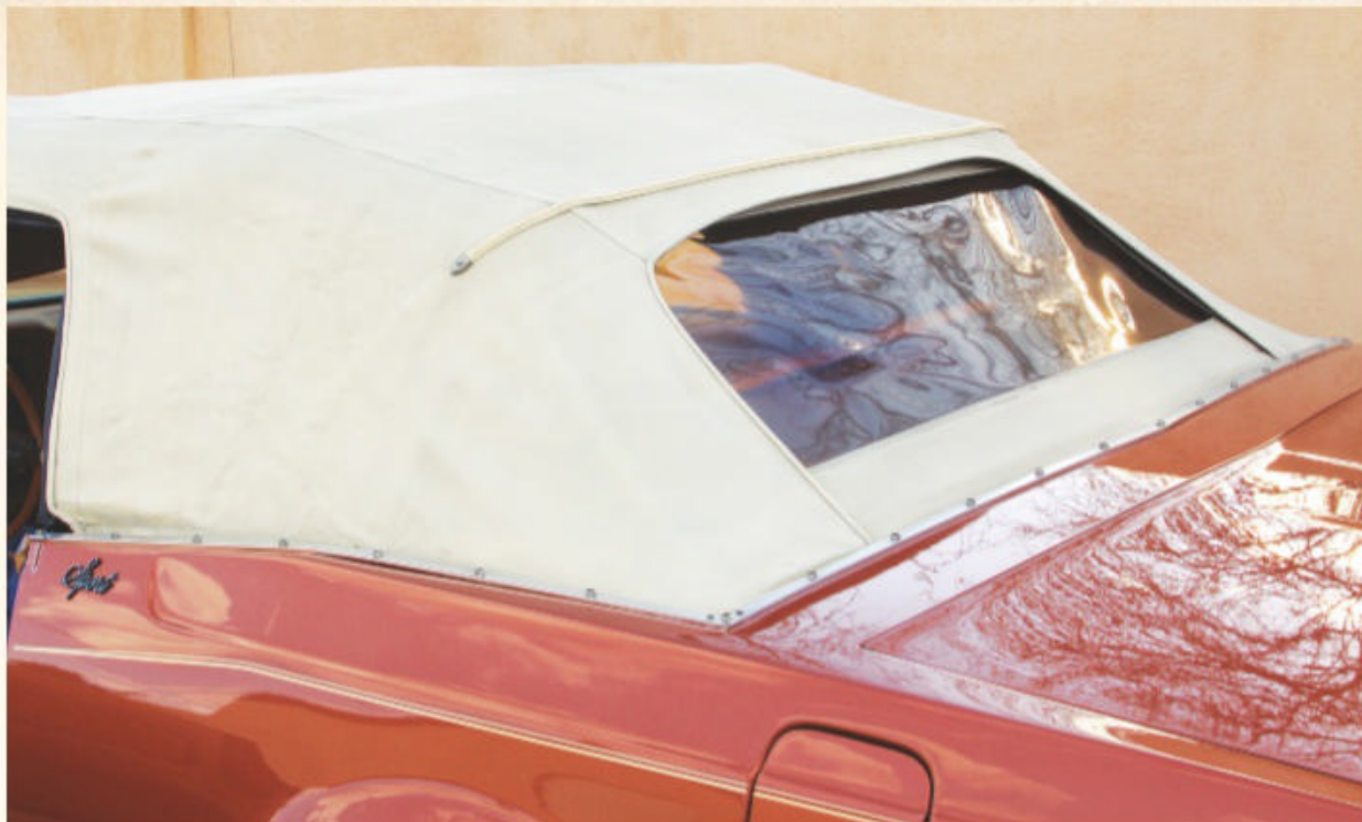
Above, the snap-in tonneau cover didn't sit quite flush but looked well finished; eliminating the roof amplifies the rear-quarter curves. Below, the erected soft top featured a velcro-clasp plastic rear window and a massive blind spot that didn't exist on coupe versions.
