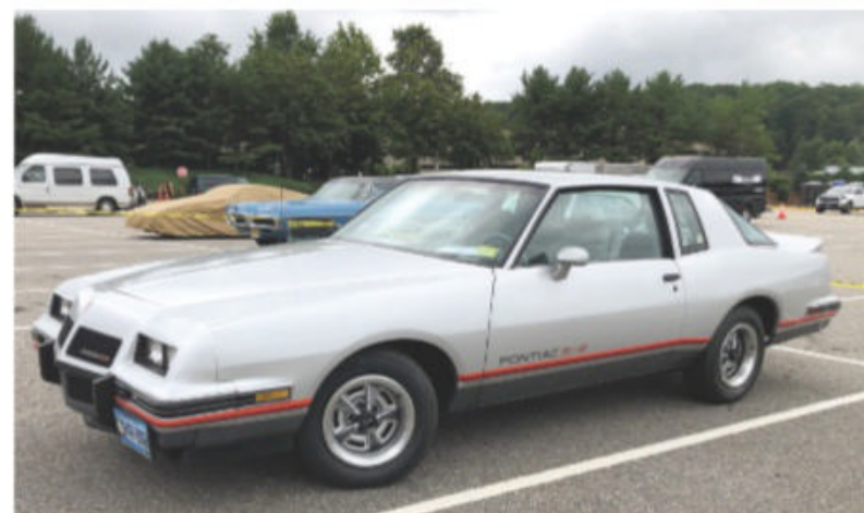
One never knows what will appear at a POCI gathering. Take, for instance, this 1986 Grand Prix 2+2, offered for sale by Mike Hust of Connecticut. The sleek nose and fastback rear window were part of the unique equipment designed in the wind tunnel—in cooperation with Richard Petty—to homologate the new aerodynamic profile for NASCAR competition. Just 1,225 were built, and three attended this year's convention.
