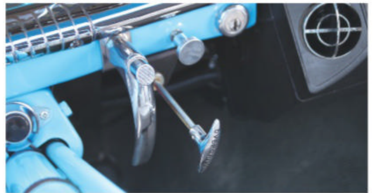
Gray leather replaces the factory broadcloth. Note lift-latch seatbelts. Despite air conditioning, the car does without a heater or a radio. Package shelf is modified for storage access. Pulling the handle marked “overdrive” locks the unit out of operation.
