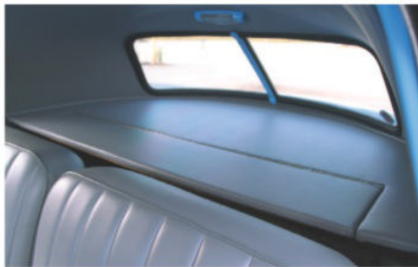
Gray leather replaces the factory broadcloth. Note lift-latch seatbelts. Despite air conditioning, the car does without a heater or a radio. Package shelf is modified for storage access. Pulling the handle marked “overdrive” locks the unit out of operation.
