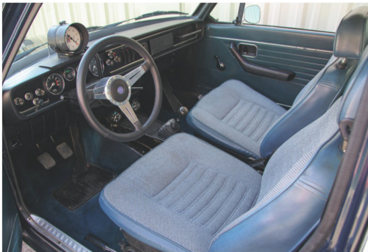
The Volvo's roomy cabin and comfortable seats easily accommodate the car's 6-foot-5 owner. The official Great Race Timewise 825 speedometer mounts atop the dash, its face twisted for quick viewing comprehension. Volvo's GT round-gauge cluster replaced the original strip speedometer, and a bank of accessory gauges monitor engine functions.
