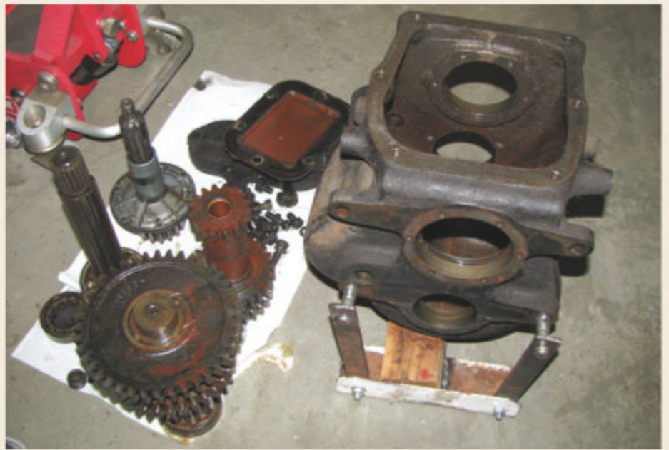
The original four-speed transmission was rusty inside from sitting with water in it, but rebuildable. Kent picked up a used four-speed and installed it to get the truck running, then eventually rebuilt this one.
