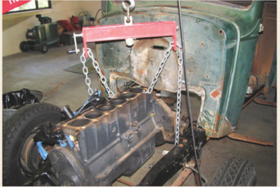
A compression test on the truck's 216-cu.in. six-cylinder revealed a dead cylinder, which turned out to be caused by a cracked cylinder head. Kent pulled the head and removed the engine for further inspection.
