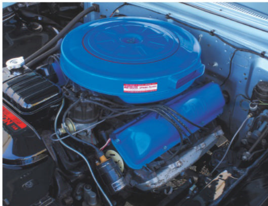
The original 220-hp 352-cu.in. V-8 did not require a major rebuild, even though it had over 213,000 miles on the clock before the restoration began.
