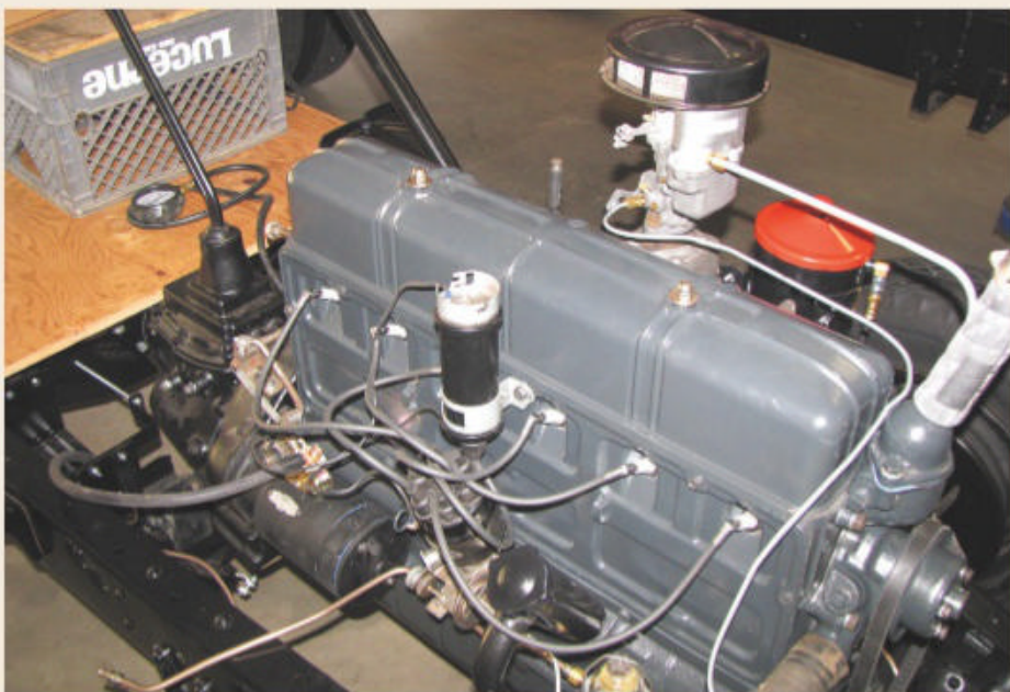
The 216, with fresh paint and a replacement head, fired up, ran great, and passed a vacuum test with flying colors. A stock Carter downdraft feeds the mix. An accessory oil filter is one of the few updates.
