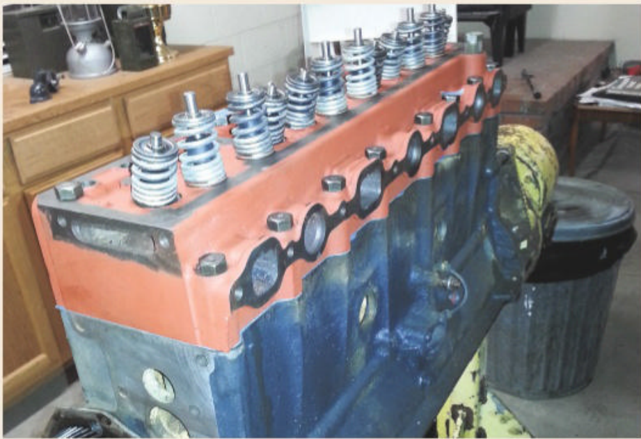
The truck's engine wasn't the original, but a 1940-vintage equivalent. Kent was able to track down a circa-1940 head that a friend reconditioned. It was then bolted to the short block, which turned out to be in good shape.
