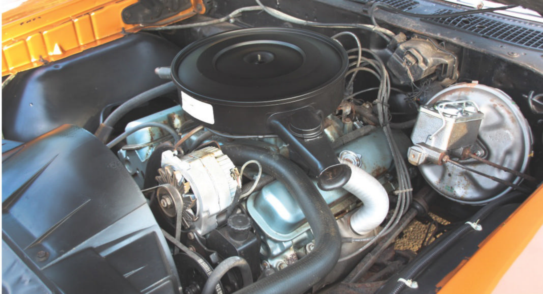
The Pontiac's original 160-hp, 350-cu.in. V-8 has been diligently maintained since new, helping it accumulate over 350,000 miles without a rebuild to date (above). Upholstery (left) is also original.
