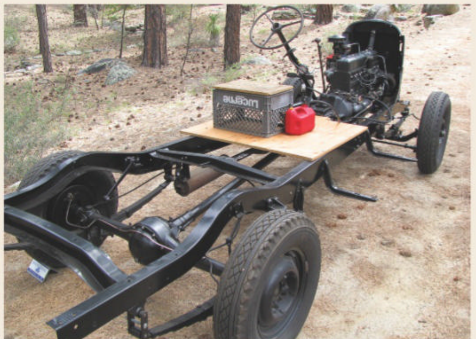
With the refinished chassis assembled and new Cunifer brake lines installed, Kent test drove the truck's running gear with a milk crate standing in for a seat and a small gas can providing the fuel.
