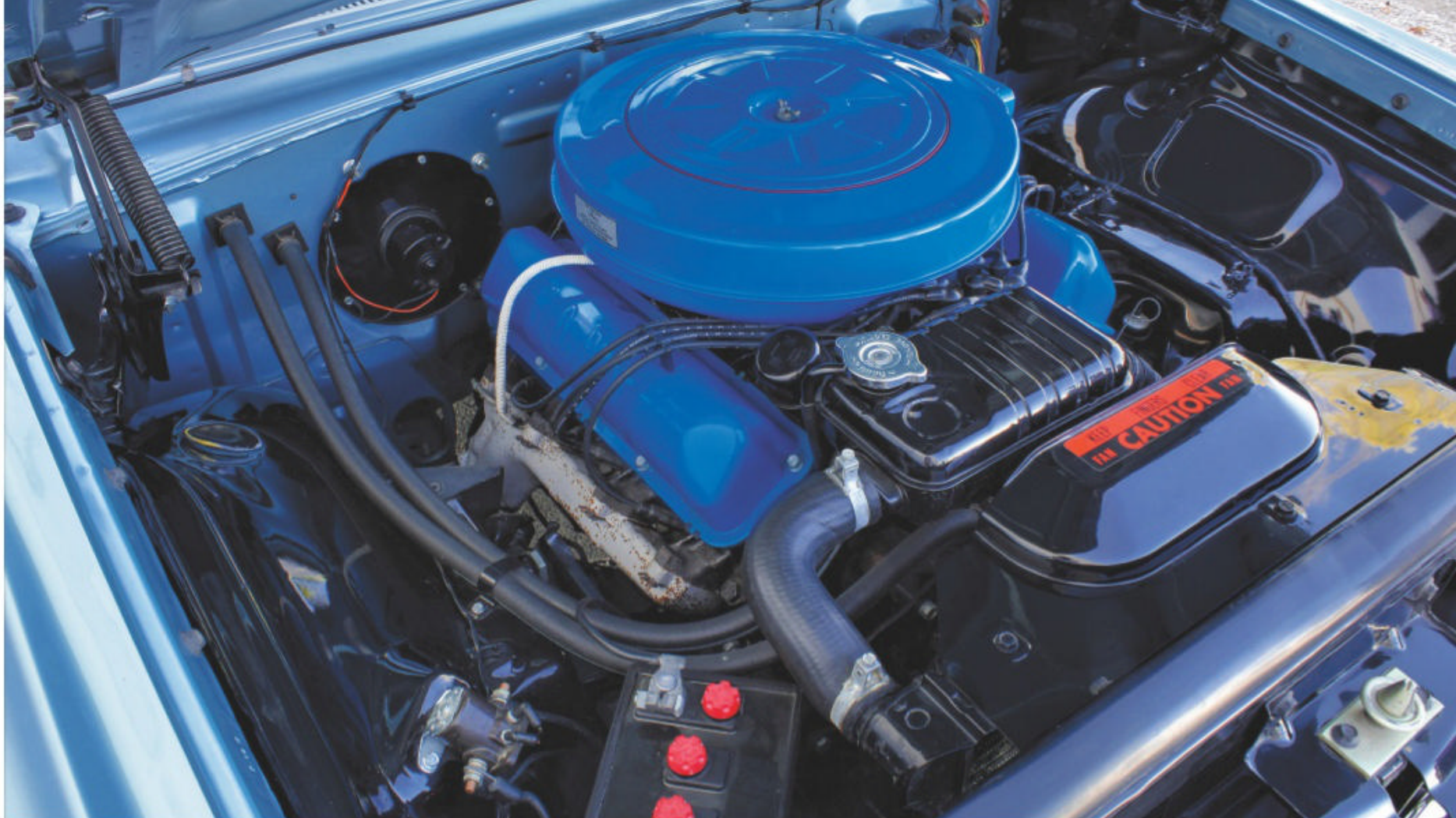
The original 220-hp 352-cu.in. V-8 did not require a major rebuild, even though it had over 213,000 miles on the clock before the restoration began.
