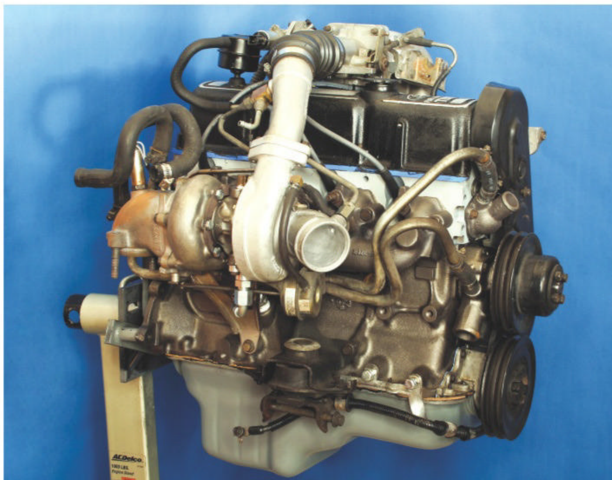
This page: Between 1983 and 1986, the fuel-injected 2.3-liter SOHC engine relied on an AiResearch T3 turbocharger. Next page: In 1987 and '88 it used an IHI turbo and a top-mounted intercooler.
