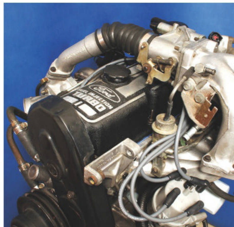
This page: Between 1983 and 1986, the fuel-injected 2.3-liter SOHC engine relied on an AiResearch T3 turbocharger. Next page: In 1987 and '88 it used an IHI turbo and a top-mounted intercooler.
