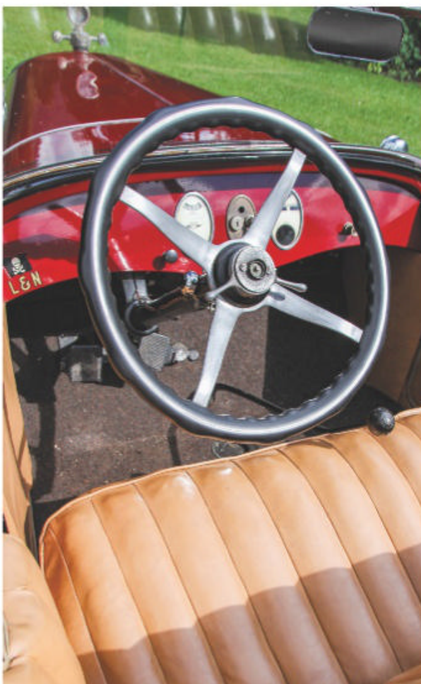
Instrument panel mounts an amps/fuel/oil-pressure gauge on the left, ignition and light switches at center and a speedometer/trip odometer/clock on the right. A few missing or replacement pieces, "L&N," and pirate flag are cryptic hints at the car's lost history.
