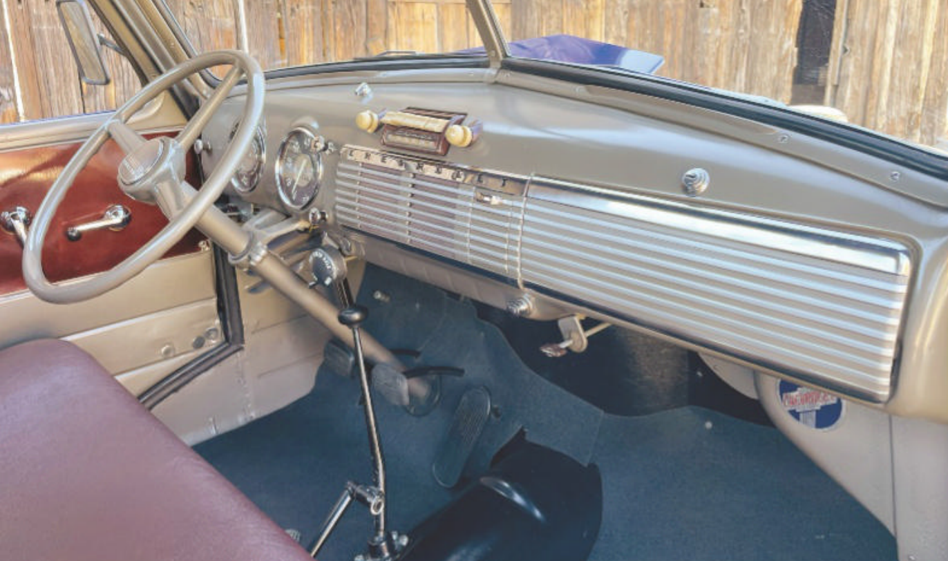
A commercial-grade cockpit, circa-1950, looks minimalist today, but this would've been considered well-appointed, sporting both a radio and a heater. The transmission is a four speed assisted by a two-speed rear axle, which is vacuum activated using the knob below the speedometer.
