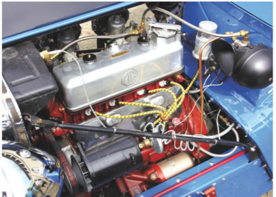
The 76-cu.in. XPAG OHV four-cylinder was introduced with the MG TB in 1939 and lasted through the earliest TF's in 1953. Jack based his engine on a TD block outfitted with TC external pieces.
