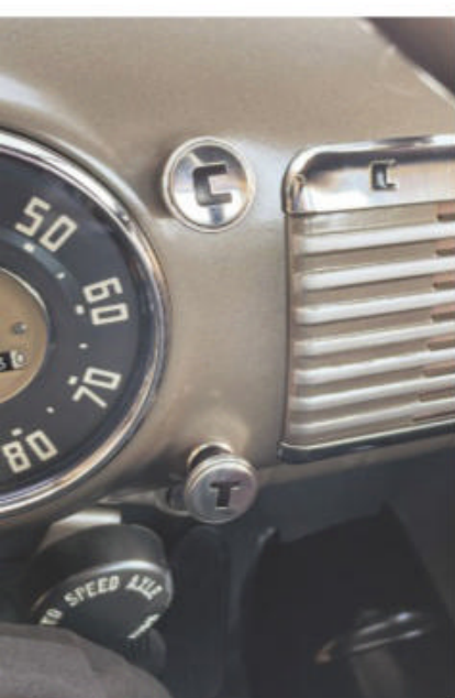
A commercial-grade cockpit, circa-1950, looks minimalist today, but this would've been considered well-appointed, sporting both a radio and a heater. The transmission is a four speed assisted by a two-speed rear axle, which is vacuum activated using the knob below the speedometer.
