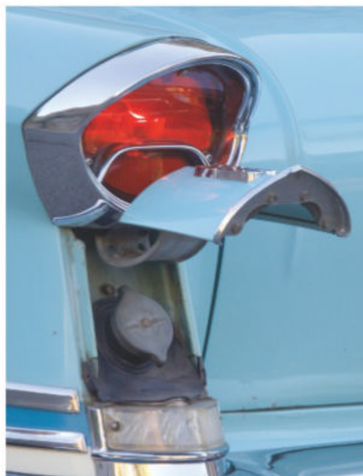
The fuel-filler cap is concealed behind a door that's part of the brightwork under the driver's side taillamp.
