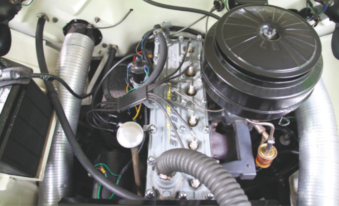
This car's 161-cu.in. straight-six was a set of points and a new muffler away from running well. Its Carter carburetor and ancillaries would be rebuilt.
