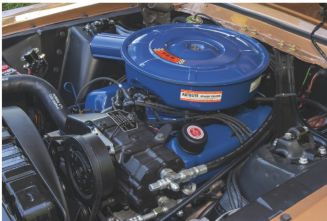
The 289-cu.in. engine was rebuilt to stock 200-hp, two-barrel specs, but an electronic ignition was added for reduced maintenance.
