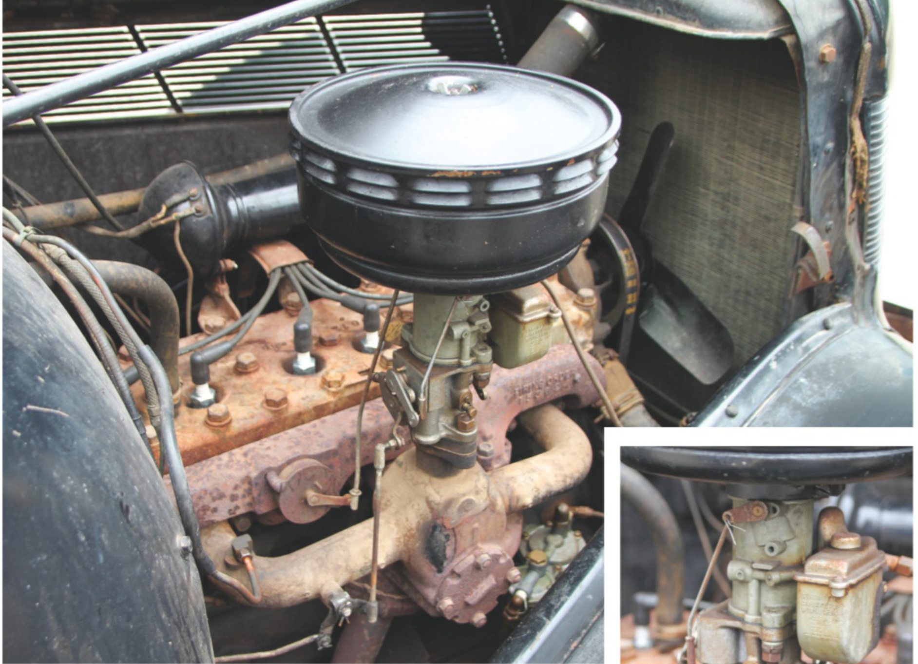
The Dictator's simple, robust, 205-cu.in., flathead, six-cylinder engine was rated at 88 horsepower making for a perfectly adequate power-to-weight ratio.
