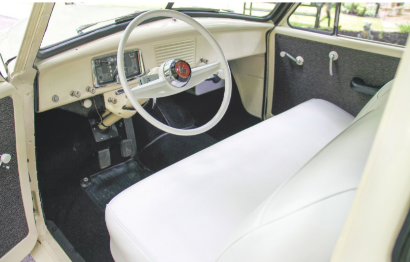
This Henry J's previous owner had reupholstered the seats, but John would have to replace interior side panels and headlining using proper automotive materials. He opted to fit carpet instead of rubber mats.
