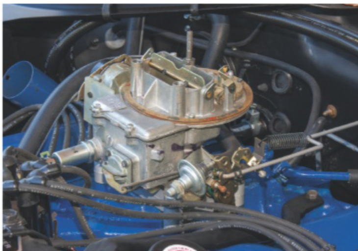
The 289-cu.in. engine was rebuilt to stock 200-hp, two-barrel specs, but an electronic ignition was added for reduced maintenance.
