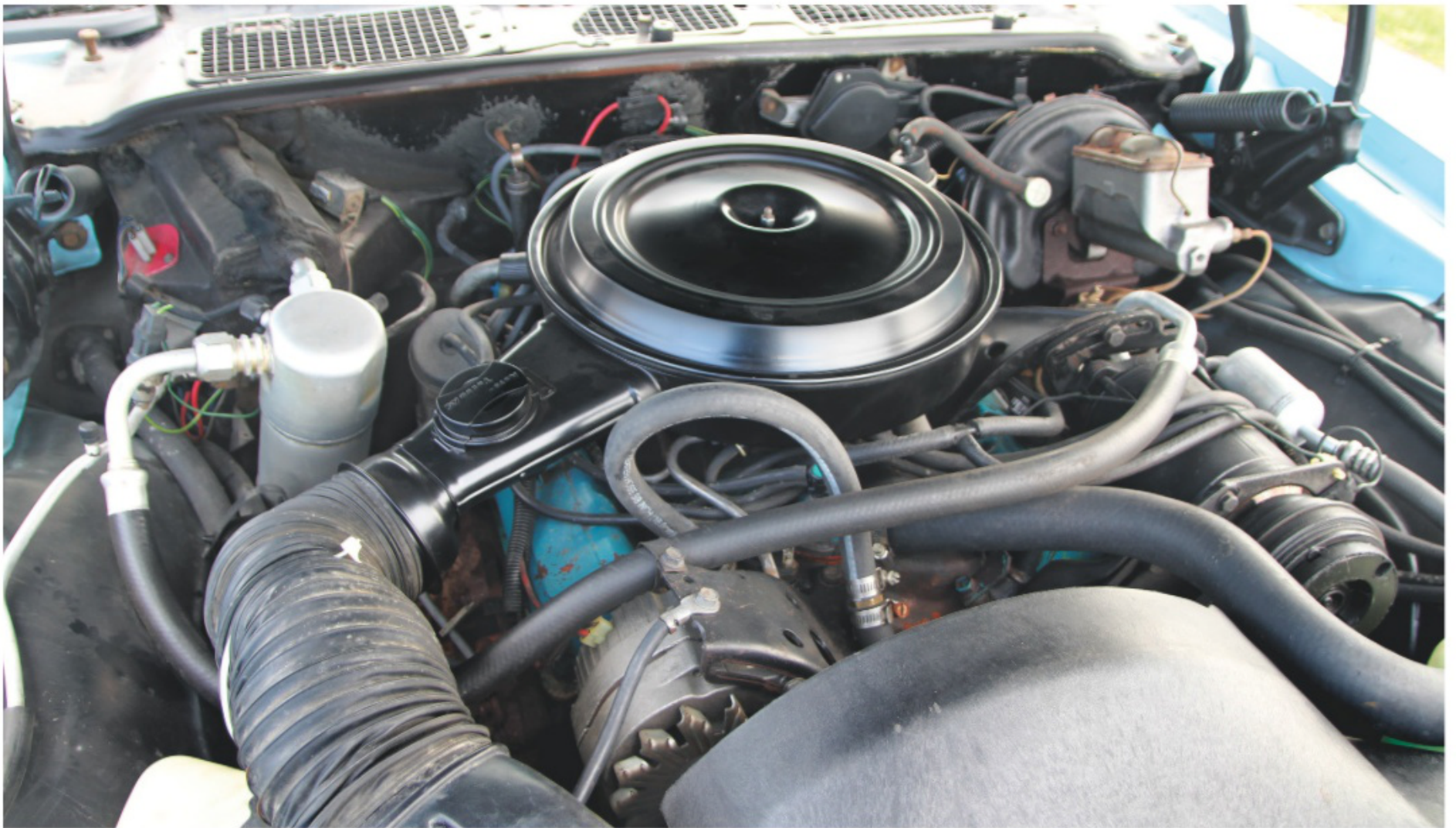
Pontiac's 1978 Firebird Sky Bird was offered with the divisions array of engine options; however, this one was delivered to its original owner with a 170-hp version of the 350-cu.in. V-8.
