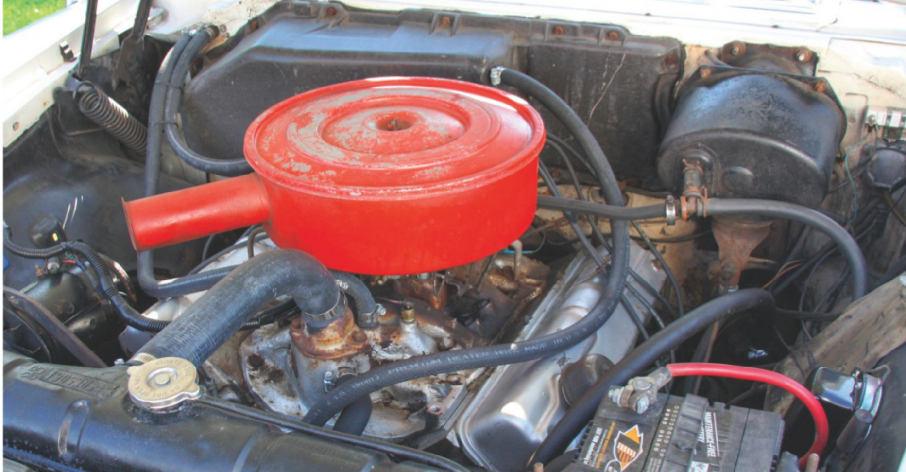
The base engine within the Fury series was the 230-hp version of the A-series “polysphere” V-8.
