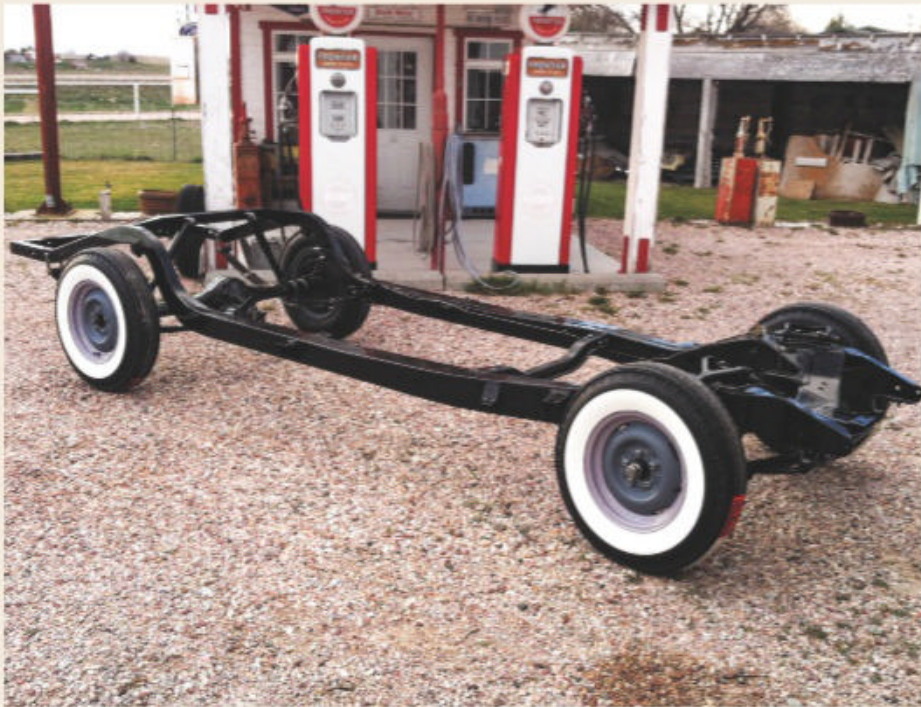
Scott stripped and painted the frame and rebuilt or replaced all the individual chassis components.
