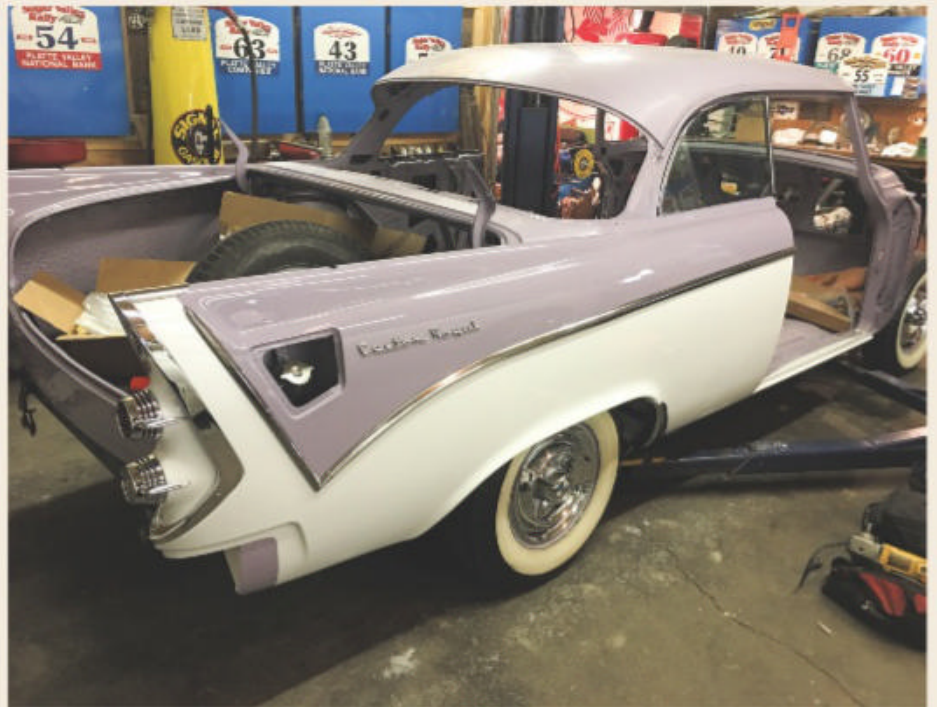
Final assembly is underway here with miscellaneous trim and quarter glass already installed.
