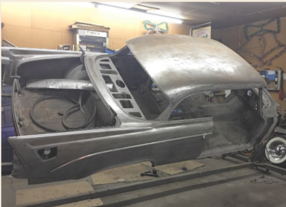
The body was stripped to bare metal and deemed to be in good condition overall with only minor rust repair required in the lower rocker panels.
