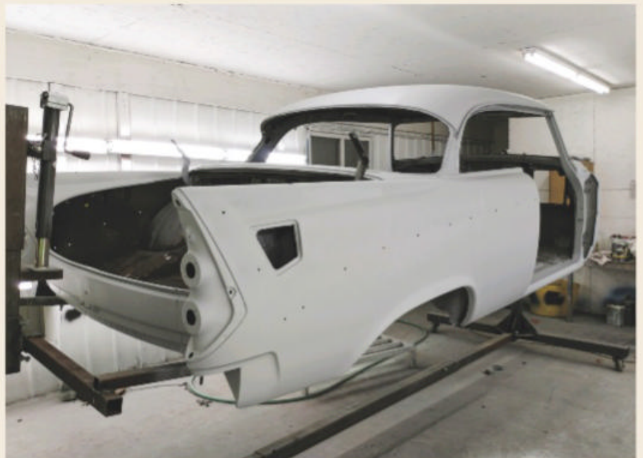
LeRoy Sanders of Sanders Auto Body in LaGrange, Wyoming, handled all the body and paint work. Once the sheetmetal repair was complete, it was sealed and an epoxy primer was sprayed.
