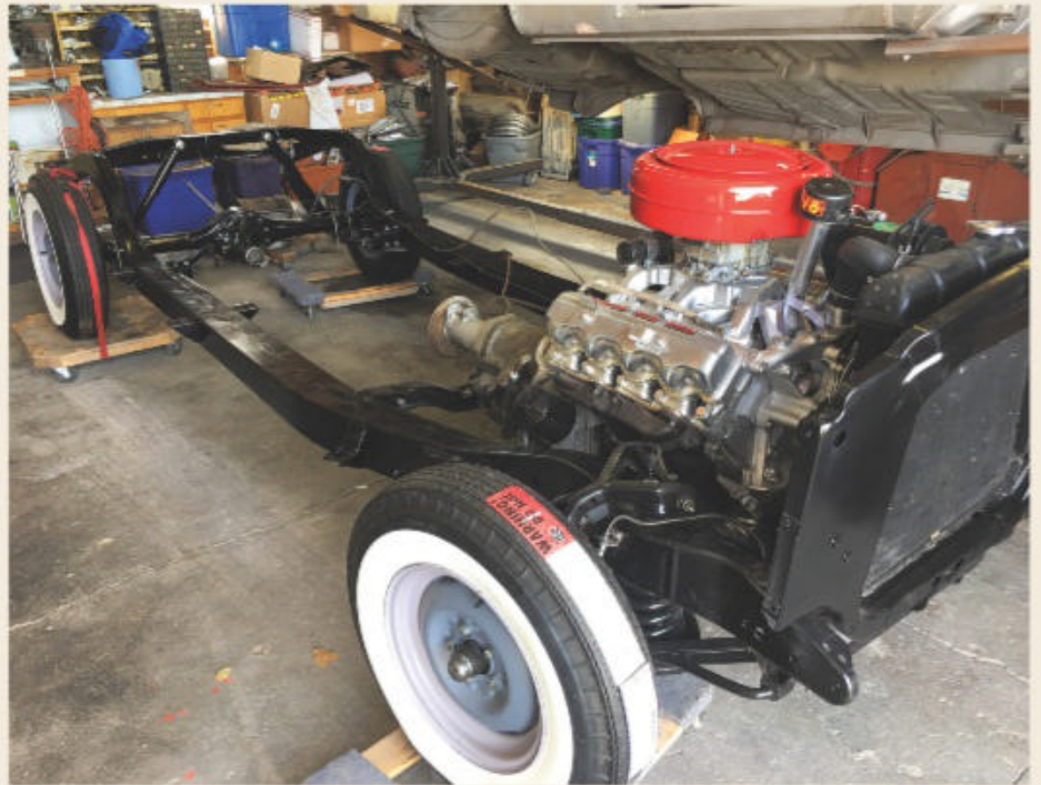
The completed drivetrain, including the rebuilt 315-cu.in. engine, was installed back in the chassis.
