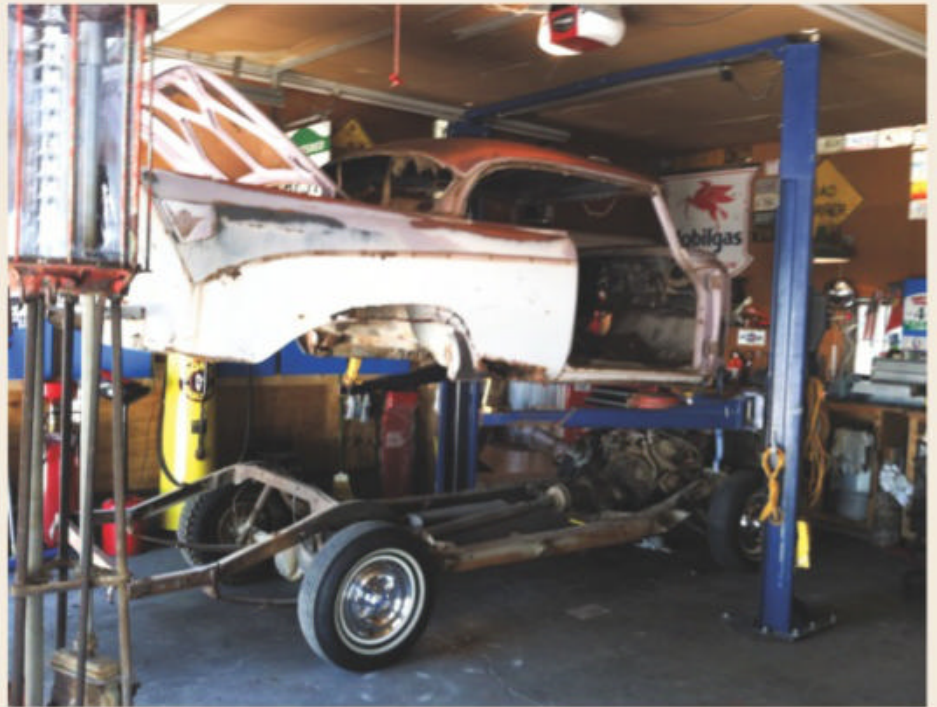
Disassembly started with separating the body from the chassis and sending out the engine for a rebuild.
