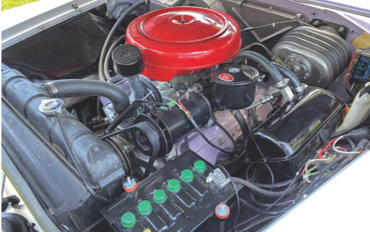
This La Femme is powered by Dodge's 230-hp, 315-cu.in. V-8 with a two-speed PowerFlite automatic. Scott took some liberty by painting the valve covers to match the body color.
