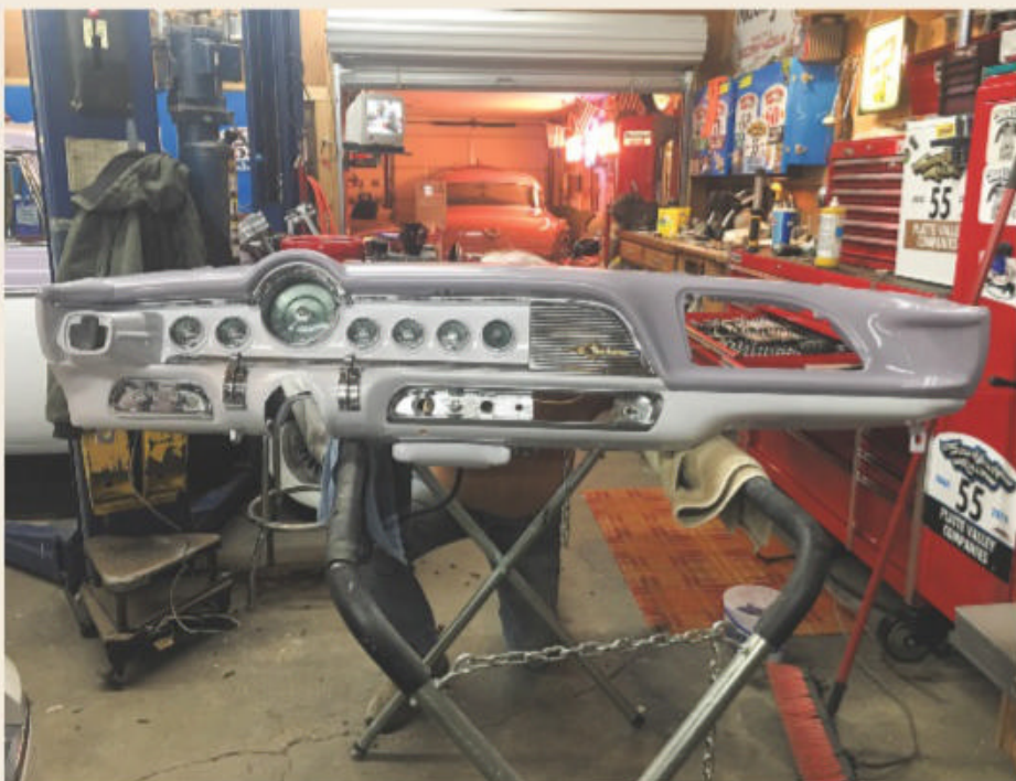
Scott spent many hours detailing and restoring the gauges, dash, and trim components.
