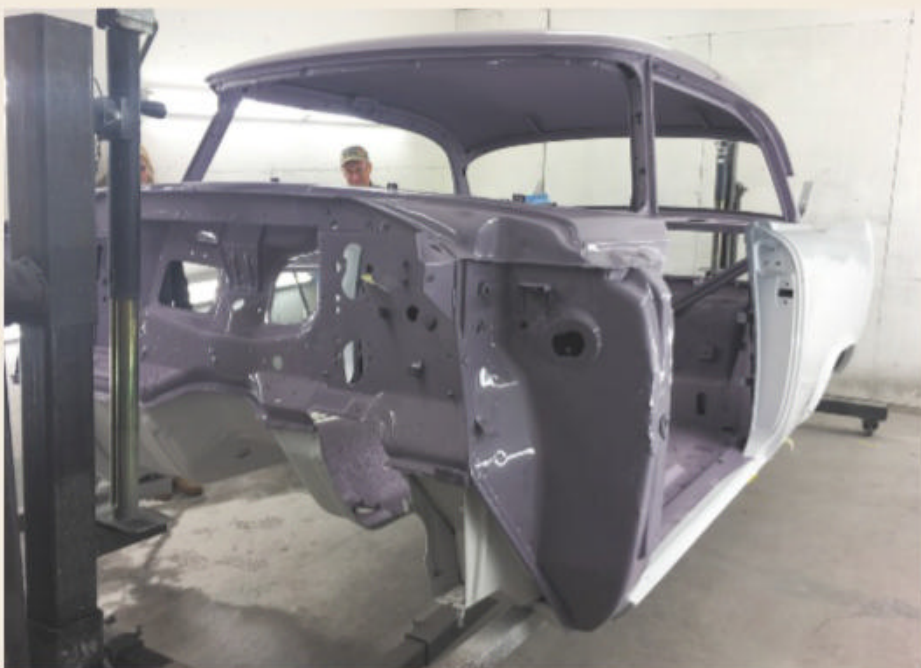
The body was then repainted in the factory two-tone Misty Orchid and Regal Orchid using a two-stage urethane paint system. It was then wet sanded and polished.
