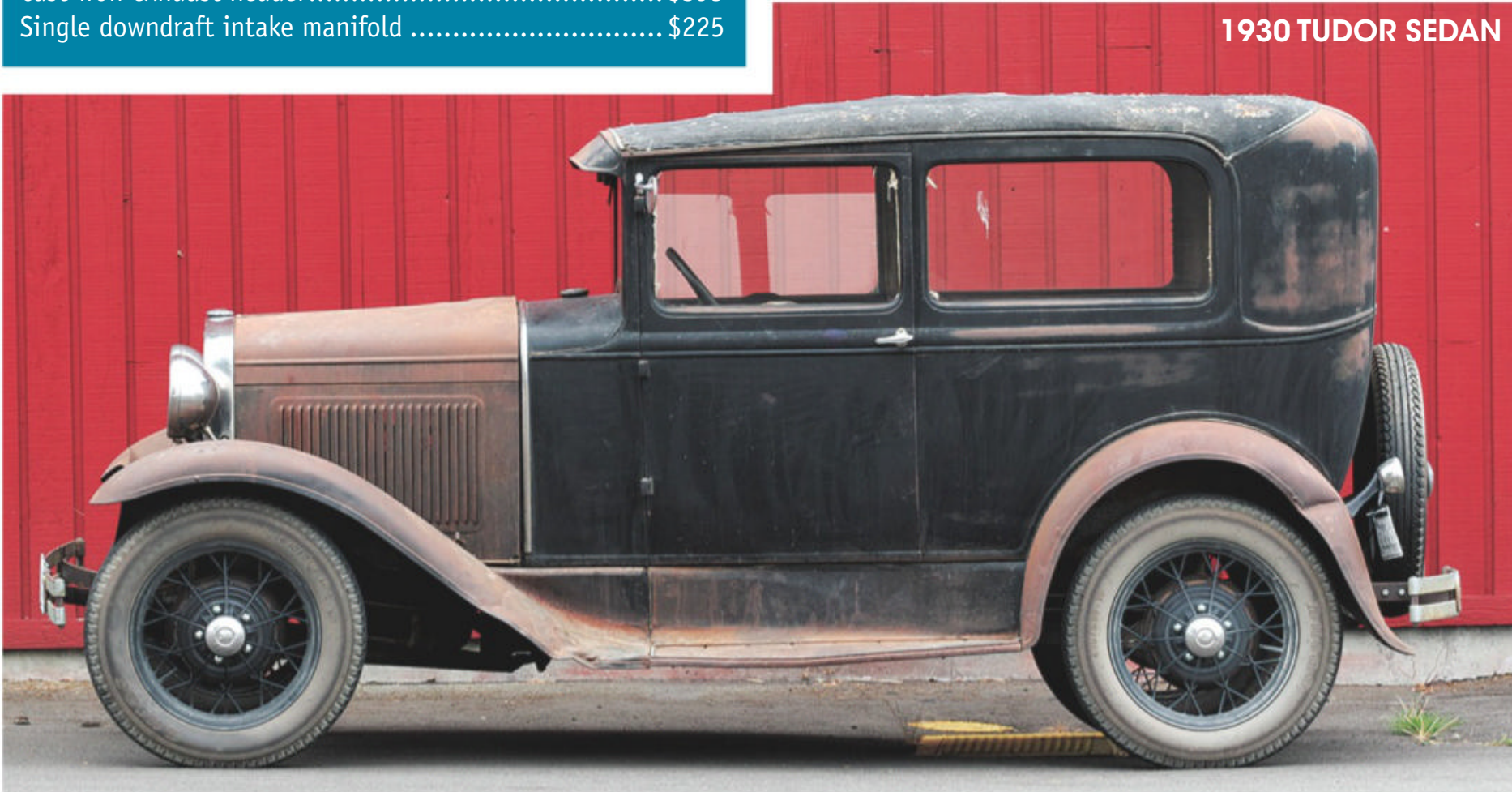
Changes after late 1928 were mostly cosmetic. The 1930 redesign, which debuted right about the time of the 1929 stock market crash, widened the cowl (granting more foot room) and updated the styling, but the engine and chassis remained essentially unchanged.
