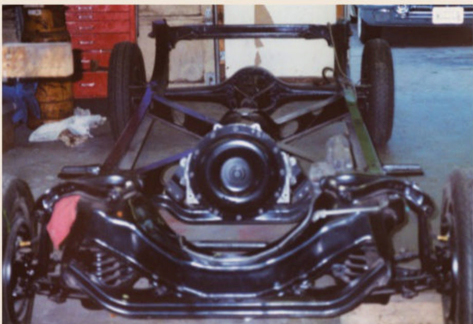
At this stage, the Pontiac's 122-inch wheelbase was painted chassis black and most of the new suspension components were reinstalled, including new brakes, stainless lines, and the Hydra-Matic transmission.
