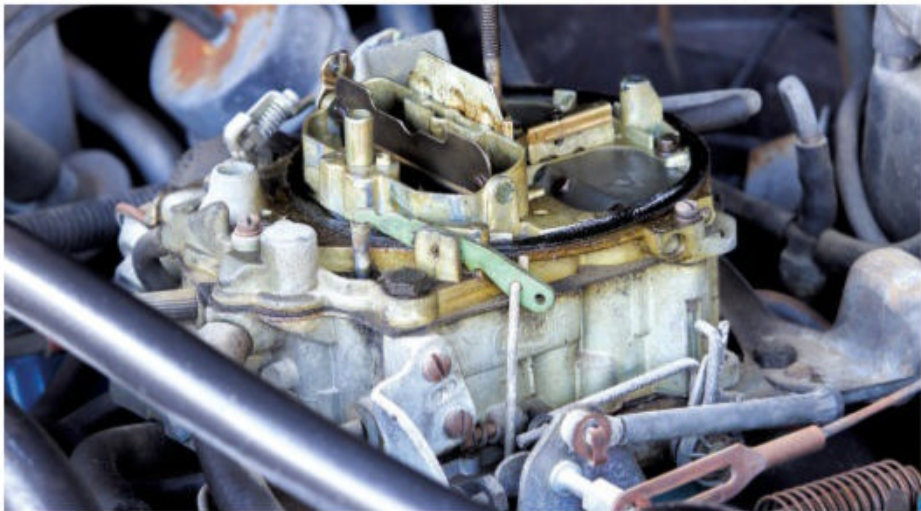
Trans Ams got Shaker scoops and 400 cubes, but the Firebird Esprit's top engine was this Canada-built 350-cube small-block Chevy; with the four-barrel carburetor on board, it was rated at 170 horsepower. Air conditioning was an option — and much loved after commuting 40 miles a day in a non-AC-equipped econobox in SoCal.
