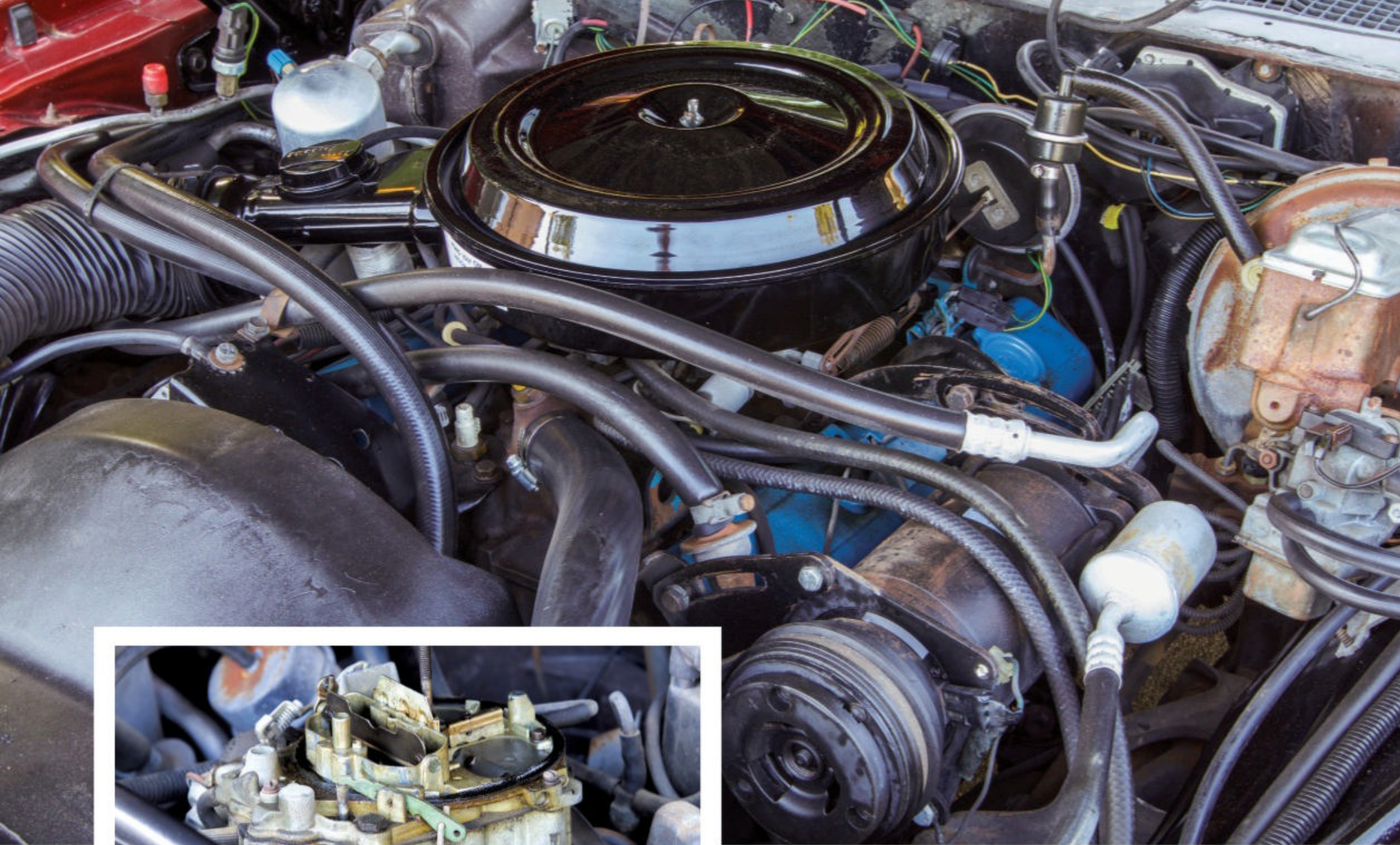
Trans Ams got Shaker scoops and 400 cubes, but the Firebird Esprit's top engine was this Canada-built 350-cube small-block Chevy; with the four-barrel carburetor on board, it was rated at 170 horsepower. Air conditioning was an option — and much loved after commuting 40 miles a day in a non-AC-equipped econobox in SoCal.
