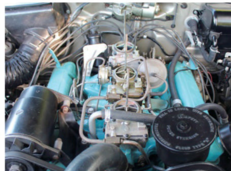
The original 347-cu.in. V-8 was rebuilt. The car was built with power steering, power brakes, and factory air-conditioning options.
