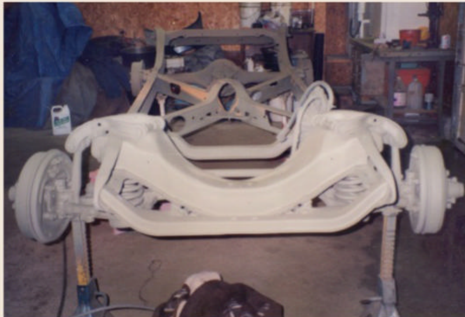
Wheeler II built a special sand-blasting booth within the family garage to media blast the frame to bare metal. As seen here, it's already received a coat of primer—to ward off flash corrosion—in advance of paint.
