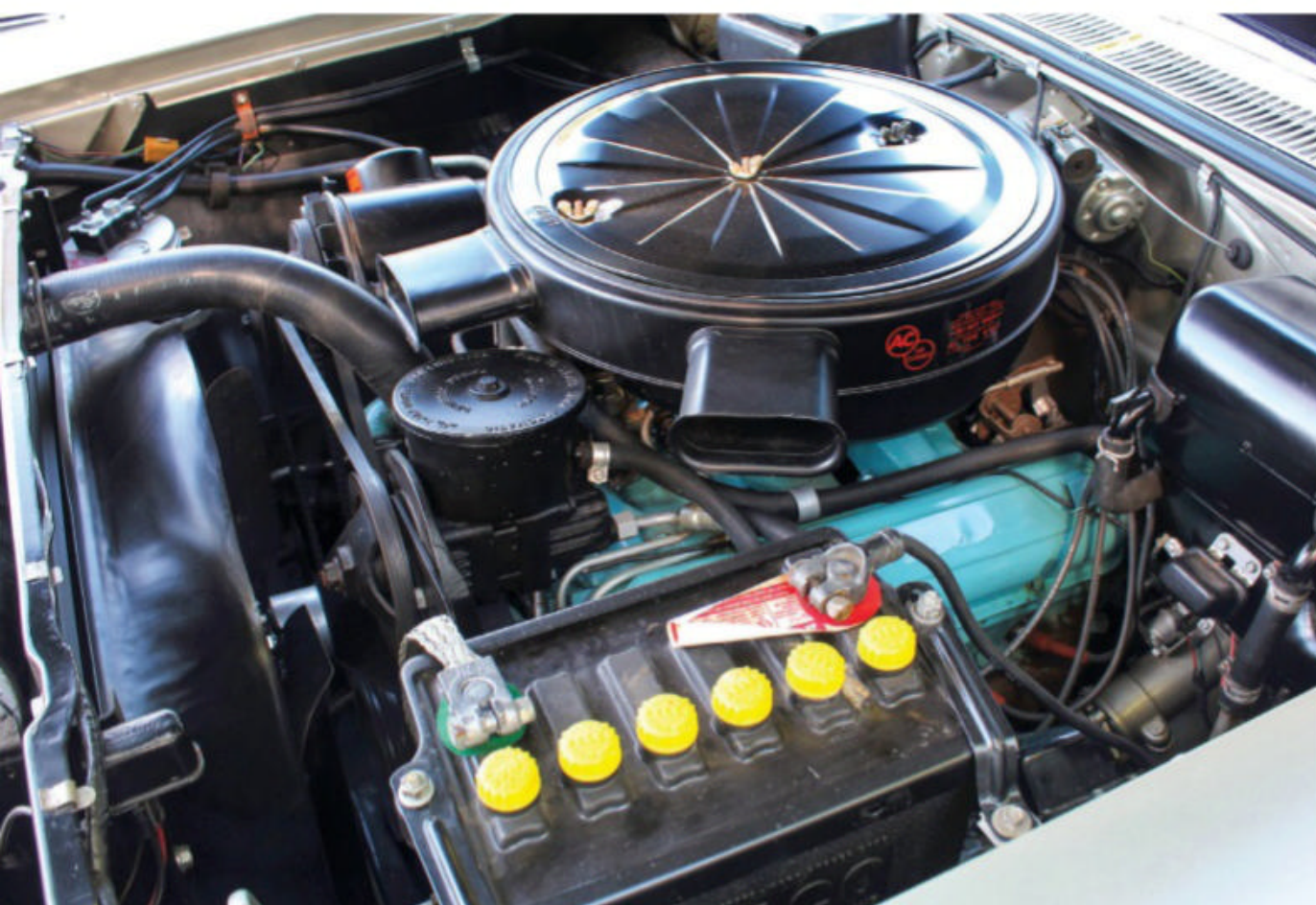
The original 347-cu.in. V-8 was rebuilt. The car was built with power steering, power brakes, and factory air-conditioning options.
