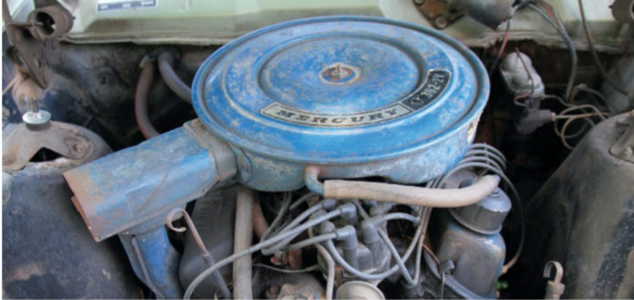
The Montego's 220-hp, 302-cu.in. engine was a venerable two-barrel economy V-8 that has managed all 65,140 miles showing on the odometer. Owner Brad reports he's yet to change the spark plugs.
