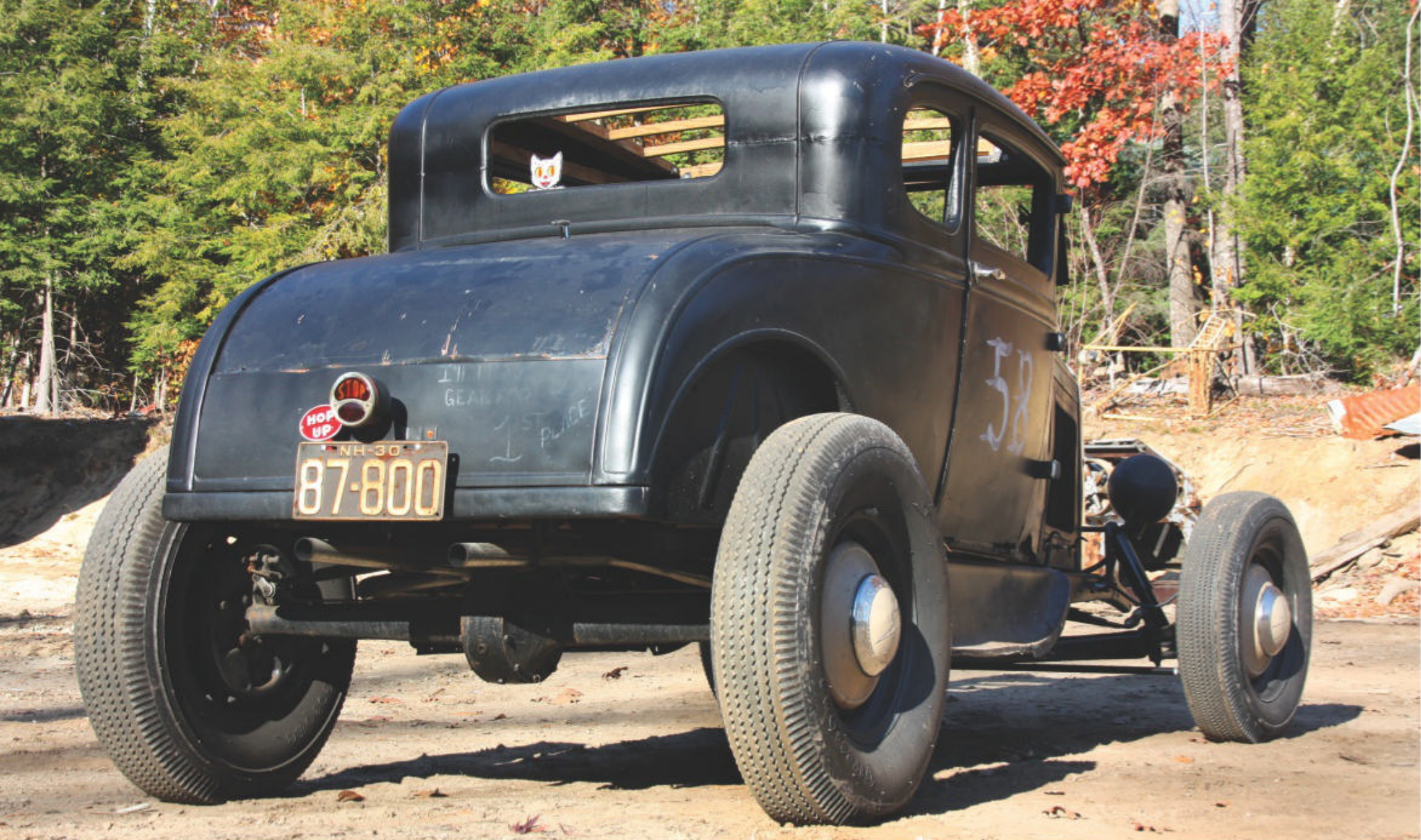
The cheeky comment about trading second gear for first place aside, early Ford components are robust when not hammered with 1960s levels of horsepower. Brian Lundgren's 1930 Ford Model A/V-8 coupe runs its flathead V-8 and 1939 Ford gearbox against an original, 4.11:1-geared Model A rear axle.
