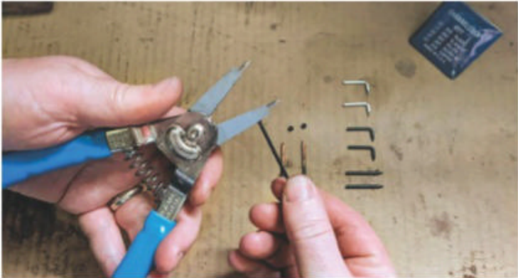
Swapping out tips is a simple matter of backing out the set screws and exchanging them for a different size or configuration included with the set.
