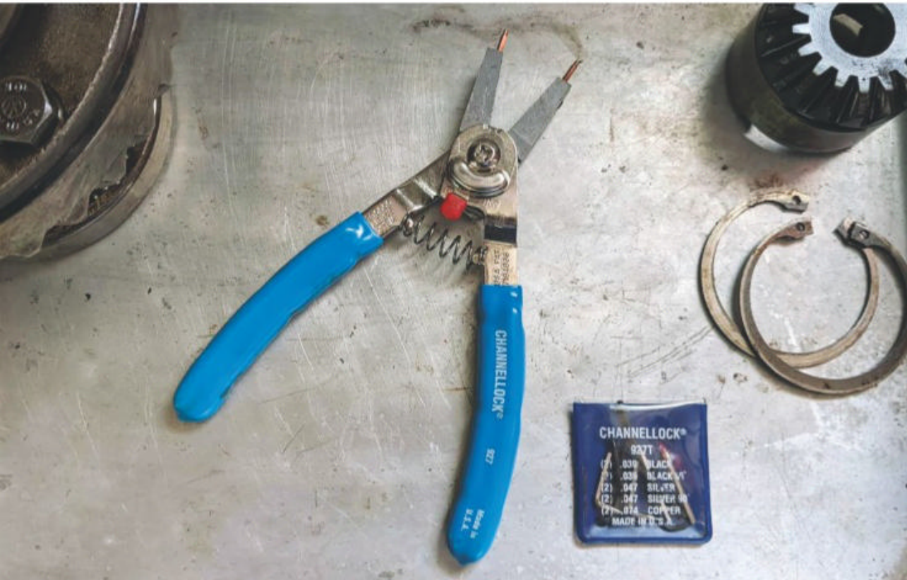
Swapping out tips is a simple matter of backing out the set screws and exchanging them for a different size or configuration included with the set.
