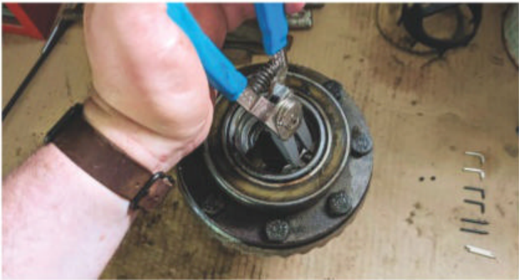
Although the Channellock pliers seem diminutive, they can easily manage big tasks. The heavy-duty snap rings in our Volkswagen differential were easy to remove and reinstall.
