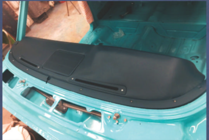
Tim sourced foam and grained vinyl and restored the dash pad himself. He stretched the foam and vinyl over the base and used Landau top contact adhesive to secure it. A heat gun and steamer were employed, as needed, to ensure that there were no wrinkles. He then vinyl dyed the pad to the proper color.
