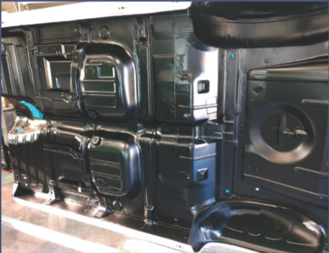
PPG high build epoxy primer followed by two coats Distinctive Image Hot Rod Black gives the floor pans a stock look, Tim notes. He also used Gravitex Plus Stone Chip Protector in the wheelwells for a factory undercoat appearance
