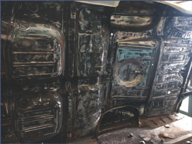
With the floors partially-stripped, their rust-free condition is revealed.
