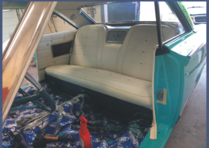
With the interior installation in process, we can see the Dynamat that was added to the floors to reduce noise transfer. The headliner, rear side panels, and recovered backseat now look factory fresh.
