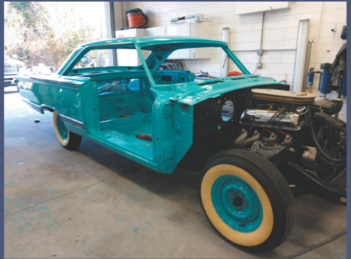
Reunited with the restored chassis with new body bushings and hardware in place, the Park Lane is beginning to look like a car again.
