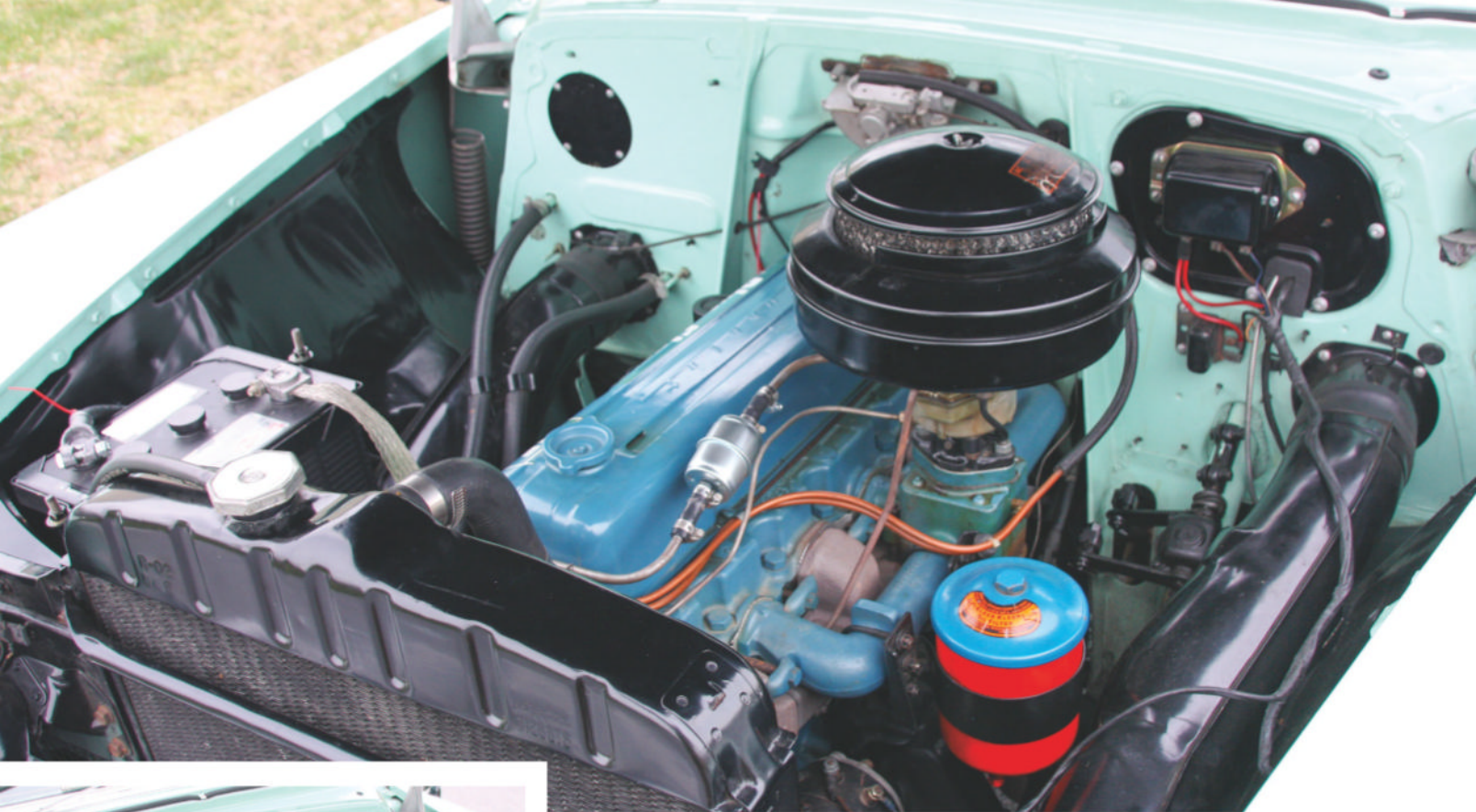
Cars with automatic transmissions got a 125-hp version of the 235-cu.in. straight six. Those who opted to stick with the base, three-speed manual got 115 hp.
