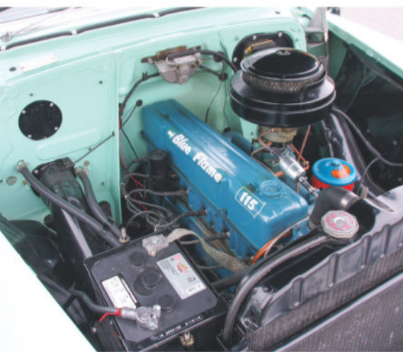
Cars with automatic transmissions got a 125-hp version of the 235-cu.in. straight six. Those who opted to stick with the base, three-speed manual got 115 hp.
