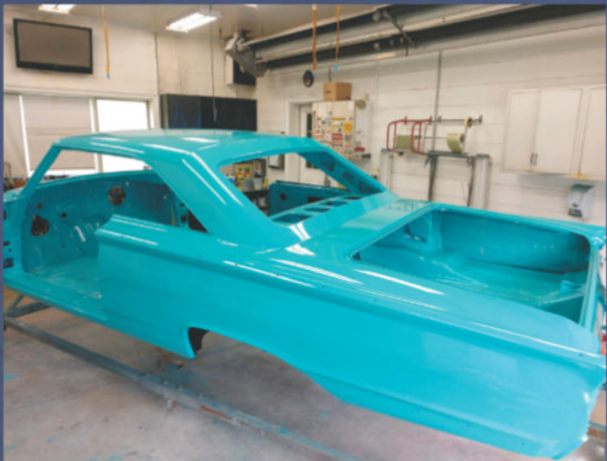
After three coats of color, four coats of clear, wet-sanding, buffing, and polishing, the shell is ready for reassembly.
