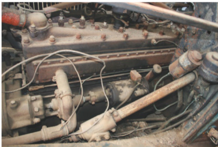
The original Lycoming engine was still wearing Ford carburetors and custom intake manifold created by the car's second owner.
