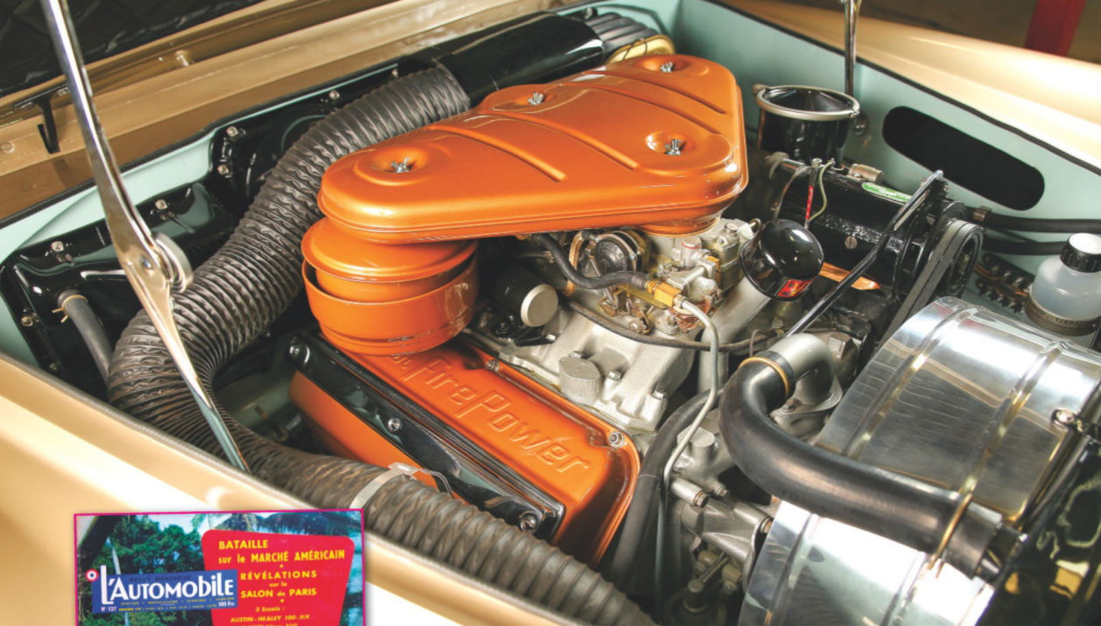
Under the hood is a powerful 340-hp, 354-cu.in. “FirePower” Hemi V-8 paired to a TorqueFlite automatic transmission.
