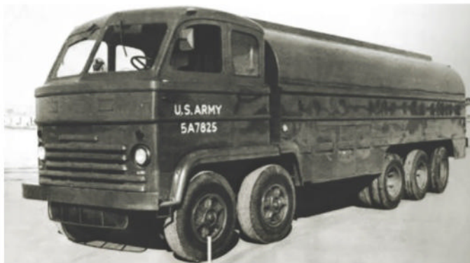
This illustration shows the four front-steering wheels, one of the features of the new twin engine truck developed by the Eisenhower Manufacturing Co., Van Wert, Ohio.
