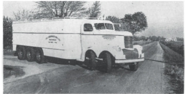
This illustration shows the four front-steering wheels, one of the features of the new twin engine truck developed by the Eisenhower Manufacturing Co., Van Wert, Ohio.
