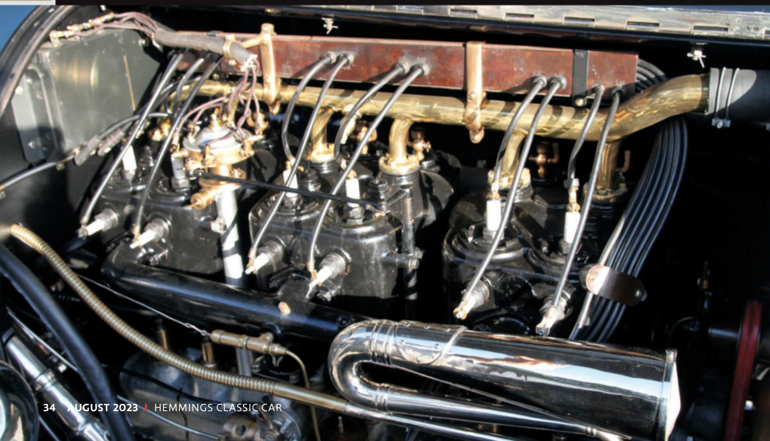
One of the interesting mechanical features of the Pierce-Arrow engine is its twin ignition system (below).
