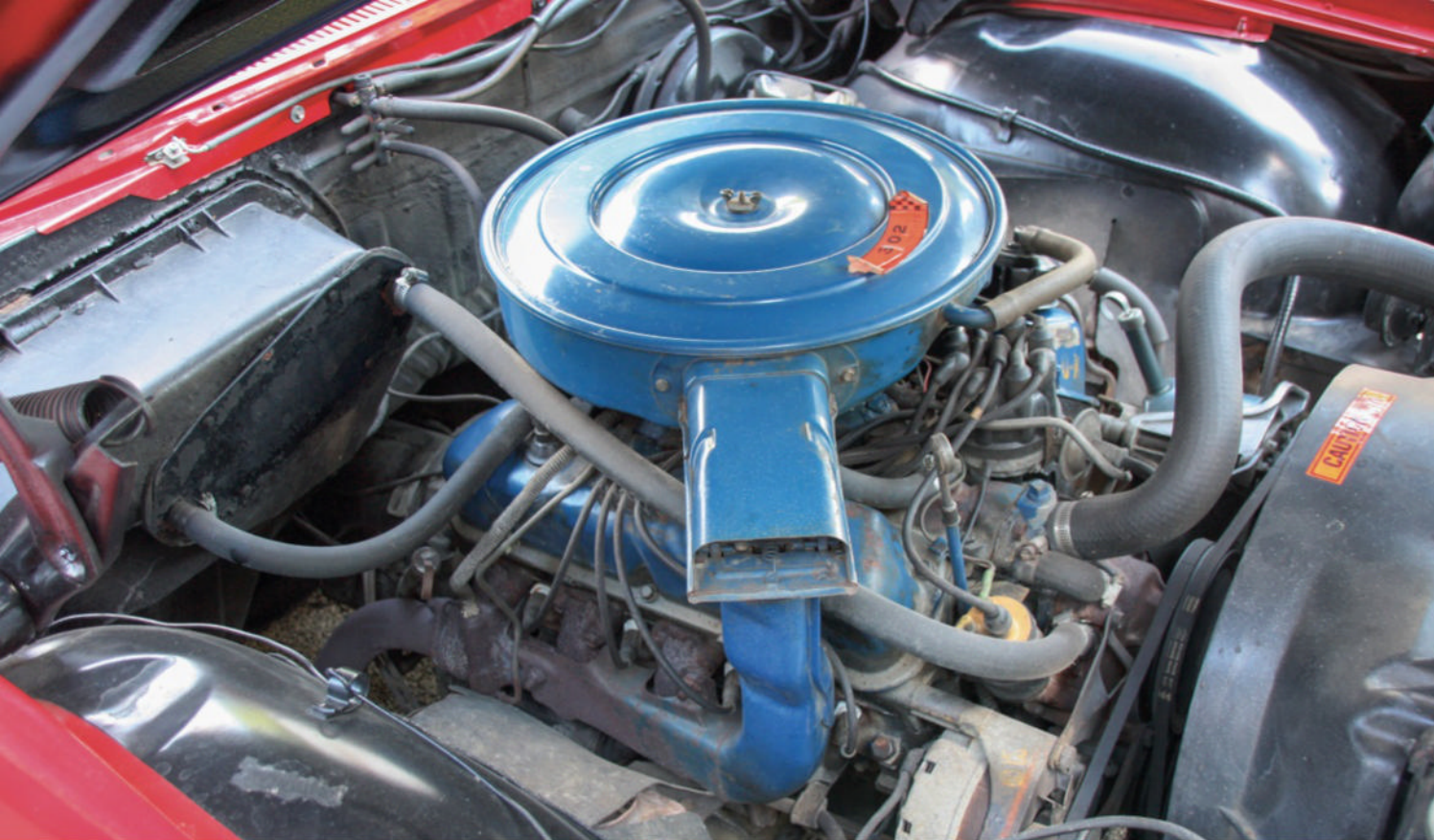
The Ford XL's standard V-8 engine for 1916 was the corporate two-barrel 302-cu.in. engine.
