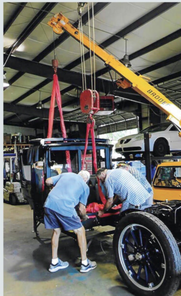
Brian's wife, Patricia, helped install the car's original six-cylinder engine (below, left) during the restoration. A friend's crane expedited the installation of the finished coachwork (right).
