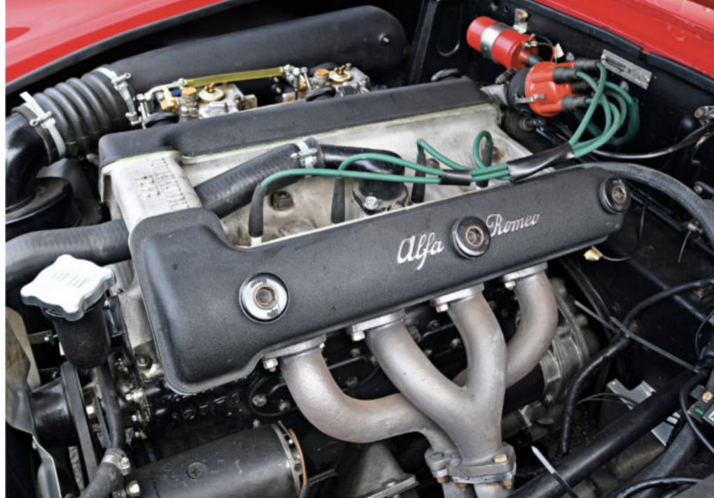
Jeff drives his Alfa Romeo with regularity throughout the summer months, so he swapped the original Solex carburetors for Webers. It's a somewhat common upgrade.
