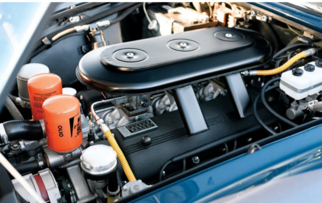
Ferrari’s 330 GTC was noted for its front-engine design and dynamic performance from its DOHC V-12.
