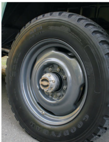
It took Mitch some searching to realize that Goodyear made a radial that looked at home on his vintage Budd wheels. These Goodyear G171s are 8R19.5 units.
