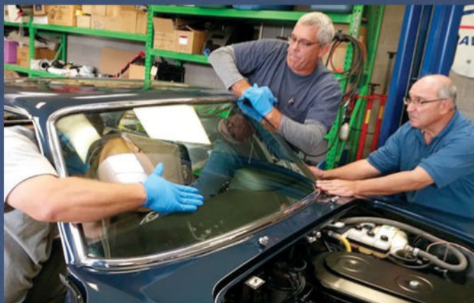
Novice enthusiasts may not be aware that Ferraris of this era were hand built with incredible precision, which means a "perfect-fit" windshield is exactly that. reinstalling one requires many hands and patience.
