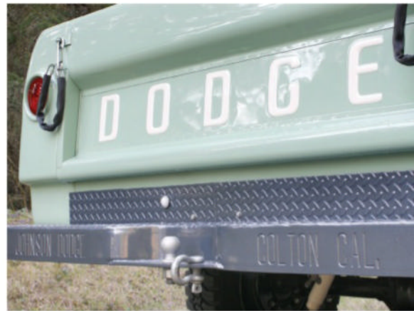
The original rear step bumper had some damage, and required considerable rebuilding plus powdercoating to end up looking as it does here. Considering it was emblazoned with the dealer name, it was worth the time and effort.
