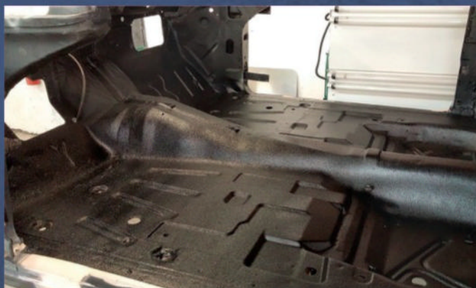
Once repairs were completed on the passenger front floorpan, the entire floor was coated with a spray-on bedliner product, followed by Dynamat.
