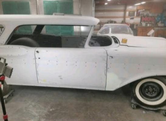
Close attention was paid to panel gaps throughout, certainly resulting in better alignment than the Mercury had when new.
