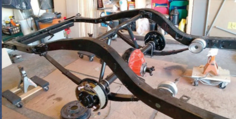
Other than the unique leaf spring bushings, refurbishing the rear axle and suspension was a typical restoration effort.
