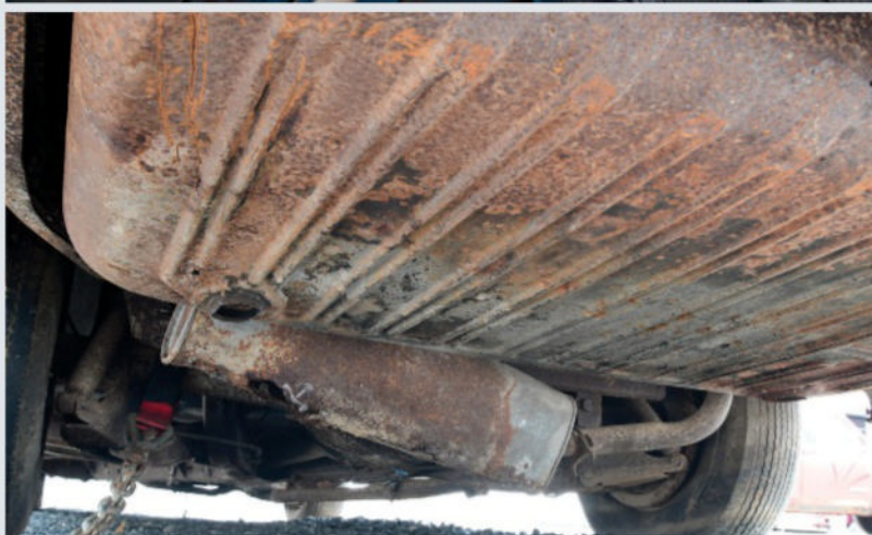
Rust had eaten away the bottom of the Buick's muffler, but not the fuel tank.
