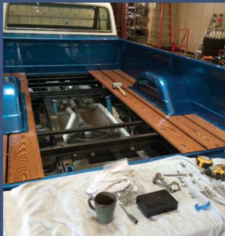
Plenty of priming and block sanding occurred to get the bed to look like this.
