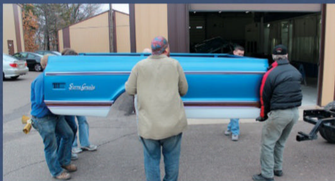
With the cab already reunited with the frame, the bed is lifted into place.
