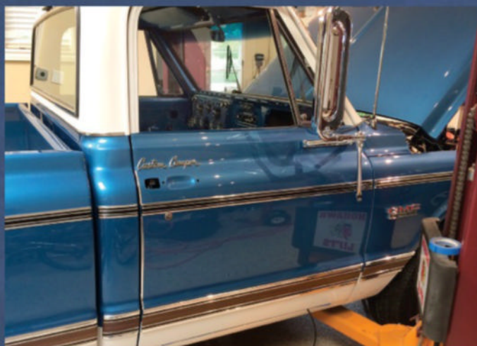
Dave has just reinstalled the factory mirrors after they were chromed. Compared to their earlier painted and tired condition, the difference is like night and day.
