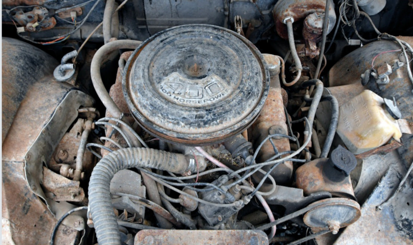
This LeSabre left the factory with a standard two-barrel equipped 300-cu.in. V-8 engine rated for 210 hp; however, someone swapped the air cleaner lid for that of a 1971 Chevy "Turbo Jet."
